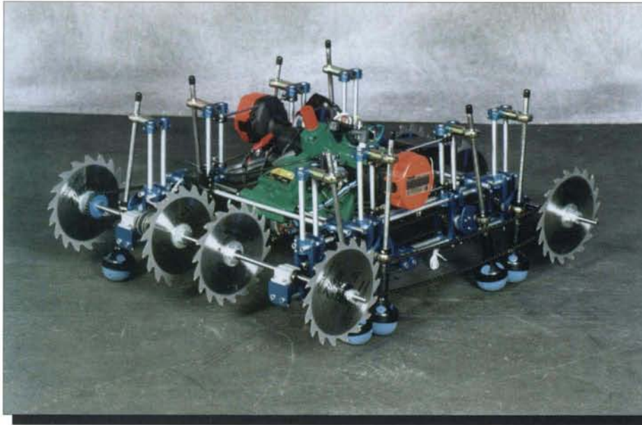
BuzzCut climbs atop opponents and rips them apart with gas weedeater-powered circular saws. Eight-legged RC walker by Christian Carlsberg of Walt Disney Imagineering. Photo by Dean Thomas Photography, L.A.
