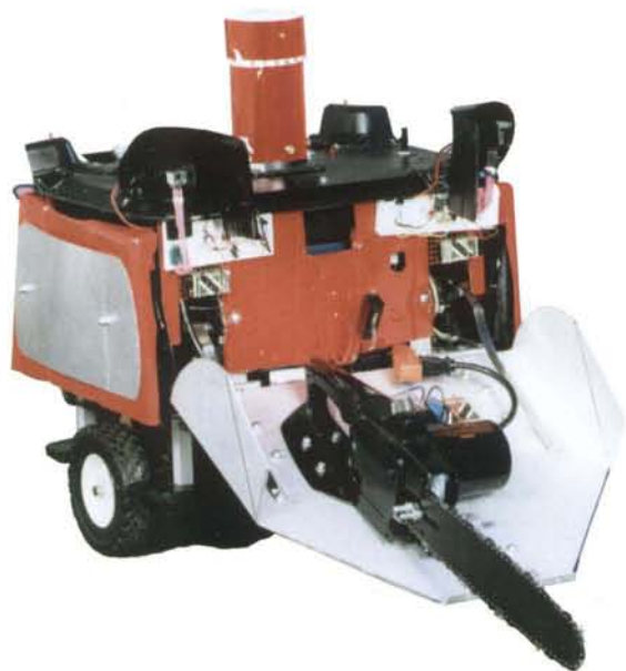
Gladiator II wields a pivoting electric chainsaw. Infrared target beacon on top. Laptop 386 under the hood. Fully autonomous attacker by Camp Peavy of Intuit. Photo by Dean Thomas Photography, L.A.
