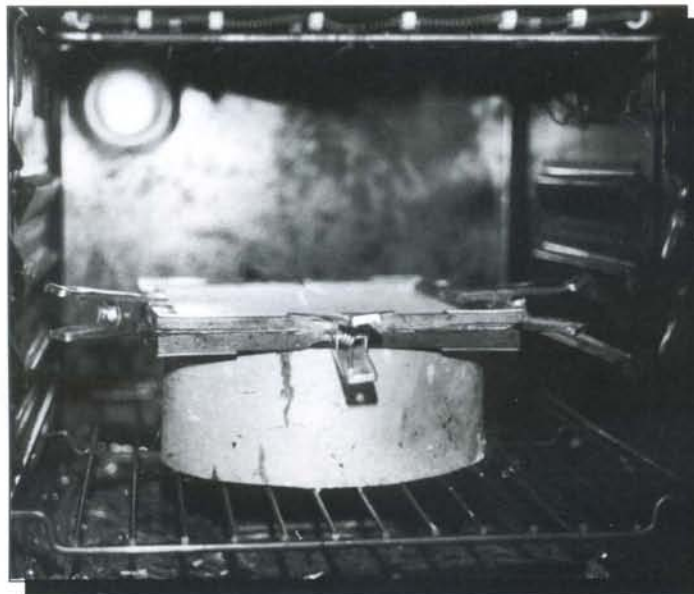
Photo 4: The plastic clamping frame in the oven. Note the metal standoff, which is supporting the frame.
