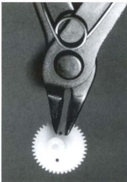
Step 5. Cut the travel-limiting spur completely off the gear.
