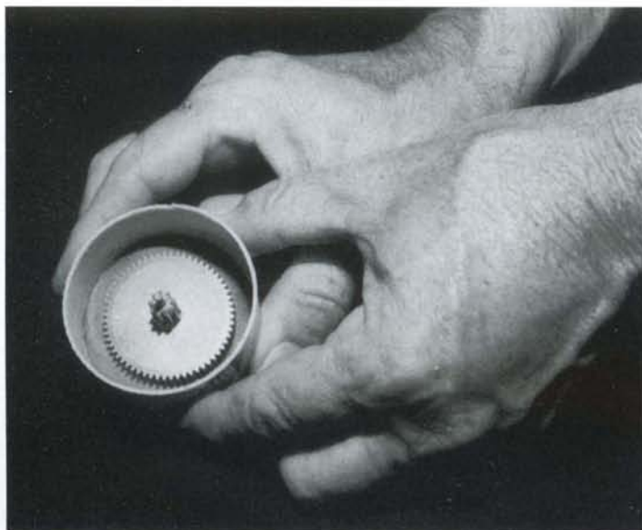
Step 2: Metal gear in place prior to pouring RTV rubber
