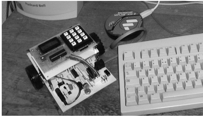
Figure 7.21: ICD 2 connected to a Derbot AGV
