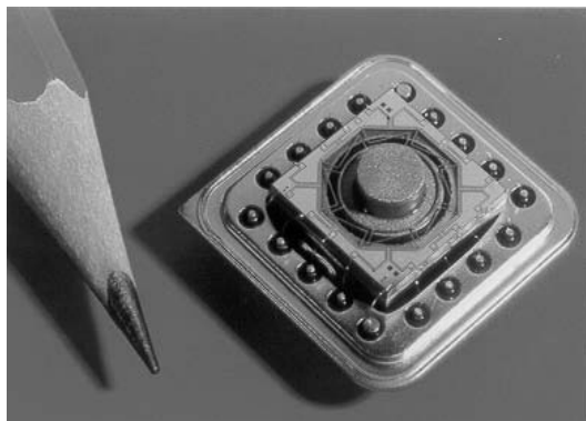
Figure 8.28 Commercial micromachined gyroscope from Silicon Sensing Systems. (From: [69]. © 1997 BAE Systems. Permission obtained from BAE Systems, who are a part of SSS.)
