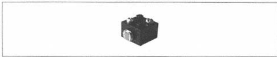
Figure 11-3. A CdS photoresistor mounted in a brick
