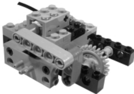
Figure 10.8 The Electric Valve with a Sensor
