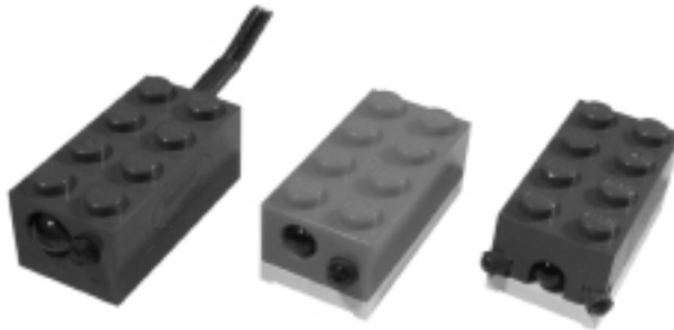
Figure 9.12 Different Kinds of Infrared Proximity Sensors
