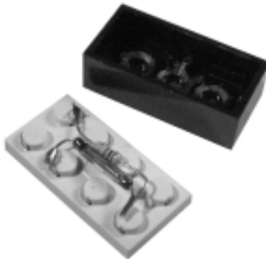
Figure 9.18 A Reed Switch Sensor before Final Assembly
