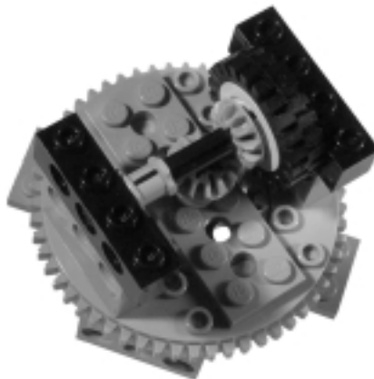
Figure 8.20 Incorrect Version of the Wheel Assembly
