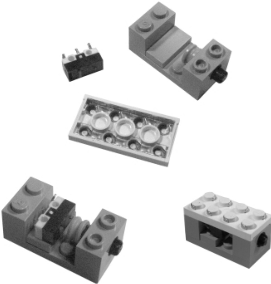
Figure 9.11 A Mouse Switch Recycled into a Touch Sensor
