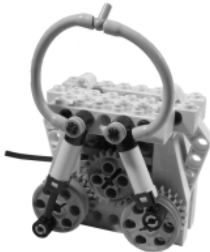
Figure 10.13 Ralph Hempel's Double Acting Compressor
