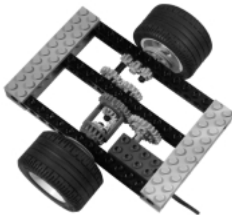
Figure 8.2 Monitoring the Difference in Right and Left Wheel Speed with a Single Rotation Sensor
