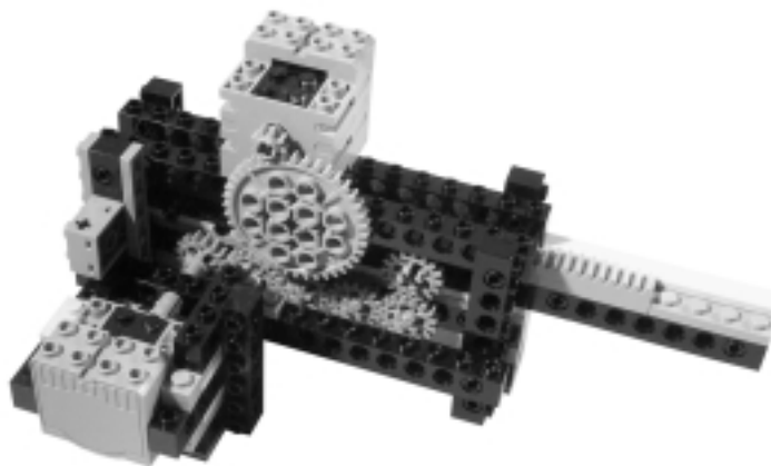
Figure 9.26 Switching a Motor among Five Output Axles
