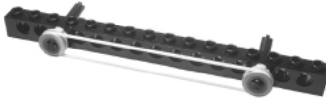
Figure 2.18 Pulleys Allow Transmission across Long Distances
