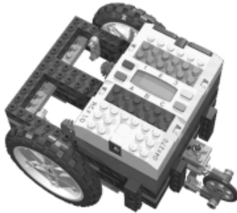
Figure 5.12 Better Positioning Improves Stability
