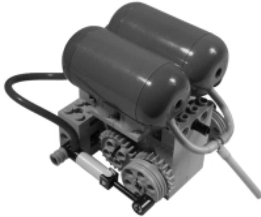
Figure 10.14 Another Double Acting Compressor
