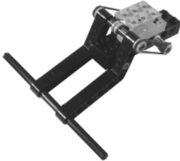
Figure 4.3 A Normally Closed Bumper
