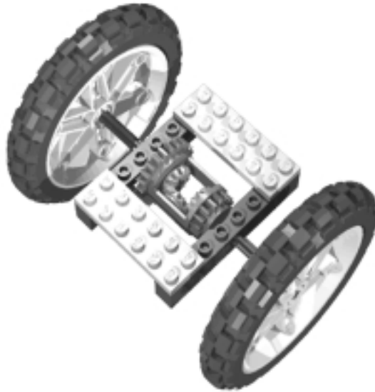
Figure 2.22 Connecting Wheels with the Differential Gear
