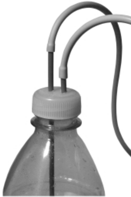
Figure 25.11 Detail of the Modified Cap
