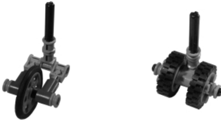
Figure 8.6 Casters Designed to Avoid Skidding
