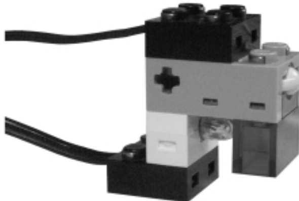
Figure 22.8 The Particulars of a Light-Button Unit
