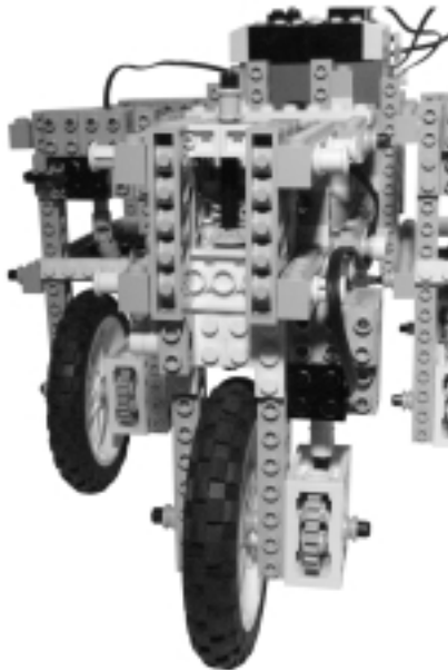
Figure 16.10 The SHRIMP Front Wheel
