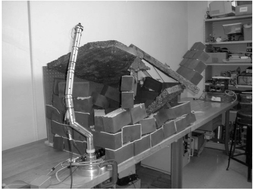
Figure 12.2 A snake robot exploring a search and rescue site. (Photograph courtesy of Howie Choset.)
