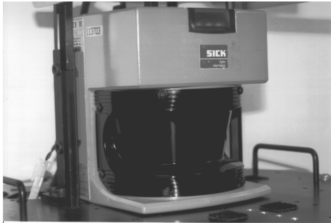
Figure 6.28 Sick laser, covering a 180° area.
