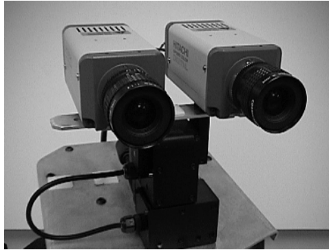
Figure 6.21 A stereo camera pair mounted on a pan/tilt head.
