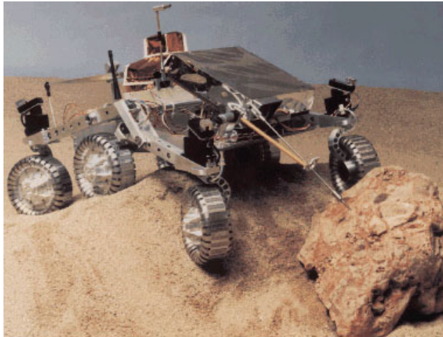
Figure 1.7 Sojourner Mars rover. (Photograph courtesy of the National Aeronautics and Space Administration.)
