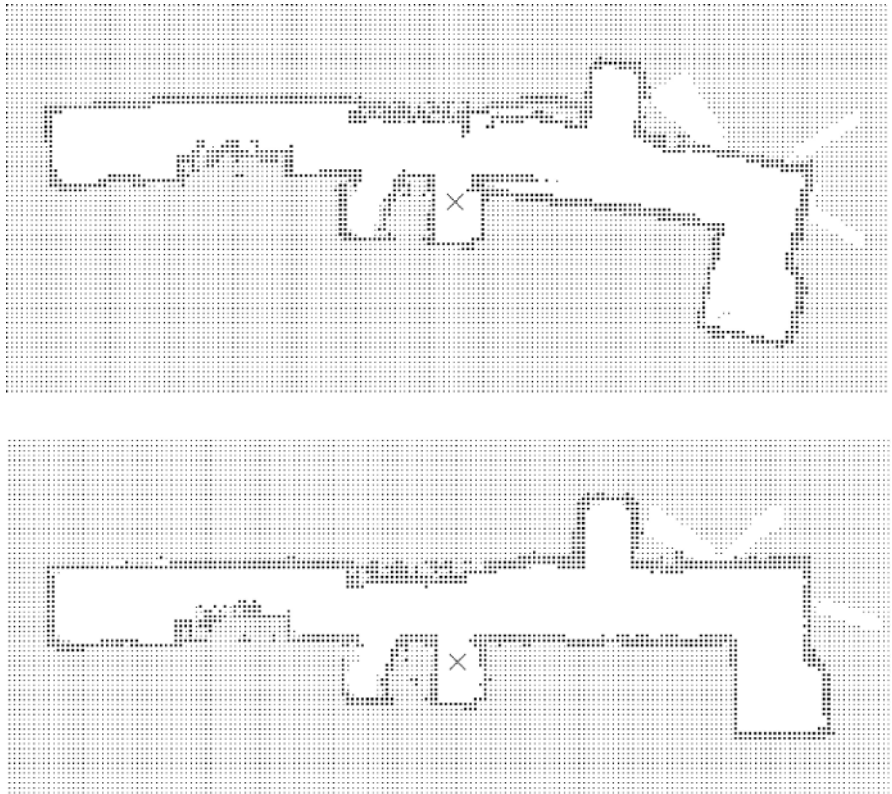
Figure 11.20 Mapping of a 70-foot hall without continuous localization (upper) and with (lower). (Figure courtesy of the Navy Center for Applied Research in Artificial Intelligence, Naval Research Laboratory.)
