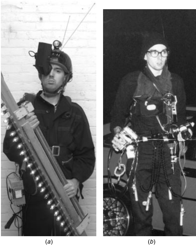
Figure 5.6 Early embodiments of the author’s original “photographer’s assistant” application of personal imaging. (a) 1970s “painting with light vectors” pushbroom” system and 1980 CRT display. The linear array of lamps, controlled by a body-worn processor (WearComp), was operated much like a dot-matrix printer to sweep out spatial patterns of structured light. (b) Jacket and clothing based computing. As this project evolved in the 1970s and into the early 1980s, the components became spread out on clothing rather than located in a backpack. Separate 0.6 inch cathode ray tubes attachable/detachable to/from ordinary safetyglasses, as well as waist-worn television sets replaced the earlier and more cumbersome helmet-based screens of the 1970s. Notice the change from the two antennas in (a) to the single antenna in (b), which provided wireless communication of video, voice, and data to and from a remote base station.
