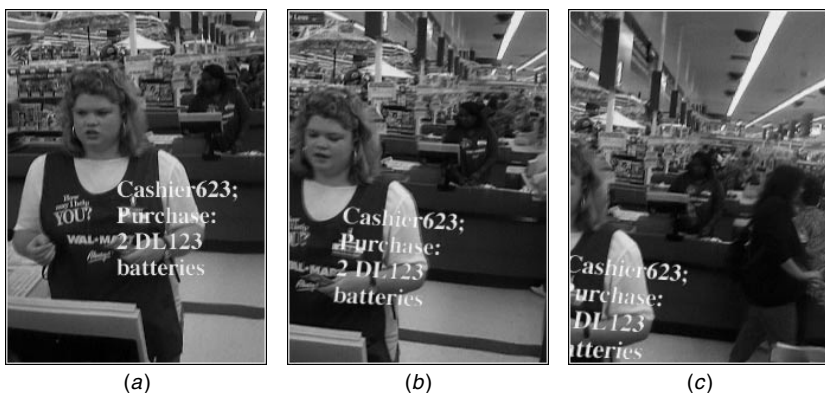
Figure 6.27 Mediated reality as a photographic/videographic memory prosthesis. RWM provides a window into reality, in which the virtual window tracks the real scene to within subpixel accuracy. (a) Wearable face-recognizer with virtual "name tag" (and grocery list) appears to stay attached to the cashier, (b) even when the cashier is no longer within the field of view of the video camera and transmitter (c).
