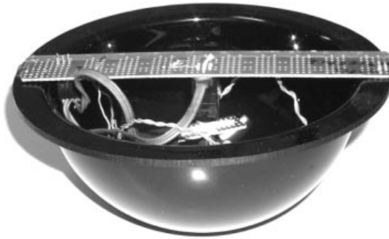
Figure 2.7 Necktie clip portion. The necktie-mounted visual augmented reality system. A smoked plexiglass dome of wine-dark opacity is used to conceal the inner components. Wiring from these components to a body-concealed computer runs through the crack in the front of the shirt. The necktie helps conceal the wiring.
