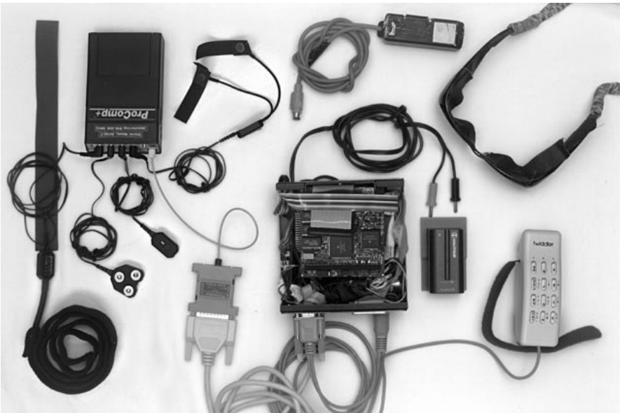
Figure 1.5 Author's personal imaging system equipped with sensors for measuring biological signals. The sunglasses in the upper right are equipped with built in video cameras and display system. These look like ordinary sunglasses when worn (wires are concealed inside the eyeglass holder). At the left side of the picture is an 8 channel analog to digital converter together with a collection of biological sensors, both manufactured by Thought Technologies Limited, of Canada. At the lower right is an input device called the "twiddler," manufactured by HandyKey, and to the left of that is a Sony Lithium Ion camcorder battery with custom-made battery holder. In the lower central area of the image is the computer, equipped with special-purpose video-processing/video capture hardware (visible as the top stack on this stack of PC104 boards). This computer, although somewhat bulky, may be concealed in the small of the back, underneath an ordinary sweater. To the left of the computer, is a serial to fiber-optic converter that provides communications to the 8 channel analog to digital converter over a fiber-optic link. Its purpose is primarily one of safety, to isolate high voltages used in the computer and peripherals (e.g., the 500 volts or so present in the sunglasses) from the biological sensors, which are in close proximity, and typically with very good connection, to the body of the wearer.
