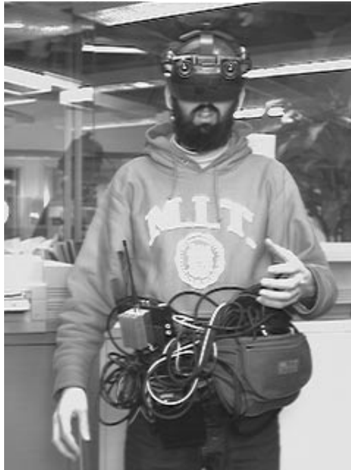
Figure 2.17 An embodiment of author's reality mediator as of late 1994. The color stereo head-mounted display (VR4) has two cameras mounted to it. The intercamera distance and field of view match approximately author's interocular distance and field of view with the apparatus removed. The components around author's waist comprise radio communications equipment (video transmitter and receiver). The antennas are located at the back of the head-mount to balance the weight of the cameras, so that the unit is not front-heavy. ©Steve Mann, 1994.
