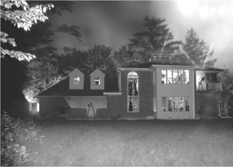
Figure 5.24 Output of antihomomorphic lightvector image processing. This picture was mathematically generated from a number of differently illuminated pictures of the same subject matter, in which the subject matter was illuminated by walking around with a bank of flash lamps controlled by a wearable computer system in wireless communication with another computer controlling a camera at a fixed base station. (©) Steve Mann, 1985 .
