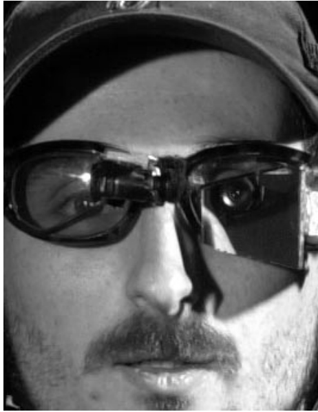
Figure 3.25 Eyeglass-based EyeTap system (left eye tapped by camera and aremac).
