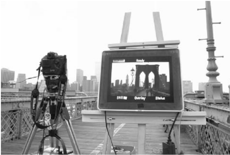
Figure 3.13 Various cameras with television outputs are set up on the walkway, but none of them can recreate the subject matter behind the television display in a manner that conveys a perfect illusion of transparency, because the subject matter does not exist in a single depth plane. There exists no choice of camera orientation, zoom setting, and viewer location that creates an exact illusion of transparency for the portion of the Brooklyn Bridge blocked by the television screen. Notice how the railings don't quite line up correctly as they vary in depth with respect to the first support tower of the bridge.
