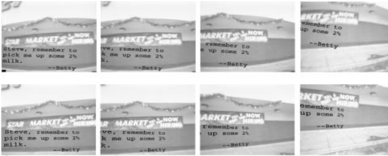
Figure 6.28 Virtual message left on the wall under the entrance to the grocery store. When the recipient of the message approaches the store wearing a reality mediator, the message left there will suddenly appear. As the wearer moves his/her head, the message will appear to be attached to the wall. This is because the homography of the plane is tracked, and a projective coordinate transformation is performed on the message before it is inserted into the wearer's reality stream. (Top) Lens distortion in WearCam results in poor registration. (Bottom) After correcting for lens distortion using the Campbell method [106] the sub-pixel registration is possible. (Data captured by author and processed later on base station; thanks to J. Levine for assisting author in porting VideoOrbits to SGI architecture used at base station.)
