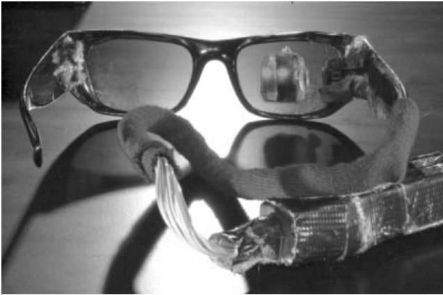
Figure D.4 Completed covert eyeglass rig: Here only the right eye position is shown wired. The second eye (left eye) position has not yet been installed. A second eyeglass safety strap and a second display is next installed. Both can now be tested with the M1 drive circuit. The next step is to build a smaller circuit that drives two Kopin CyberDisplays. Not shown in this system is the installation of the cameras, which are each reflected off the back of the optical element used for the display.
