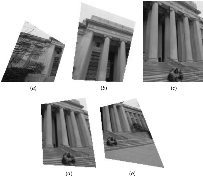
Figure 6.13 Frames from original image video orbit after a coordinate transformation to move them along the orbit to the reference frame (c). The coordinate-transformed images are alike except for the region over which they are defined. The regions are not parallelograms; thus methods based on the affine model fail.
