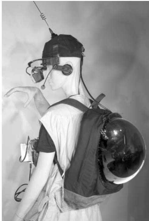
Figure 2.9 Early personal safety device (PSD) with radar vision system designed and built by the author, as pictured on exhibit at List Visual Arts Center, Cambridge, MA (October 1997). The system contains several sensing instruments, including radar, and camera systems operating in various spectral bands, including infrared. The headworn viewfinder display shows what is behind the user when targets of interest or concern appear from behind. The experience of using the apparatus is perhaps somewhat like having eyes in the back of the head, but with extra signal processing as the machine functions like an extension of the brain to provide visual intelligence. As a result the user experiences a sixth or seventh sense as a radar vision system. The antenna on the hat was for an early wireless Internet connection allowing multiple users to communicate with each other and with remote base stations.
