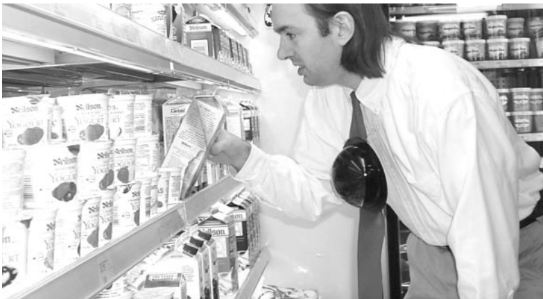
Figure 2.6 Wearable portion of apparatus, as worn by author. The necktie-mounted visual augmented reality system requires no headwear or eyewear. The apparatus is concealed in a smoked plexiglass dome of wine-dark opacity. The dark dome reduces the laser output to safe levels, while at the same time making the apparatus blatantly covert. The dome matches the decor of nearly any department store or gambling casino. When the author has asked department store security staff what's inside their dark ceilings domes, he's been called "paranoid," or told that they are light fixtures or temperature sensors. Now the same security guards are wondering what's inside this dome.
