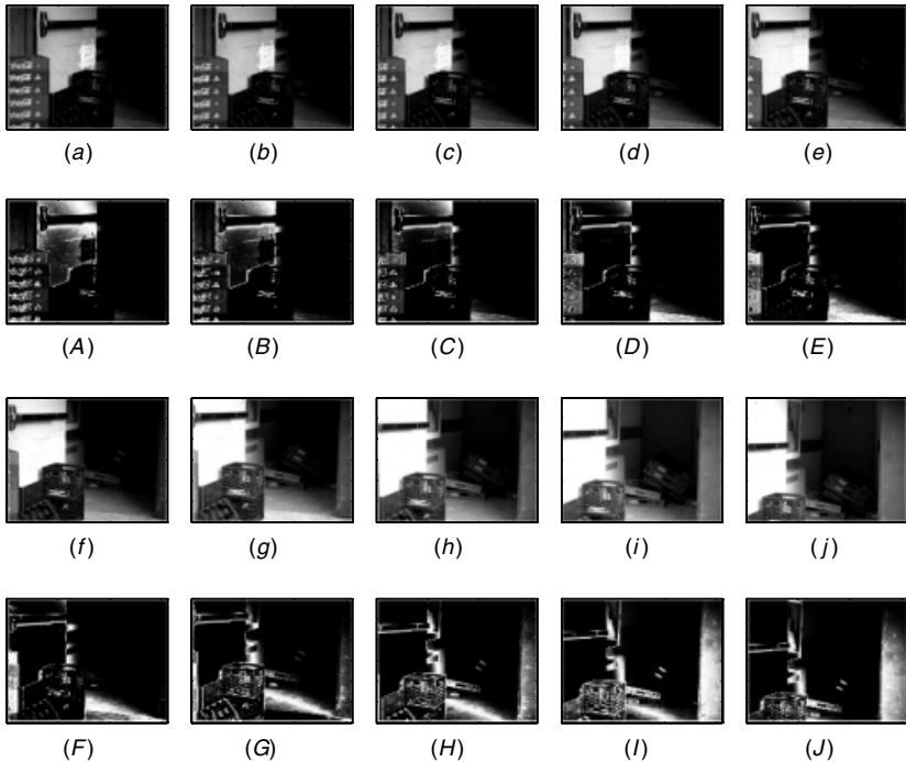
Figure 6.19 The fire-exit sequence, taken using a camera with AGC. (a)–(j) frames 0 to 9: As the camera pans across to take in more of the open doorway, the image brightens and shows more of the interior, while at the same time, clipping highlight detail. Frame 0 (a) shows the writing on the white paper taped to the door very clearly, but the interior is completely black. In frame 5 (f) the paper is completely obliterated. It is so washed out that we cannot even discern that there is a paper present. Although the interior is getting brighter, it is still not discernible in frame 5 (f), but more and more detail of the interior becomes visible as we proceed through the sequence, showing that the fire exit is blocked by the clutter inside. (A)–(J) “certainty” images are corresponding to (a) to (j).
