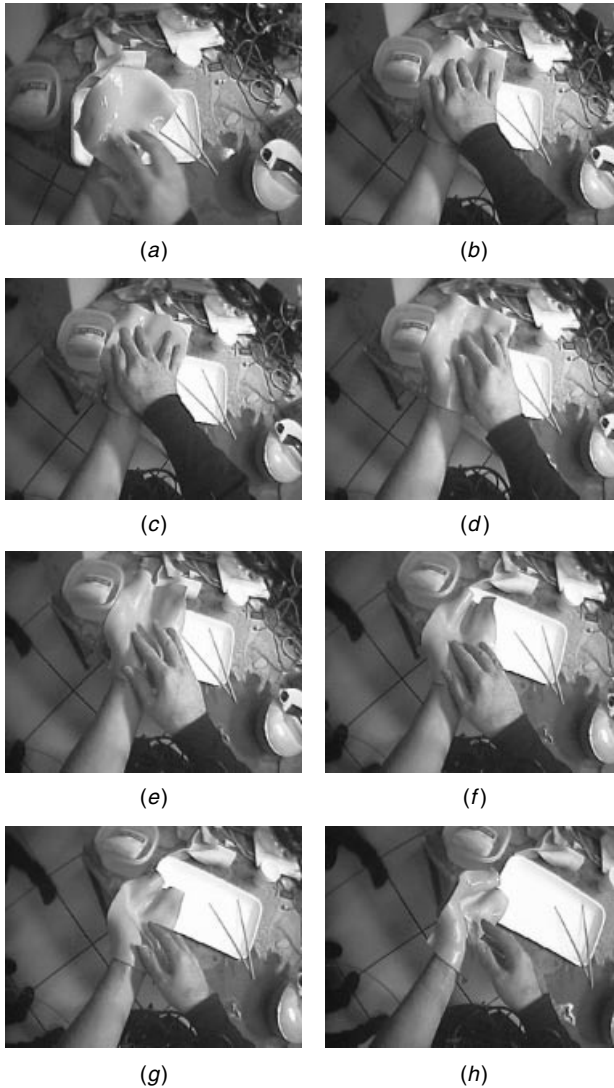
Figure B.3 Shaping the soft-heated plastic to perfectly fit the hand. (a) Here a left-handed keyer is in the making; (b–c) soft-heated plastic is pressed down to form nicely between the fingers so that the keyer will conform perfectly to the hand’s shape; (d–h) when the right hand’s taken away, the material should feel comfortable and naturally stay in position on the left hand.
