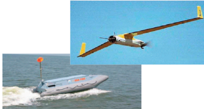
Fig. 1. The Insitu Group Seascan UAV (Top) and the Northwind Marine Seafox USV (Bottom)
