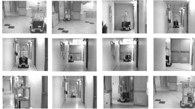
Fig. 15. Experiment combining visual path following for door traversal and topological navigation for corridor following
