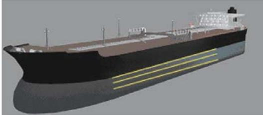
Figure 3: The horizontal slice method; the vehicle makes passes at constant depth.
