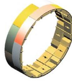
Figure 4: Two consecutive rings of the formwork. Each ring consists of eight segments.
