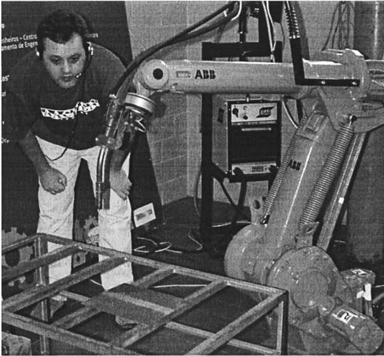
Figure 4.9 Shell of the voice interface application showing the welding operation, and a user (author of this book) commanding the robot using a headset microphone
