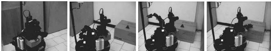
Fig. 13.12. Full calibration: after the laser and the binocular systems are calibrated, the robot can navigate and reach objects in 3-D accurately
