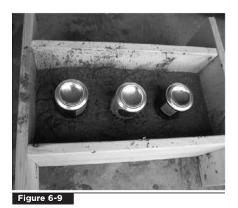
Pour your papier-mâché concrete slump to just a little over full into the mold. Tap on the mold with a hammer to help settle the slump.
