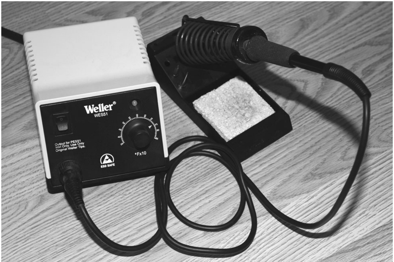
Figure I-23 A midrange heat-controlled soldering iron.
