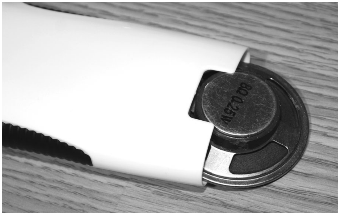
Figure 10-16 Making a simple pillow speaker.
