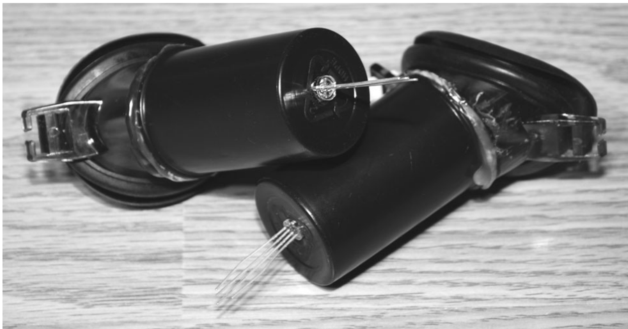
Figure 18-9 Diffuser tubes glued to the goggles.
