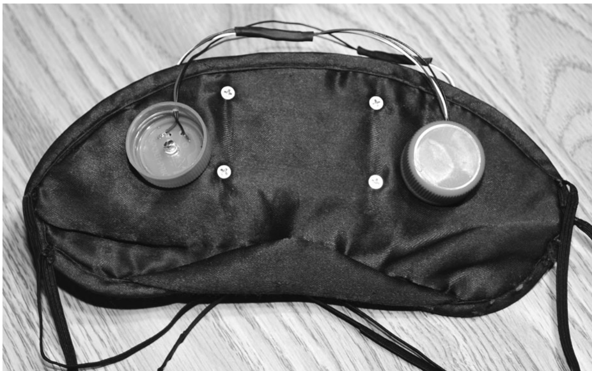
Figure 12-7 Installing the hardware onto the sleep mask.
