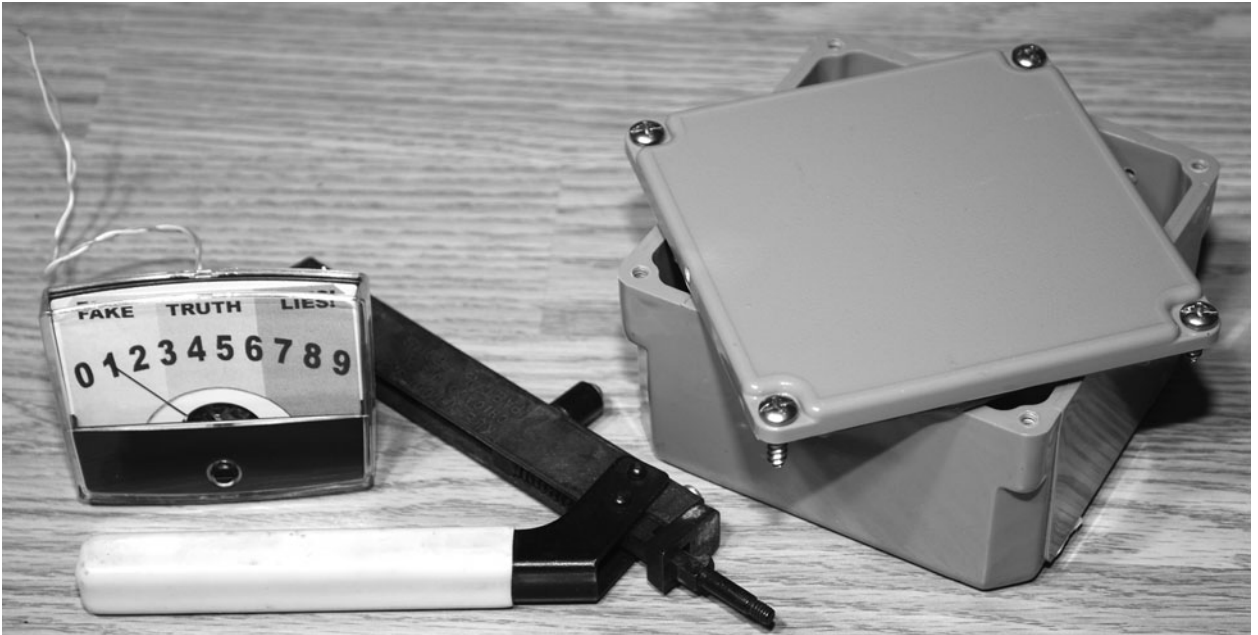
Figure 6-8 A notching tool is great for cutting square holes.
