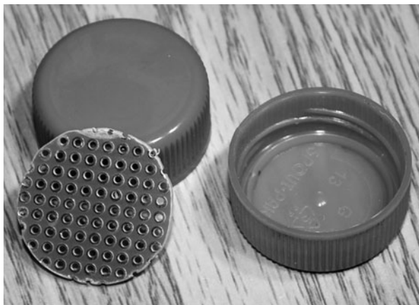
Figure 12-3 Cutting a small perf board to fit the bottle cap.
