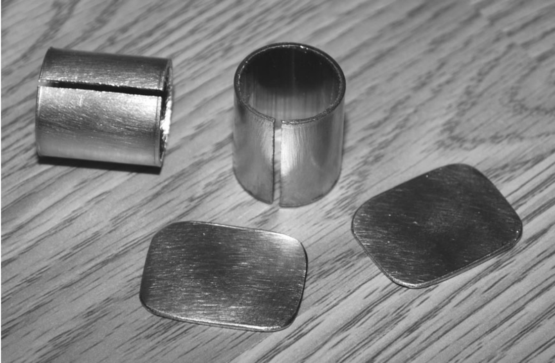
Figure 1-8 Making finger and body probes.
