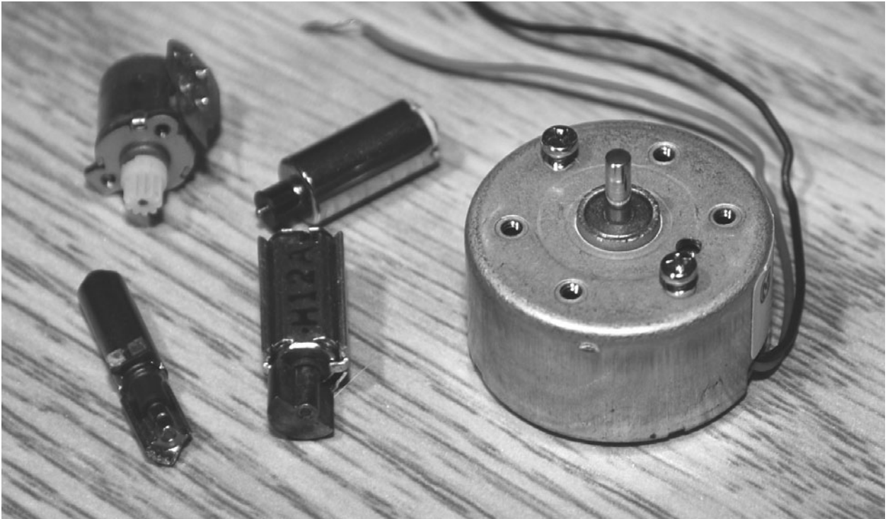
Figure 9-3 Small dc motors that can make vibrations.
