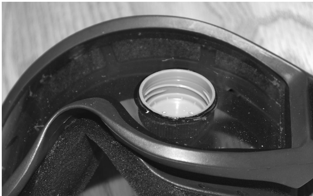
Figure 11-9 Inserting the cap through the lens hole.
