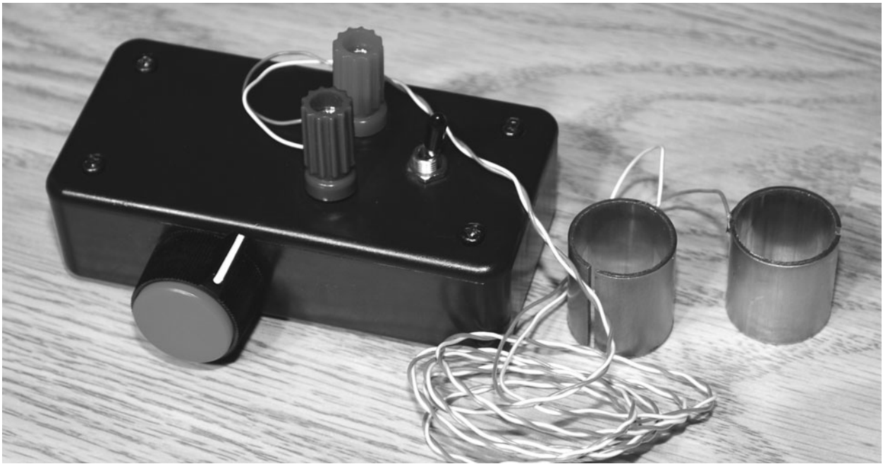
Figure 1-10 The completed biofeedback device and probes.
