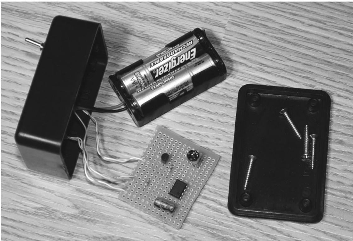
Figure 15-8 Putting together the oscillator unit.
