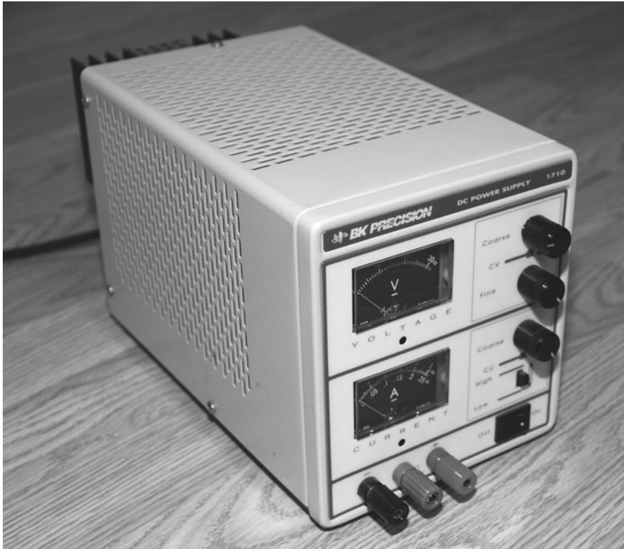
Figure I-24 A variable dual power supply.
