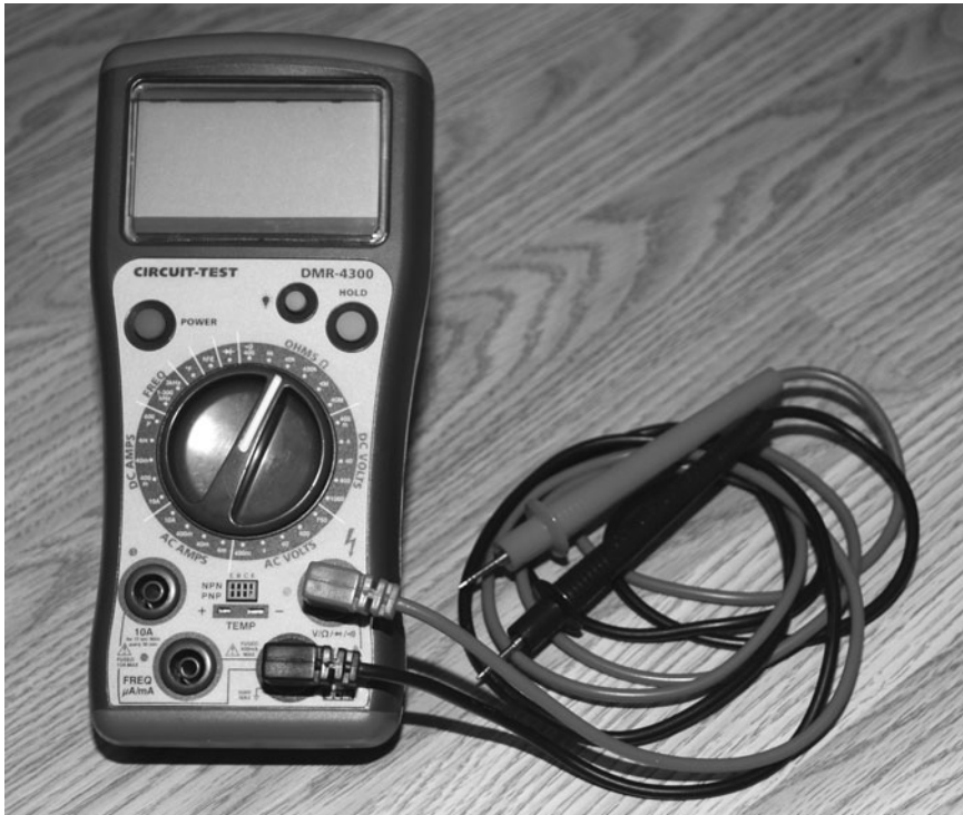
Figure I-25 A basic digital multimeter.
