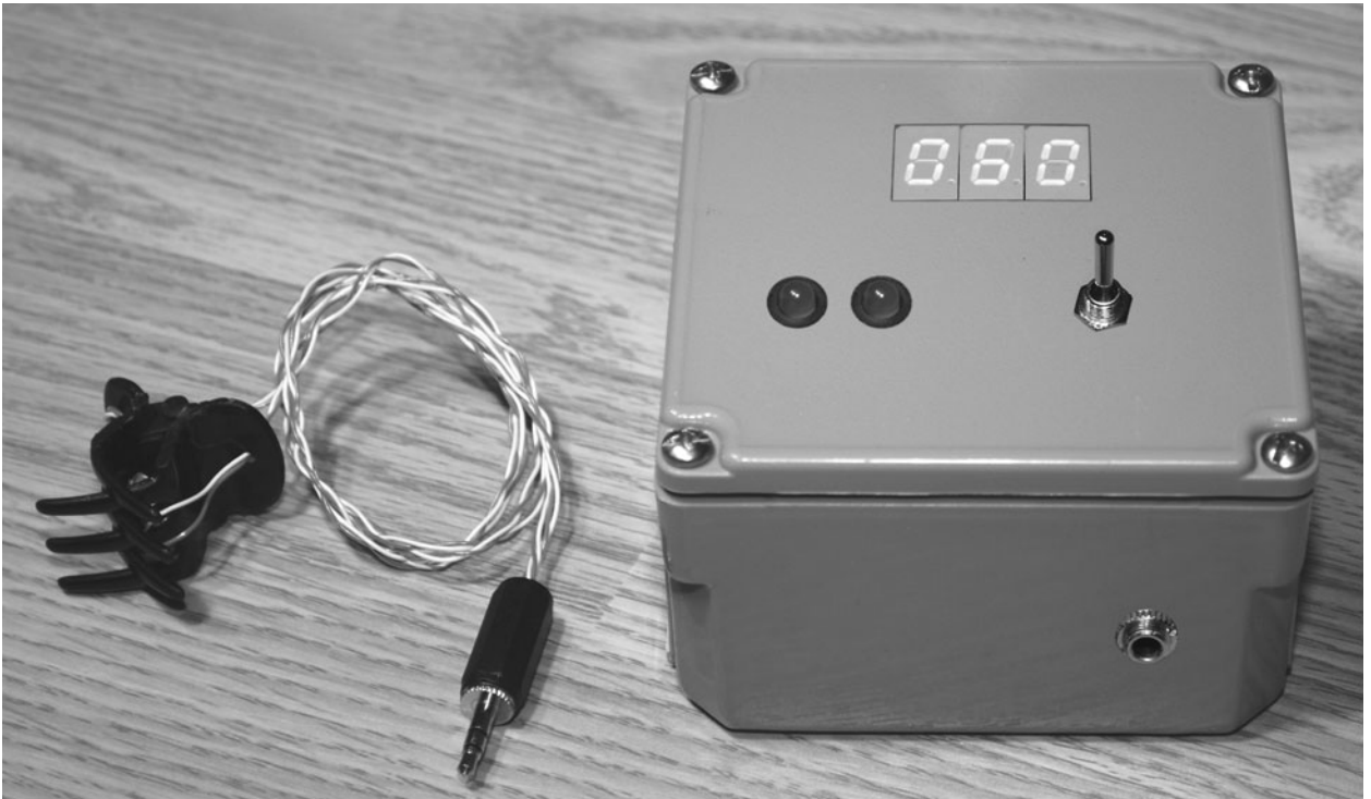
Figure 5-12 The completed heart rate monitor.
