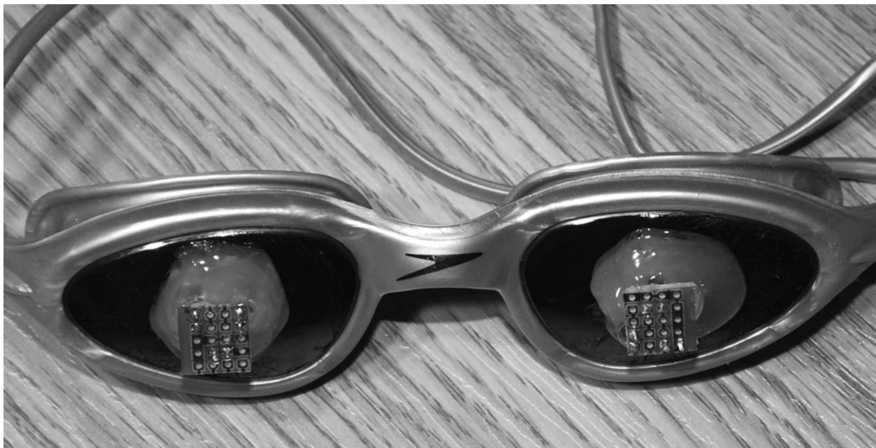
Figure 15-6 Mounting the LEDs to the goggles.
