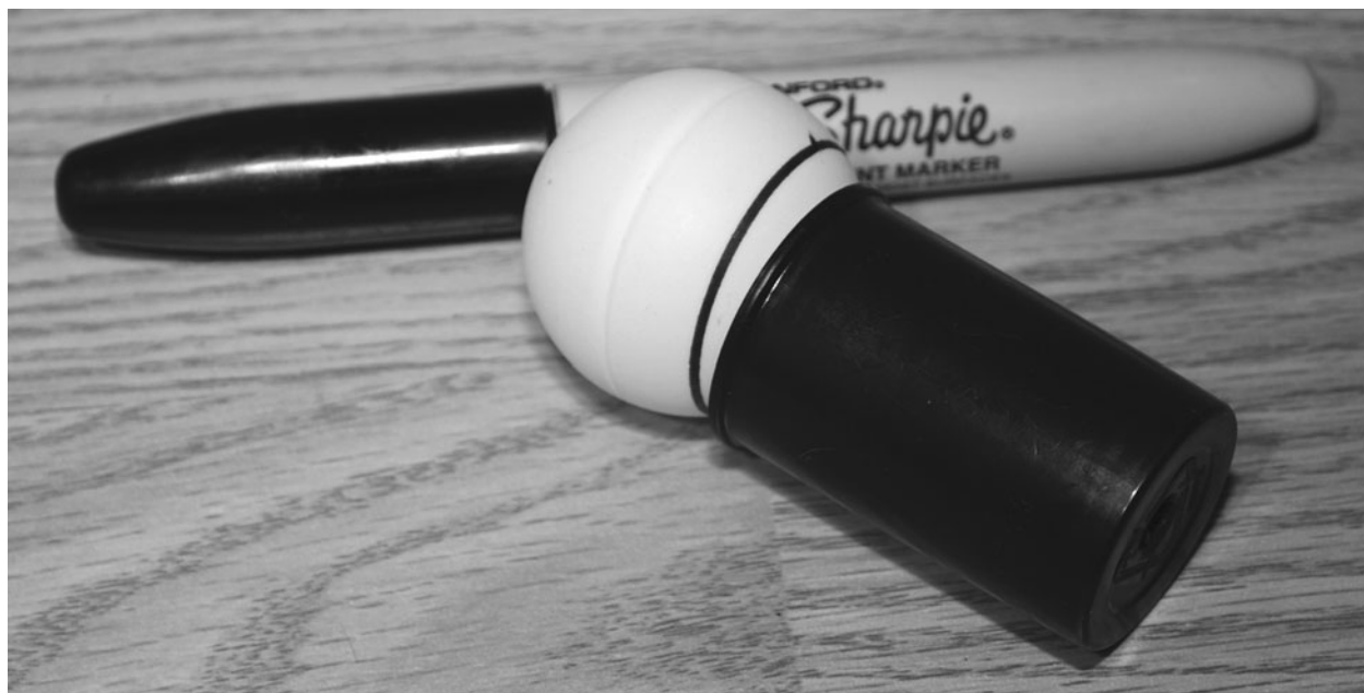
Figure 18-7 Making a diffuser tube for the goggles.
