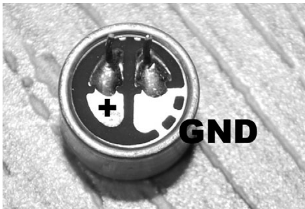
Figure 4-3 Electret microphones are polarized.
