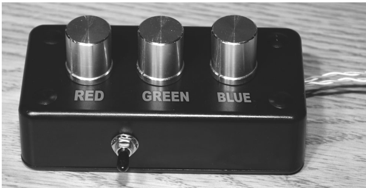
Figure 18-11 The completed color-therapy control box.
