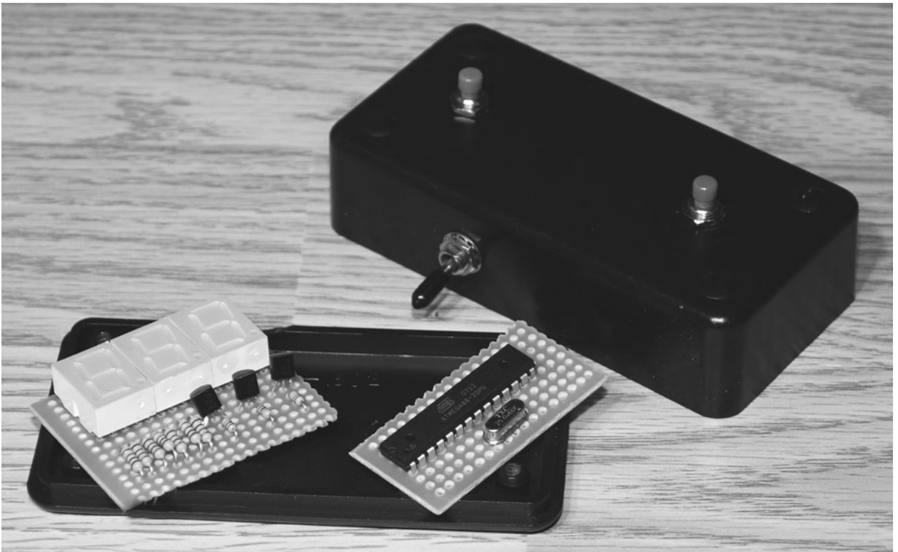
Figure 16-4 Deciding on a cabinet and board layout.
