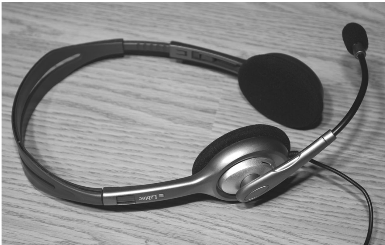
Figure 4-4 A headset containing an electret microphone.
