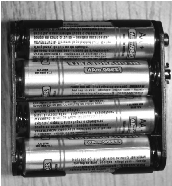
Figure 2-7 Six volts from four batteries.
