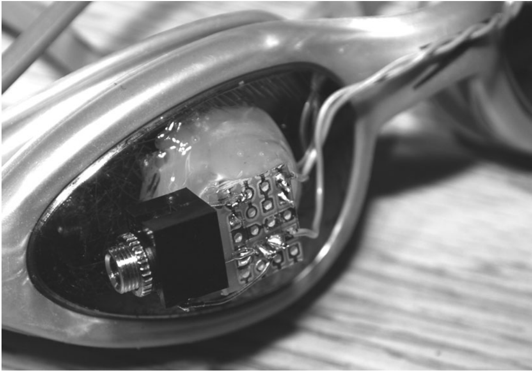
Figure 15-7 Wiring the LEDs for external access.
