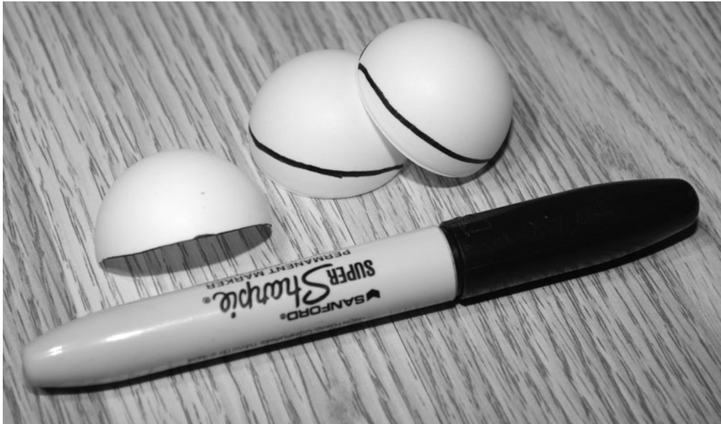
Figure 14-4 Shaping the ball halves to conform to your face.
