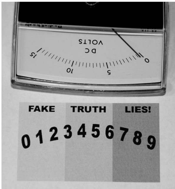
Figure 6-4 Making a replacement readout plate.
