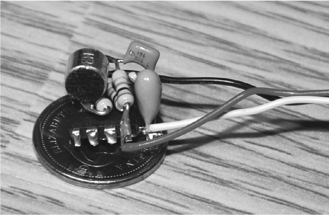
Figure 4-6 Building a circuit without a circuit board.
