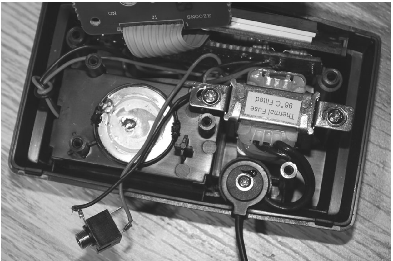
Figure 10-7 Adding an alarm output jack.
