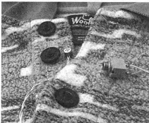
Figure 2-17 A small microphone will hide behind a button with a hole drilled through it.
