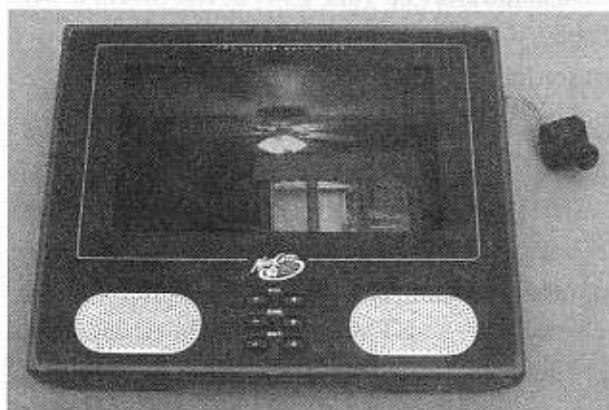
Figure 5-2 A small LCD monitor is a great tool for spot checking video.
