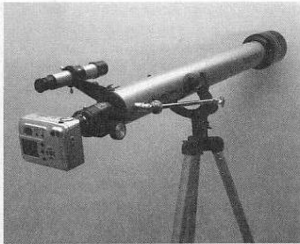
Figure 4-14 An adapter made from a Barlow lens holds the camera to the eyepiece.
