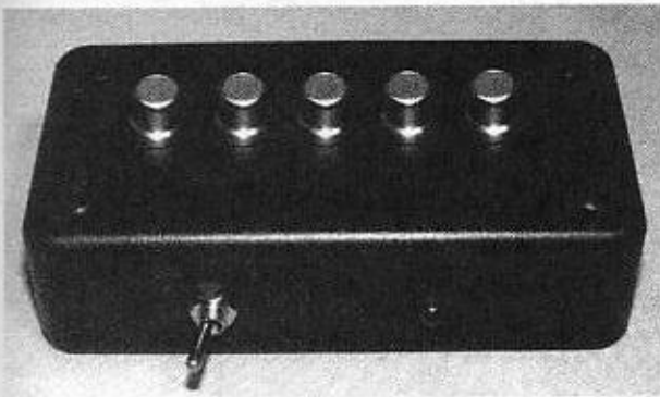
Figure 5-10 The multiple camera auto switcher completed.
