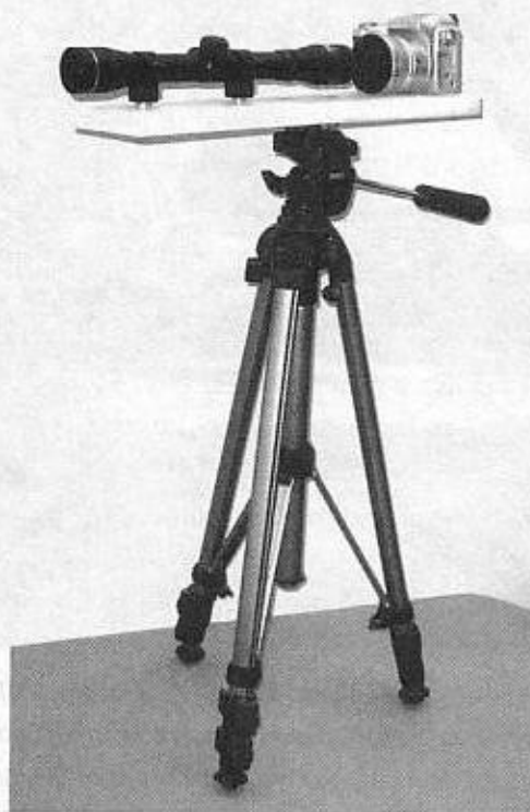
Figure 4-11 Camera and gun sight mounted to a strip of nylon plastic.
