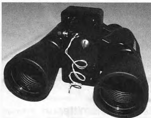
Figure 14-3 The plastic container is bolted to the binocular shell.
