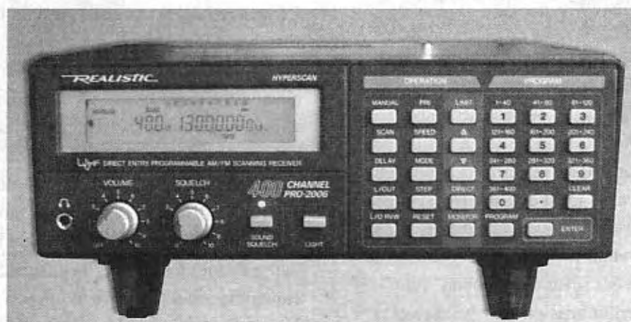
Figure 12-1 A typical radio scanner base unit.
