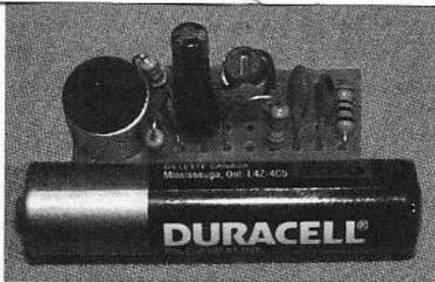
Figure 9-11 The completed FM transmitter with 1.5-volt power source.
