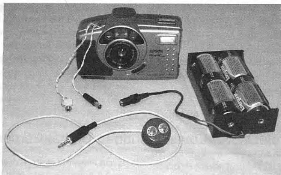
Figure 4-5 Wiring modifications completed for external power and trigger switch.
