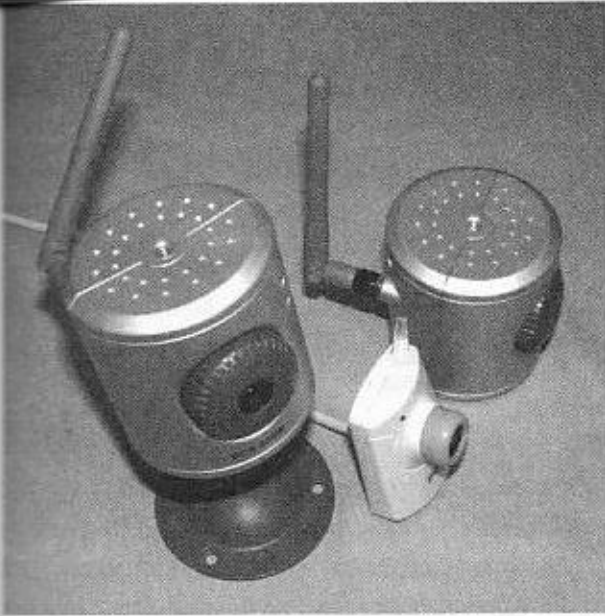
Figure 5-13 A few basic web cameras used for long-range video surveillance.
