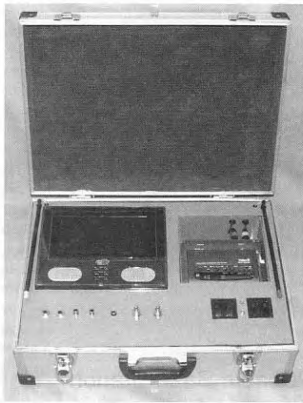
Figure 15-24 A professional-looking portable base station built into a briefcase.
