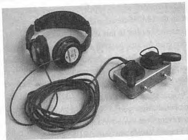
Figure 2-9 Completed bionic stereo spy ears.
