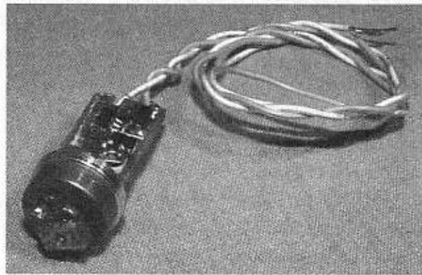
Figure 8-16 A hacked green laser pointer reduced to the diode and driver board.
