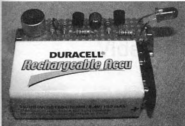
Figure 9-20 The invisible light transmitter listening to every whisper in a room.
