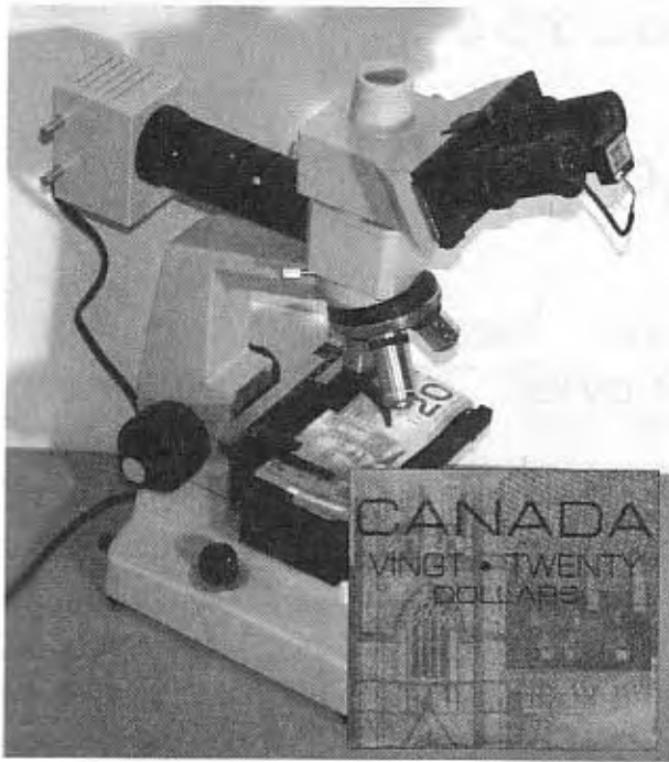
Figure 6-15 Currency is examined and recorded using a microscope and video camera.
