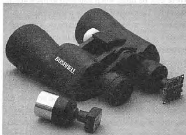
Figure 6-13 A pair of lens caps glued together form a removable eyepiece adapter.
