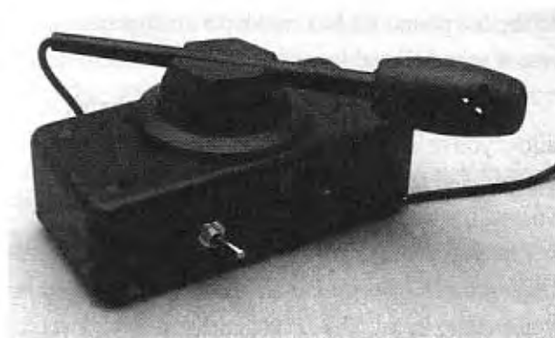
Figure 3-15 The voice changer is built into a small box for hand held operation.
