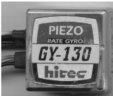
Figure 2.9: HiTec piezo gyroscope, Seika inclinometer
