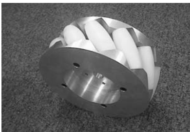
Figure 8.1: Mecanum wheel designs with rollers at 45°
