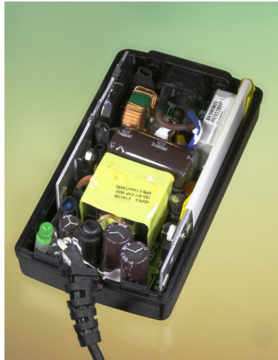
Figure 16-6. The interior of the type of switching power supply that powers a laptop computer.
