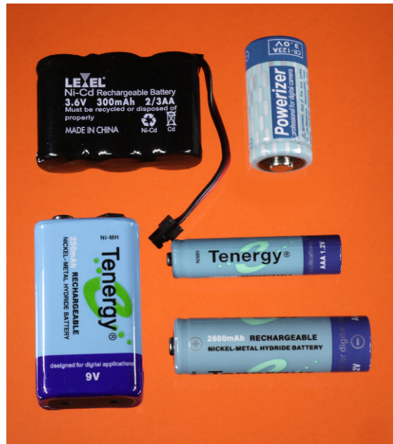
Figure 2-9. Top left: NiCad battery pack for a cordless phone. Top right: Lithium battery for a digital camera. The other batteries are rechargeable NiMH substitutes for everyday alkaline cells.
