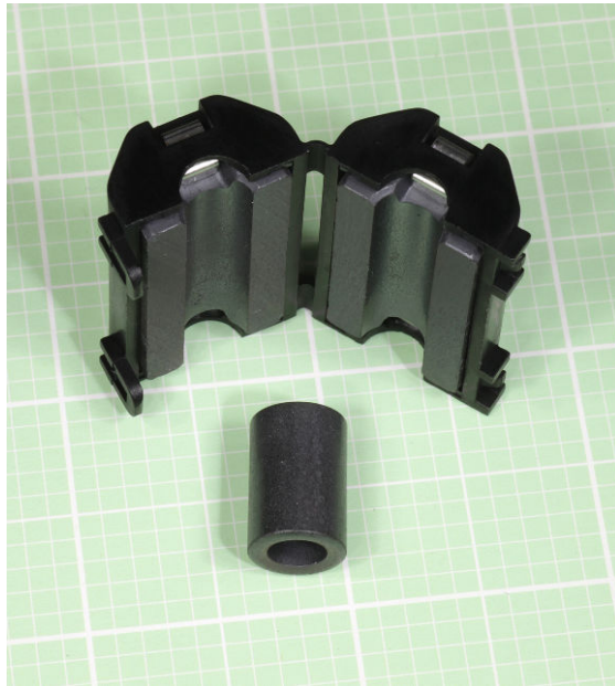
Figure 14-13. Two examples of ferrite beads. They can inhibit radio-frequency radiation from a wire, or protect the wire from interference.
