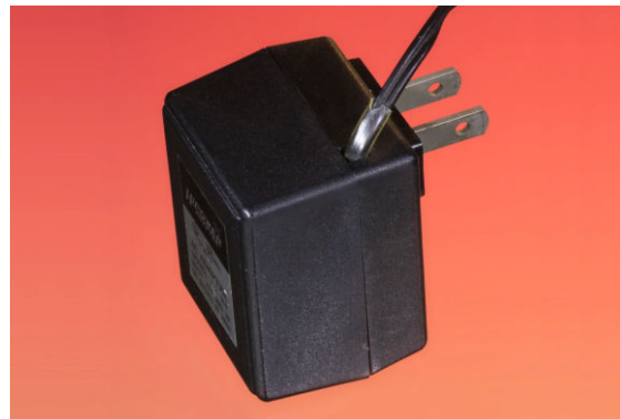
Figure 16-2. A simple transformer-based power supply can be encapsulated in a plastic shell, ready to plug into a power outlet. However, today this format more typically contains a switching power supply, which is usually lighter, smaller, and cheaper.
