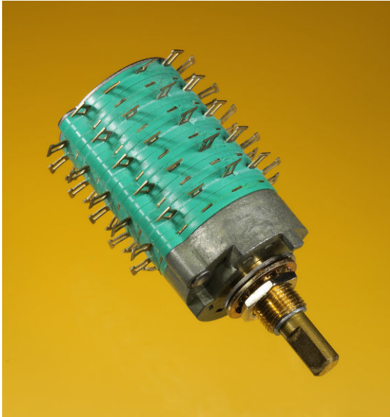
Figure 7-4. A five-pole, twelve-position rotary switch.
