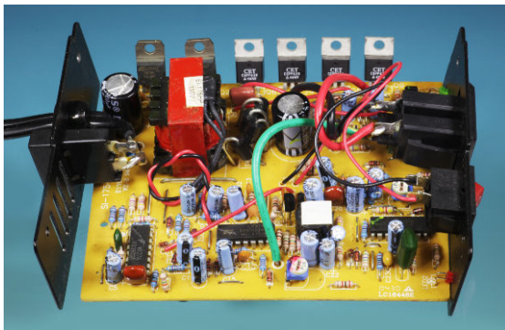
Figure 18-1. The interior components in a 175-watt inverter.
