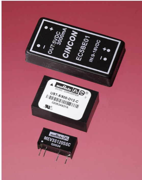
Figure 17-7. A selection of sealed DC-DC converters.
