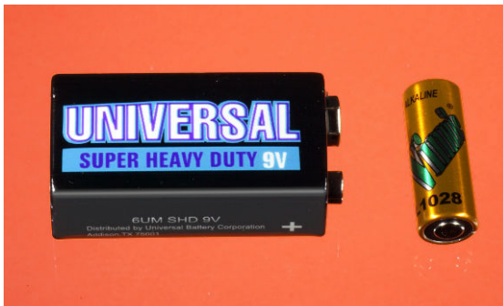
Figure 2-7. At left, a cheap carbon-zinc battery; at right, a 12V alkaline burglar-alarm battery. See text for additional details.
