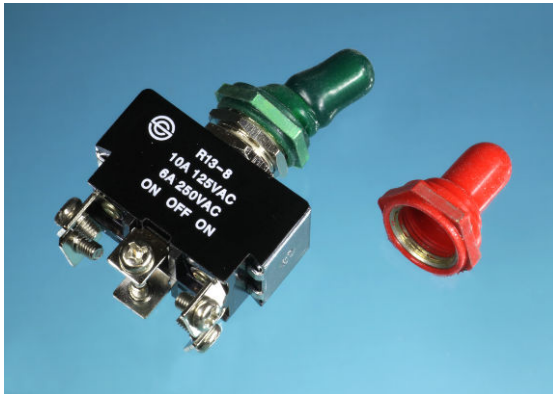
Figure 6-14. A rubber or vinyl boot can be used to protect a toggle switch from contamination with dirt or water. Each boot contains a nut that screws onto the threads of a toggle switch, as shown at left.
