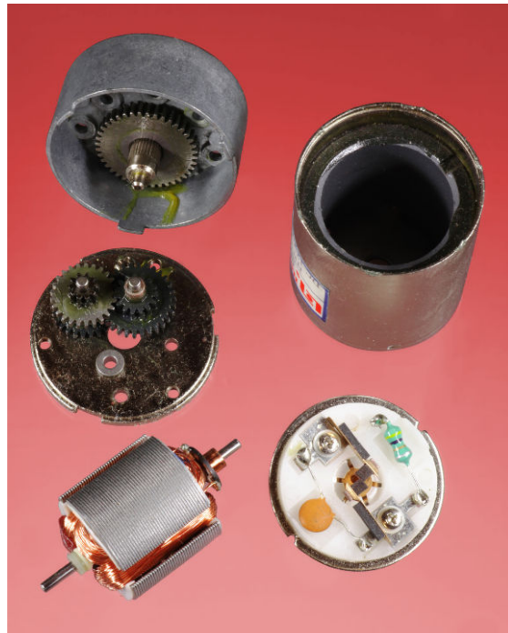
Figure 22-7. Spur gears from a gearhead motor provide speed reduction and increased torque.
