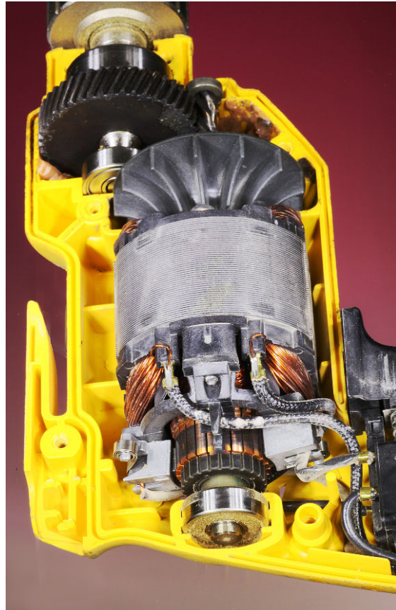
Figure 23-12. A motor in a corded electric drill uses coils in a brushed rotor to enable variable speed output. In most AC motors, the speed is not adjustable and the rotor does not make any electrical connection with the rest of the motor.
