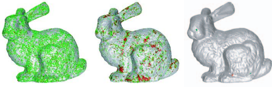
Fig. 6.26. The evolution and progress in the Cocone family of algorithms, illustrated on the Stanford bunny, 36k points. From left to right: Cocone, Tight Cocone and Robust Cocone. Triangles featuring non manifold edges and vertices are colored
