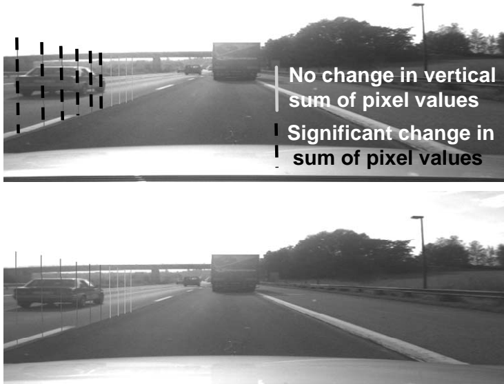
Figure 11.31. A vehicle moving through the columns in the image most likely will produce changing values of the sums; these columns are marked as dashed dark lines . Their vertical extension symbolized distance at the lane boundary. To determine range to a changing feature, its horizontal distance from the lane marking has to be taken into account.
