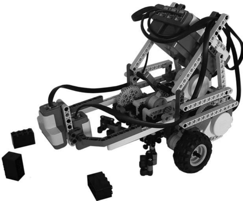
Figure 7-1. The Mine Sweeper is equipped with a ravine-avoidance sensor. The mines shown here are built using two black 2 × 4 LEGO bricks.
