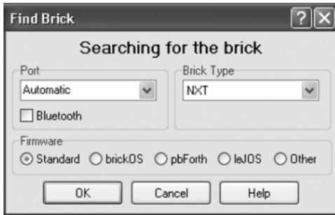
Figure A-1. The Find Brick form that shows up when you open BricxCC
