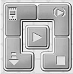
Figure 2-7. The NXT controller, which you can find in the right bottom of the software main window
