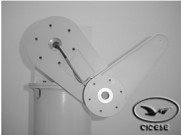
Figure 5.1. Pelican: experimental robot arm at CICESE, Robotics lab.
