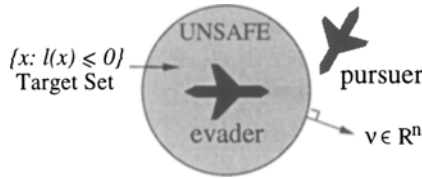
Fig. 5.1. The evader and pursuer, with Target set and its outward pointing normal \nu
