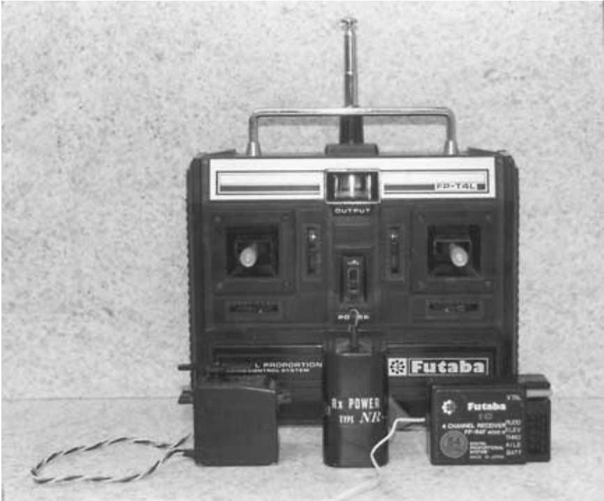
FIGURE 4-1. Three-channel remote control system.
