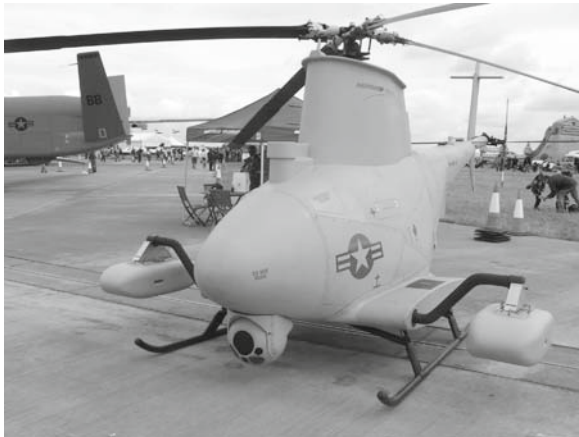
Fig. 1.8 MQ-8B unmanned helicopter used by the US Marine Corps and the US Navy, manufactured by Northrop Grumman
