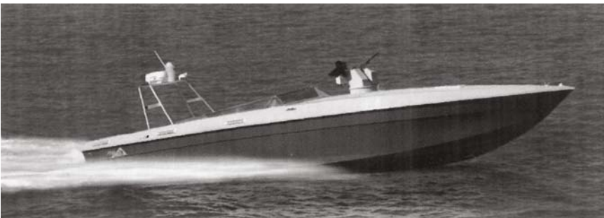
Fig. 1.7 Silver Marlin unmanned surface vessel with autonomous obstacle avoidance, manufactured by Elbit Systems (Courtesy of Oreet International Media Ltd.)
