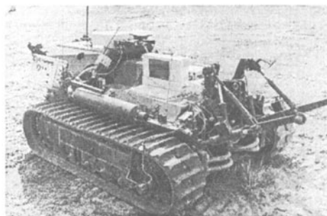
Fig. 4b: An autonomous prototype vehicle, which can be used e.g. for pulling trunks out of forest (Modulaire Ltd.)
