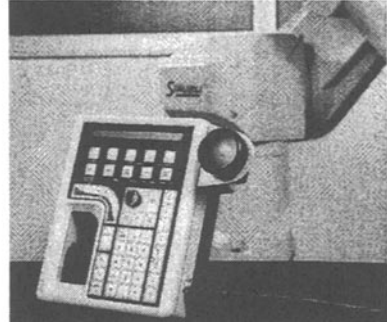
Fig. 13 SPACE MOUSE is used now by different leading robot manufacturers in their control panels (KUKA left, STÄUBLI right)
