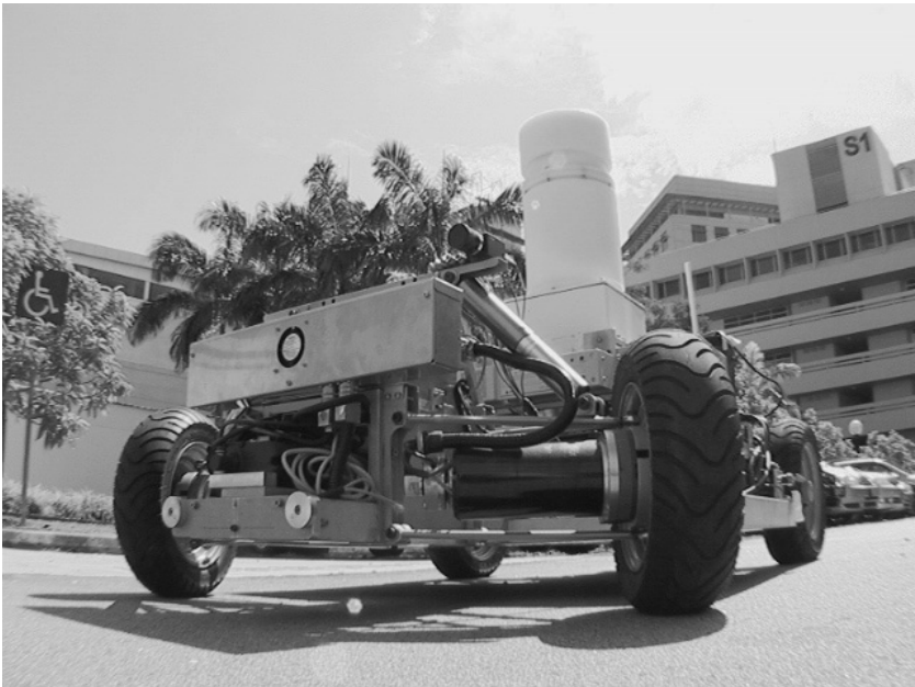
FIGURE 2.1 A 360° scanning MMW RADAR mounted on a vehicle test bed for SLAM experiments within the NTU campus.
