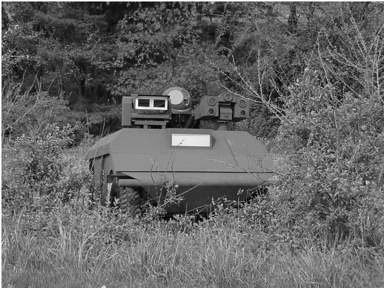
FIGURE 17.16 The Army Demo III experimental unmanned vehicle. On the left-top is the LADAR. In the center-top is a Reconnaissance Camera ball. On the right-top is a pan/tilt unit with a color stereo pair, a FLIR stereo pair, and a color high resolution monocular camera. The white panel in the center front is for a radar. The front bumper is instrumented to detect obstacles hidden in the weeds. (Photo courtesy of General Dynamics Robotic Systems.)
