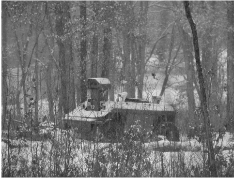
FIGURE 17.17 An Army Demo III experimental unmanned vehicle driving autonomously through the woods during a snow storm at Ft. Indiantown Gap, Pennsylvania, in January 2003.
