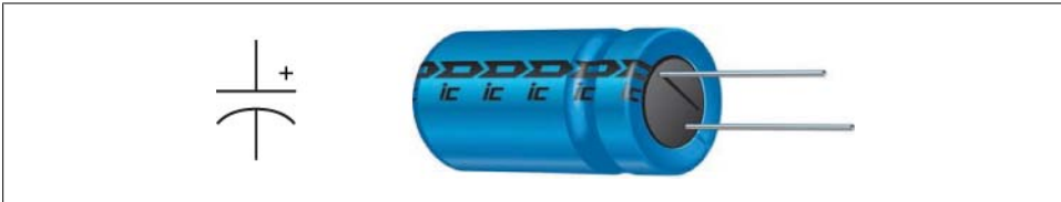
Figure 11-3. The electrical symbol for a capacitor and a representation of a capacitor
