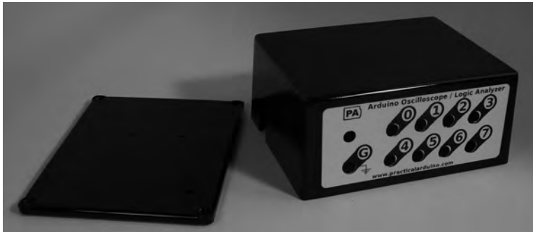
Figure 11-5. Front panel label in place with holes drilled
