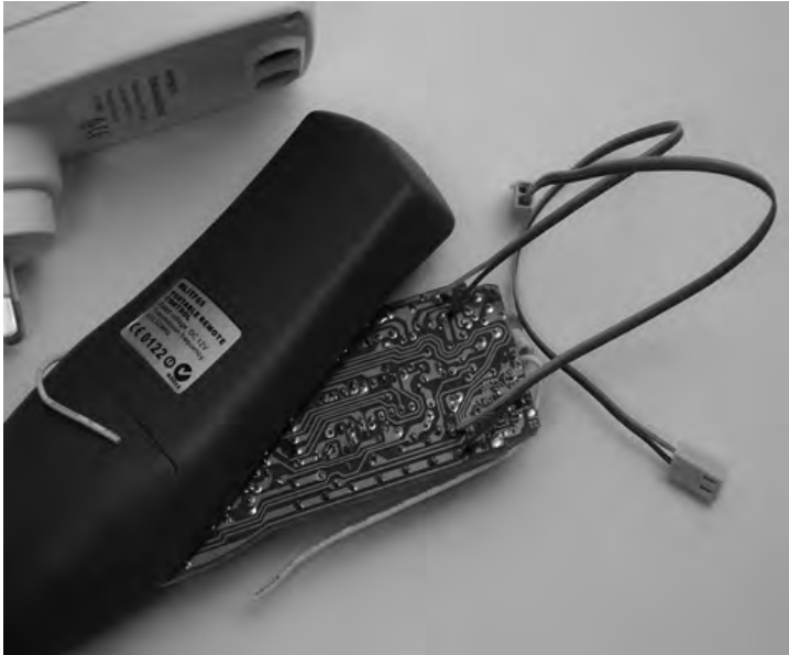
Figure 2-11. Remote control transmitter with connections in place
