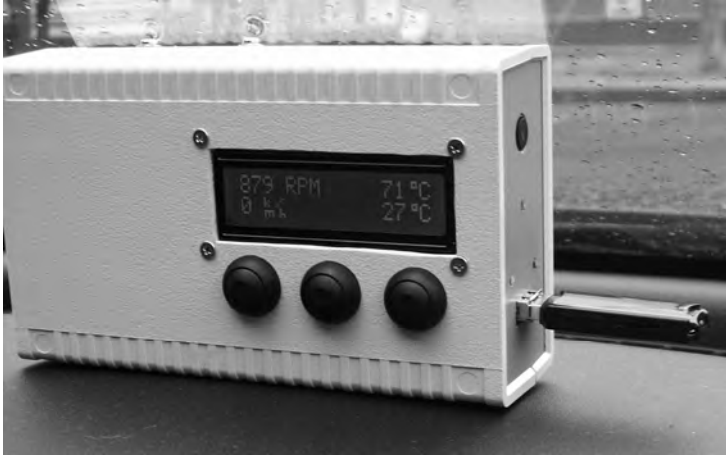
Figure 15-32. The complete system assembled in a case with USB memory stick attached
