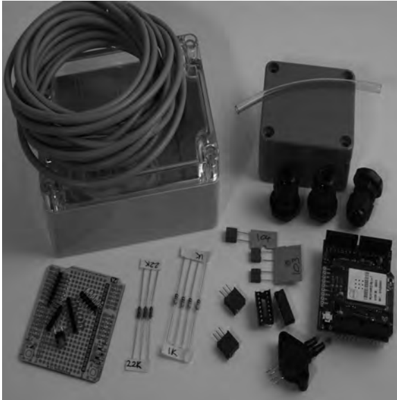
Figure 12-1. Parts required for water tank depth sensor
