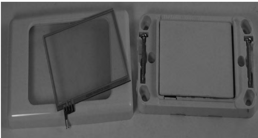
Figure 8-7. Wall plate with removed piece glued back in place behind its original location
