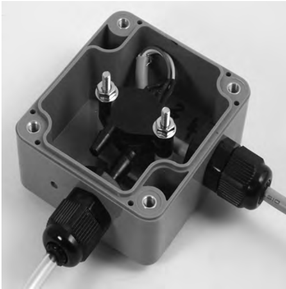
Figure 12-13. Transducer box fully assembled and ready to be closed up
