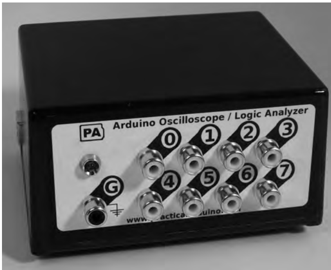
Figure 11-6. Connectors and LED mounted in front panel
