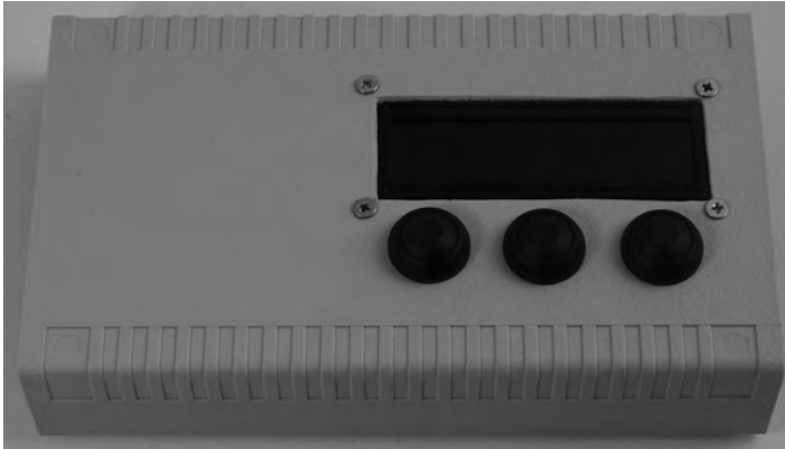
Figure 15-28. The LCD and menu buttons mounted in the case
