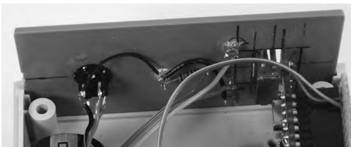
Figure 15-31. The Logging button and status LEDs glued into the front panel
