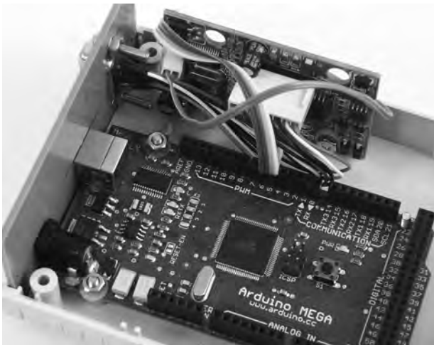
Figure 15-26. The Arduino Mega mounted on plastic spacers with the USB socket protruding through the back panel
