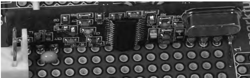
Figure 13-8. RXB1 receiver mounted on shield
