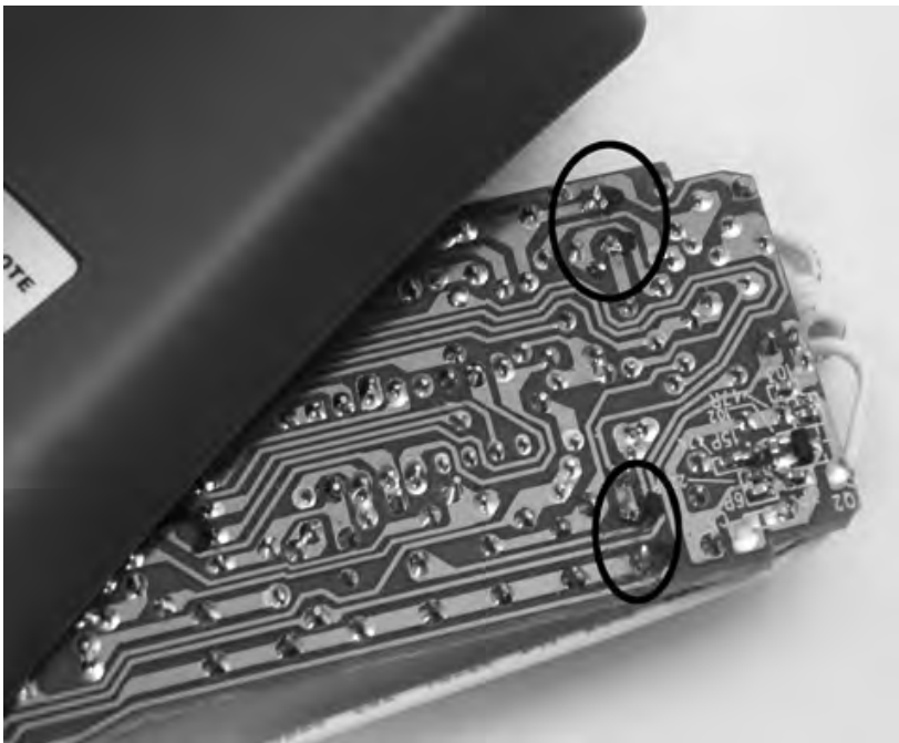
Figure 2-4. PCB of appliance remote control transmitter
