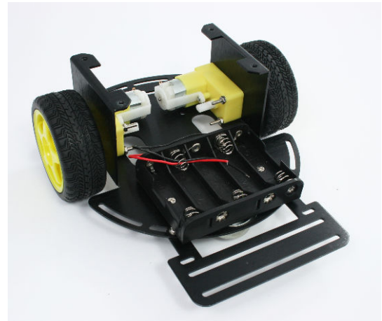
Figure 3-11. Chassis with Battery Pack Attached
