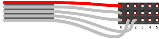
Figure 2-13. Ribbon cable connections to shield pins
