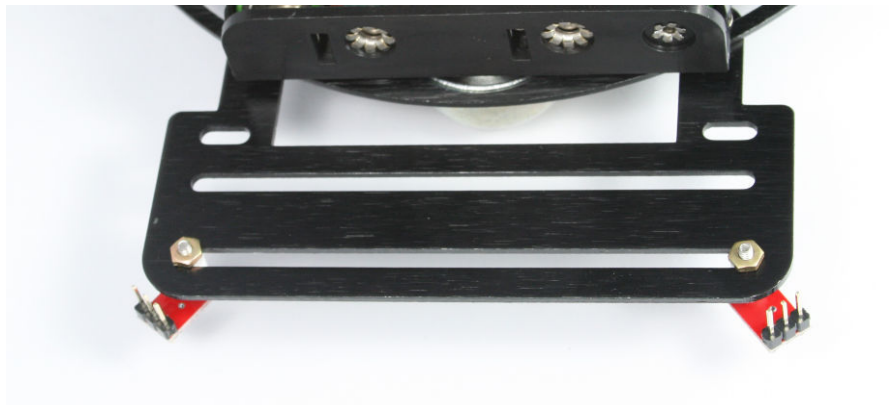
Figure 3-27. Reflectance Sensor location for Edge Detection
