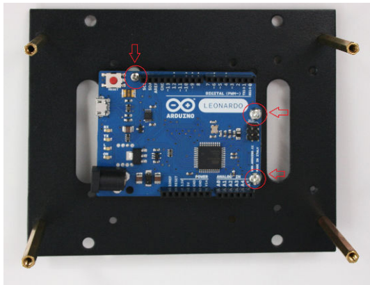
Figure 4-22. Arduino board mounted using three spacers
