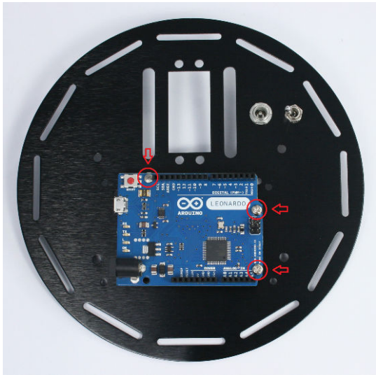
Figure 3-22. Mounting the Arduino board as viewed from the top of the chassis
