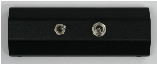
Figure 4-9. Rear panel switch and power jack assembly viewed from the front
