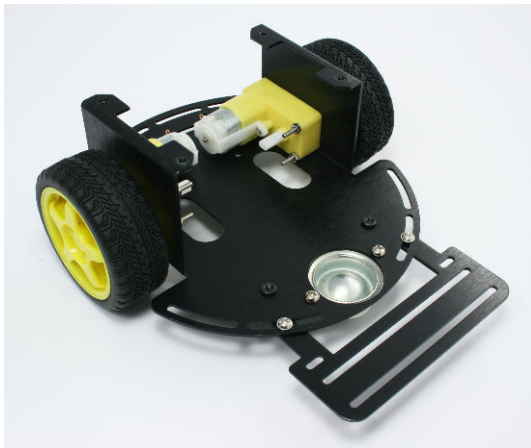
Figure 3-8. Sensor bracket viewed with the robot right side up
