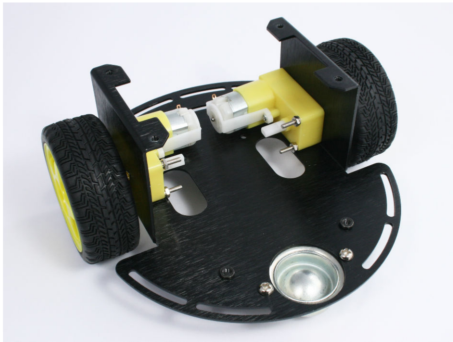
Figure 3-7. Wheels and caster mounted
