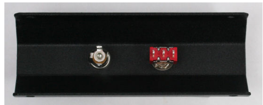
Figure 4-10. The other side of the panel showing the switch orientation and power jack
