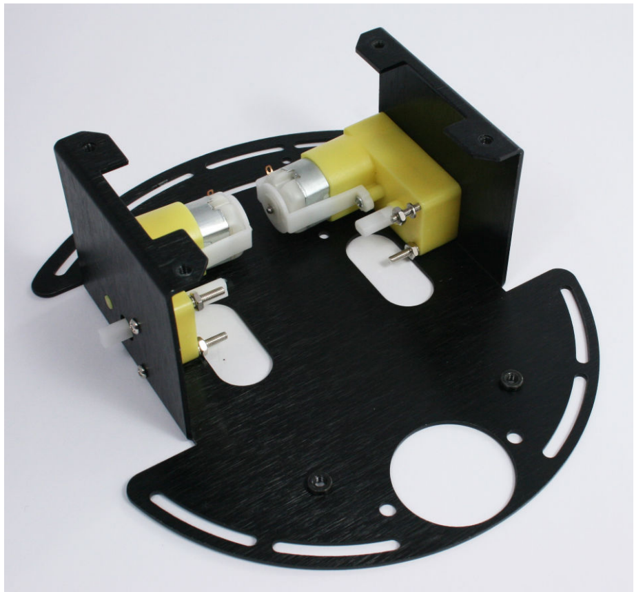
Figure 3-4. Motors mounted on the chassis lower plate
