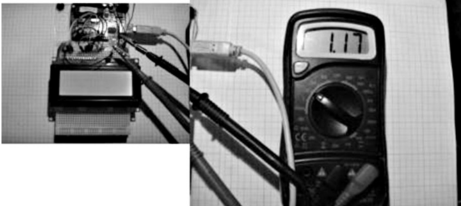
Figure 8-24. Measuring the DC voltage at pin 3 of the LCD with the electrical tape removed from the CdS cell
