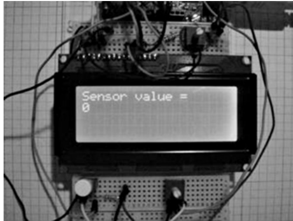
Figure 8-27. Low-cost proto-evaluation breadboard. The push-button switch and potentiometer allow quick evaluation of the Manual Counter and Read Sensor sketches.
