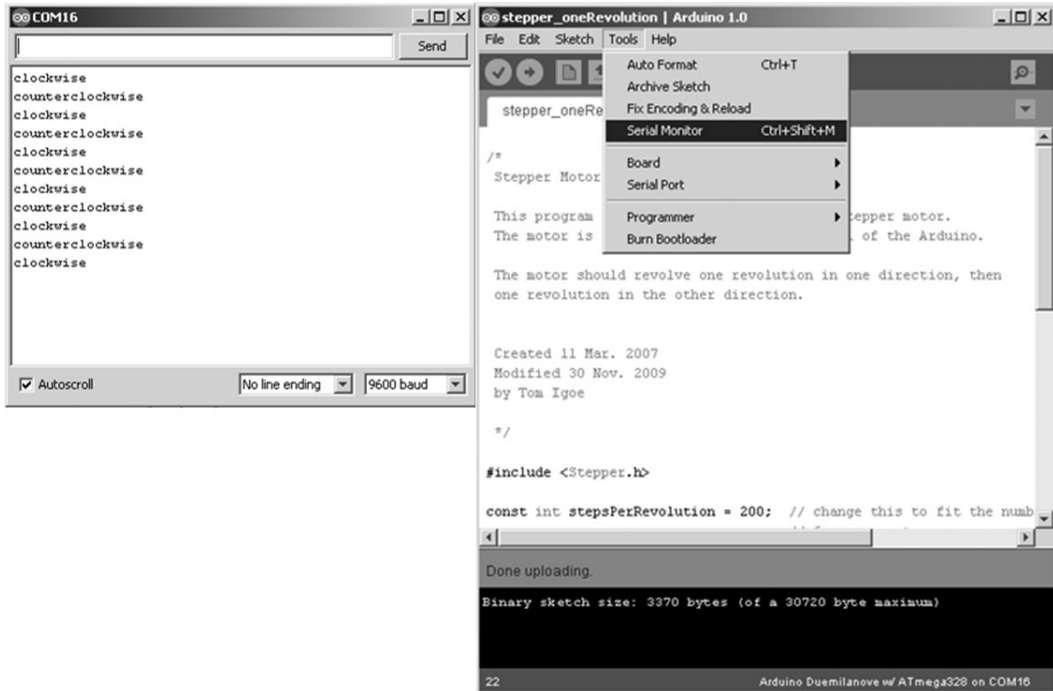
Figure 5-34. Gaining access to the Serial Monitor for viewing messages within the Arduino Processing IDE
