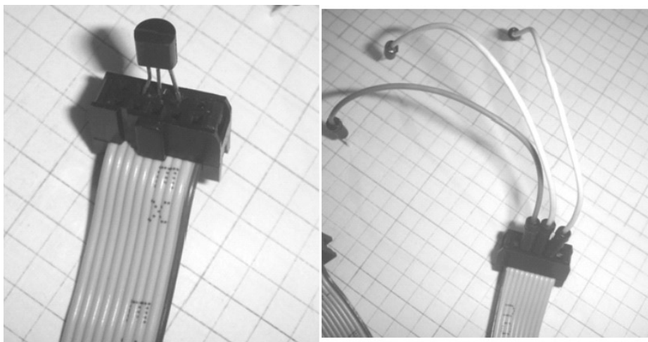
Figure 10-5. Close-up of ribbon end connectors with attached temperature sensor and jumper wires
