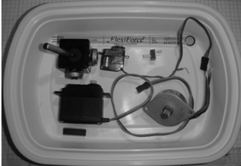
Figure 5-1. Parts required for motion control servo and stepper motor projects and experiments
