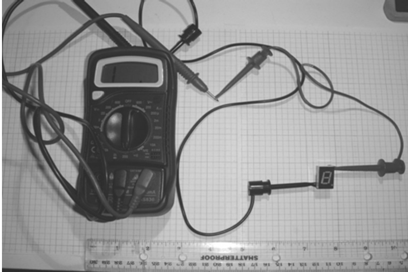
Figure 2-17. Testing a seven-segment LED display (common anode) with a DMM set to ohmmeter mode
