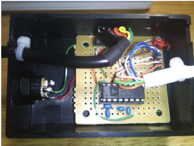
Figure 6-22. Inside the PC side box. Cable exiting on the left is the FTDI USB cable; below that is the DC jack. White cable exiting on the right is to the sensor.
