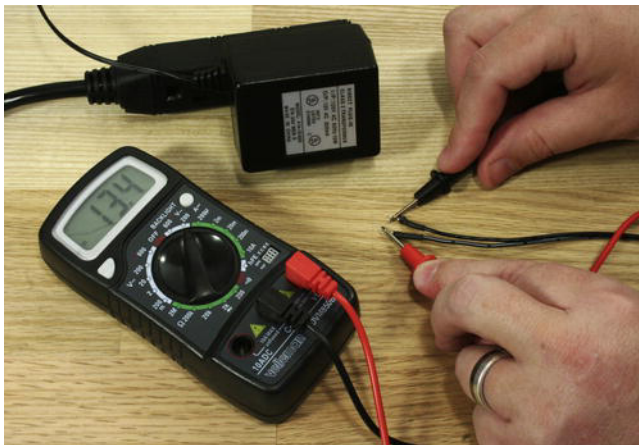
Figure 7-11. Measuring AC adapter voltage
