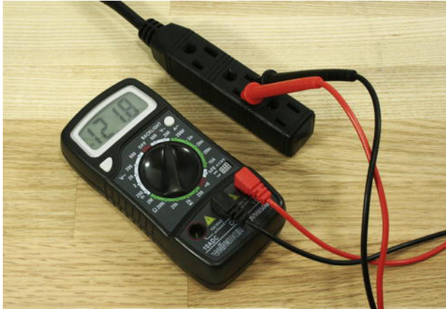
Figure 7-10. Measuring AC mains voltage
