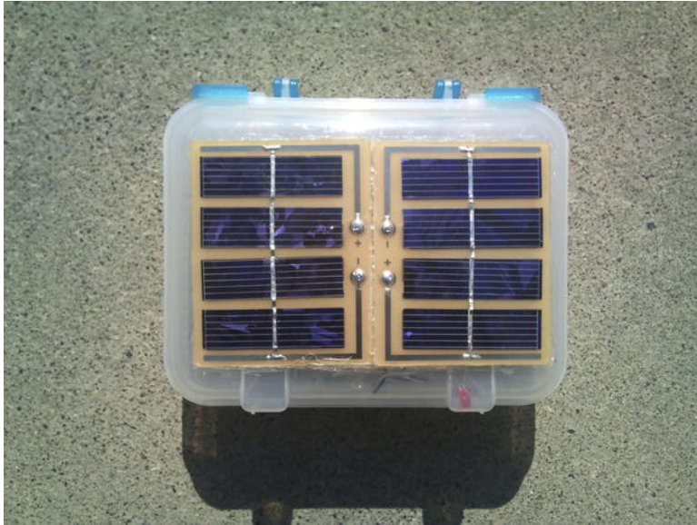
Figure 3-12. Solar panels mounted to the outside of a plastic box
