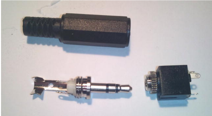
Figure 2-11. 1/4-inch phono plug, plug jacket, and panel mount jack
