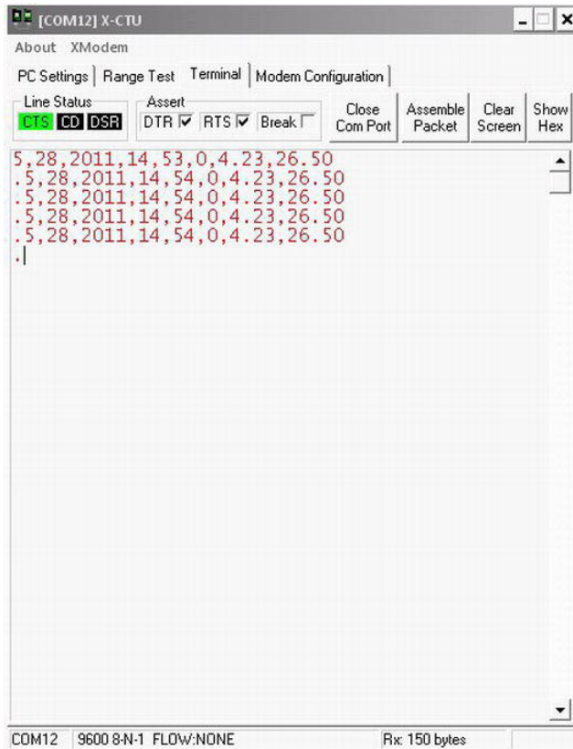
Figure 4-5. The X-CTU terminal window with data streaming from the end node
