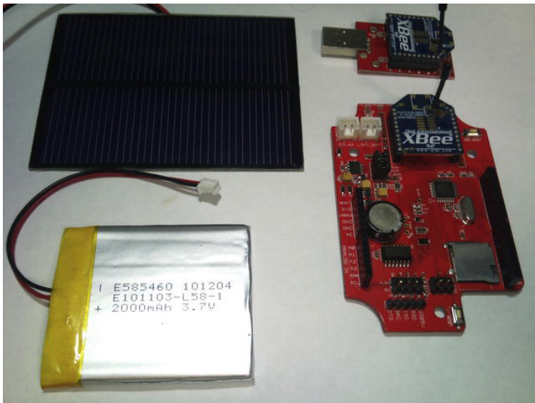
Figure 3-4. The Dangerous Prototypes Stalker V2, with LiPo battery, solar panel, Xbee radio, and a USB Xbee dongle
