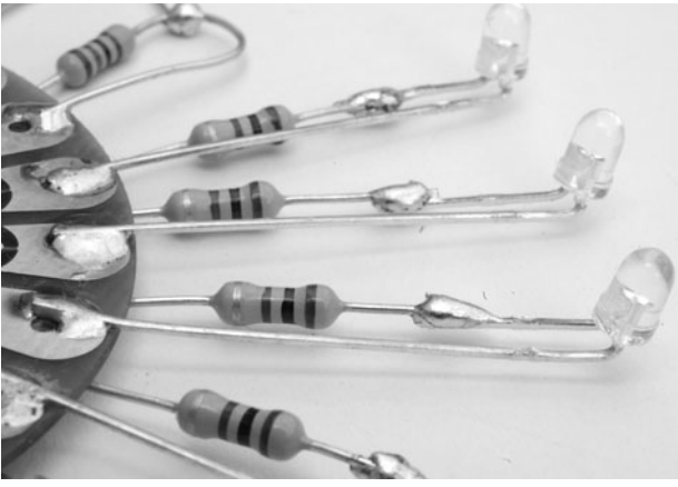
Figure 9-13 Close-up of LED attached to a resistor.
