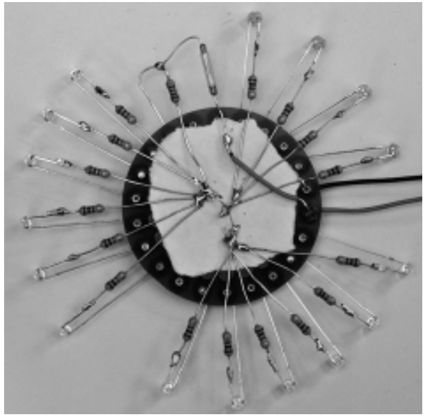
Figure 9-14 Bottom side of Lilypad board.
