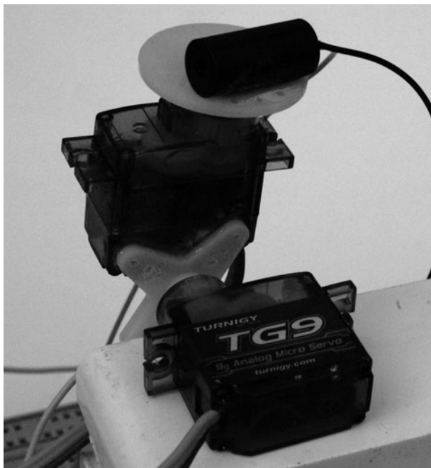
Figure 8-15 Servo and laser assembly.
