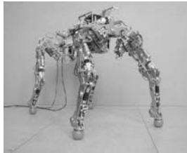
Fig. 3. The quadrupedal walking machine BISAM. Due to the five active degrees of freedom in the body and the ability to rotate the shoulder and hip, BISAM implements key elements of mammal-like locomotion.
