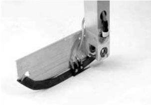
Fig. 3. In practice, we obtained the best results with a foot radius of 25 [cm], a foot length of 13 [cm], and a forward displacement of 6 [cm]. The foot switch allows the controller to adapt to the actual step time by registering the exact instant of heel strike
