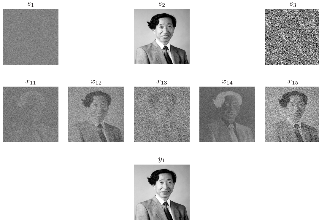
Fig. 5.13 Exemplary computer simulation results for mixture of three 512 \times 512 image signals, where s_j and x_{1j} stand for the j -th original images and mixed images, respectively, and y_1 the image extracted by the extraction processing unit shown in Fig. 5.6. The learning algorithm (5.91) with q = 1 was employed [68, 1142].
