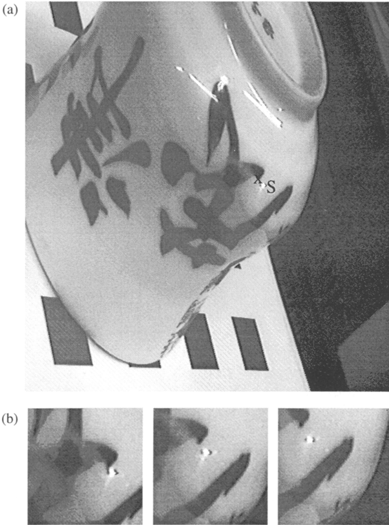
Figure 2.8: Motion parallax as a robust cue for surface curvature at a specularity.
