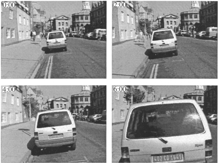
Figure 5.6: Using image divergence to estimate time to contact.
