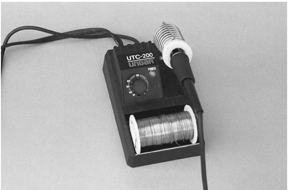
FIGURE 7-2 Use a low-wattage (25 to 30 W) soldering pencil for all electronics work.
