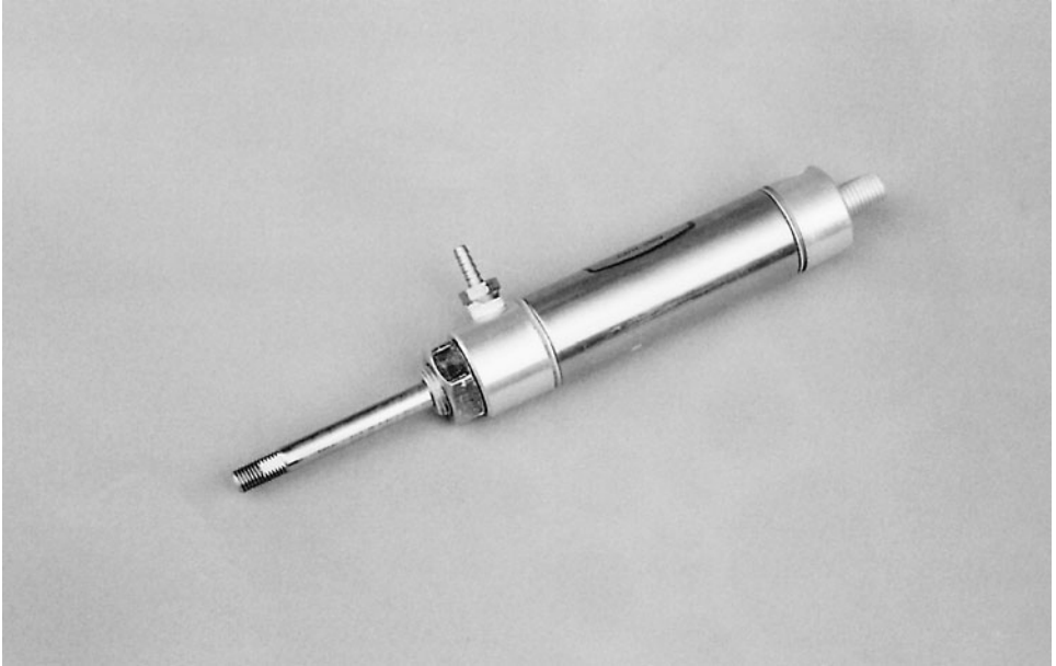
FIGURE 26-5 One of the many available sizes and styles of pneumatic cylinders. This one has a bore of about \frac{1}{2} in and a stroke of three in.
