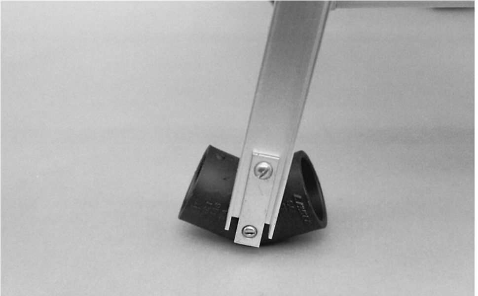
FIGURE 24-15 PVC plumbing fittings used as feet. The feet use a flat mending iron. Add pads or rubber to the bottom of the feet as desired.
