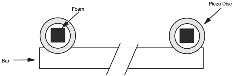
FIGURE 30-31 Glue the piezo discs to a piece of plastic; the plastic is a support bar for the discs that also makes it easier to mount the touch bar sensor onto your robot.
