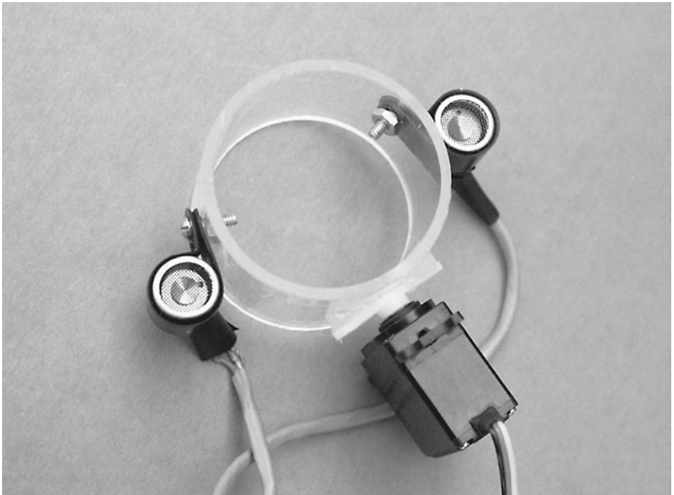
FIGURE 30-14 Ultrasonic sensors mounted on an RC servo scanner turret.
