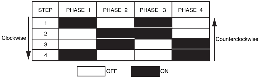
FIGURE 21-4 The enhanced on-on/off-off four-step sequence of a unipolar stepper motor.
