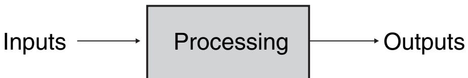
FIGURE 13-4 Typical beginner program flow. Input data is passed to a block of code for processing and then output. This program model cannot be used for robot programming.
