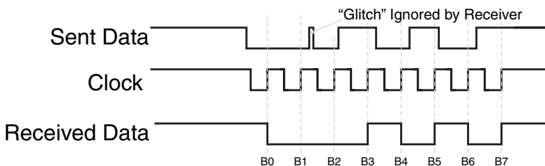
FIGURE 12-4 Close-up detail showing how synchronous serial data is only picked up on the clock edge.
