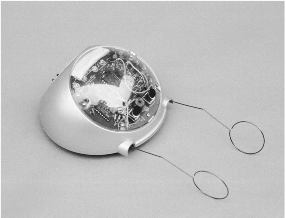
FIGURE 30-18 The Movit WAO robot (one of the older models, but the newer ones are similar). Its two tentacles, or whiskers, allow it to navigate a space.
