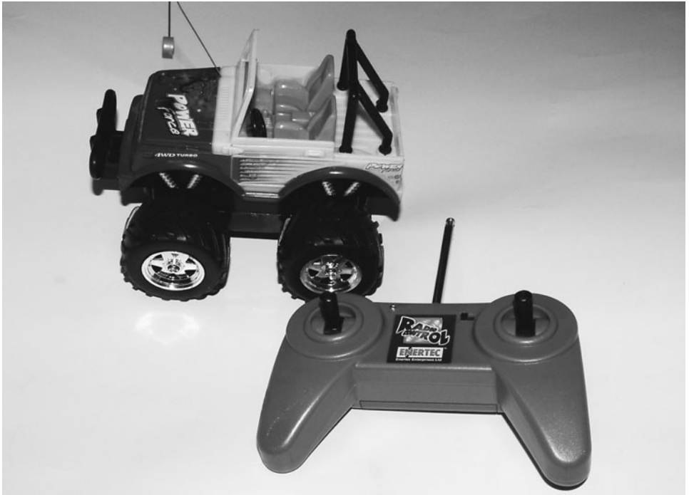
FIGURE 11-7 This remote control robot was purchased as a set of two for less than $10. The remote controls work at 27 and 49 MHz and the toys are powered by three AA alkaline batteries.
