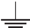
FIGURE 5-16 This symbol is used for the common negative voltage connection in an electronic circuit.
