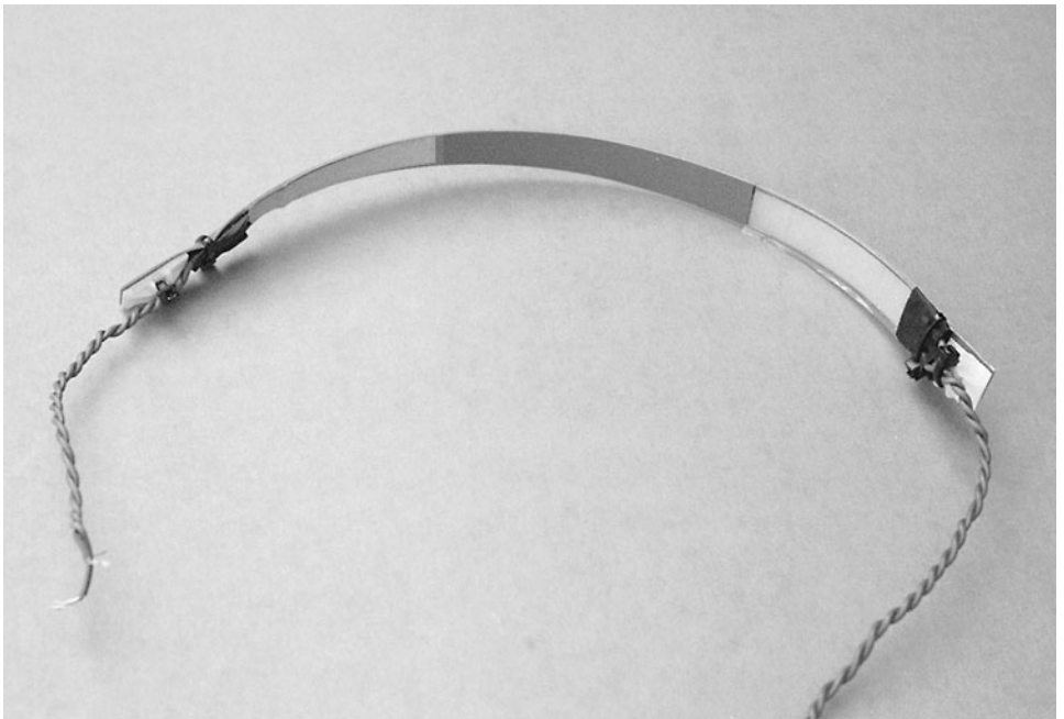
FIGURE 29-14 The prototype Kynar piezo bend sensor.
