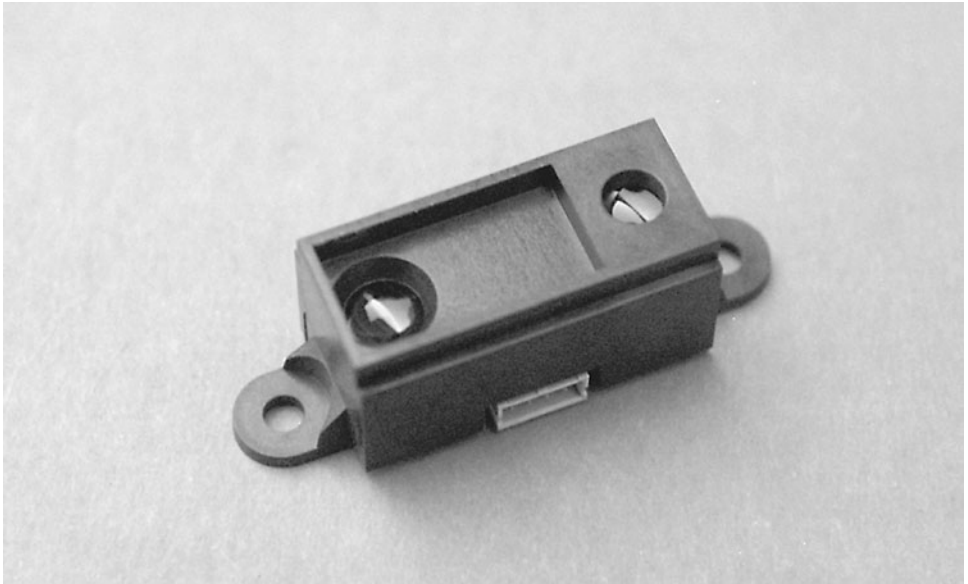
FIGURE 30-7 The Sharp infrared sensors work similarly to the BS2 proximity sensor presented earlier in the book.
