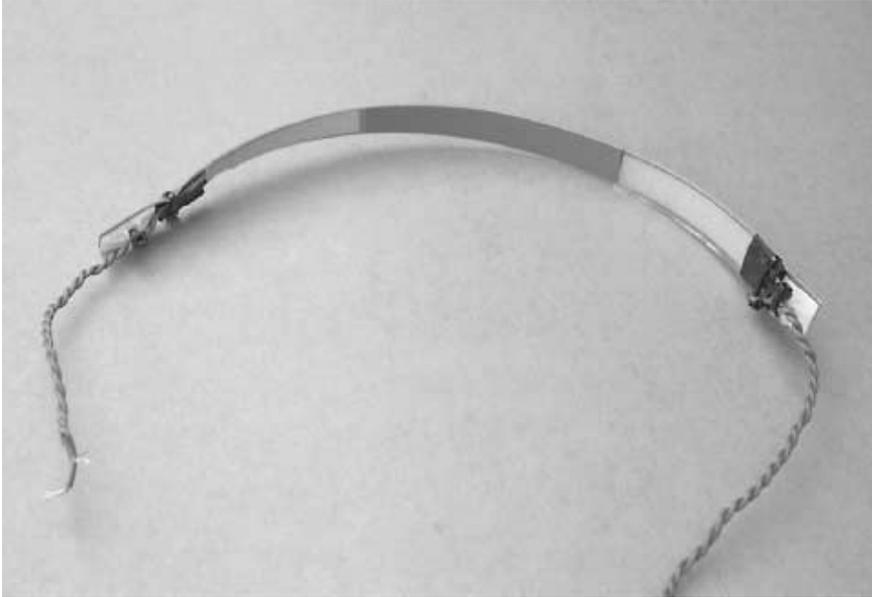
**FIGURE 35.11** The prototype Kynar piezo bend sensor.
