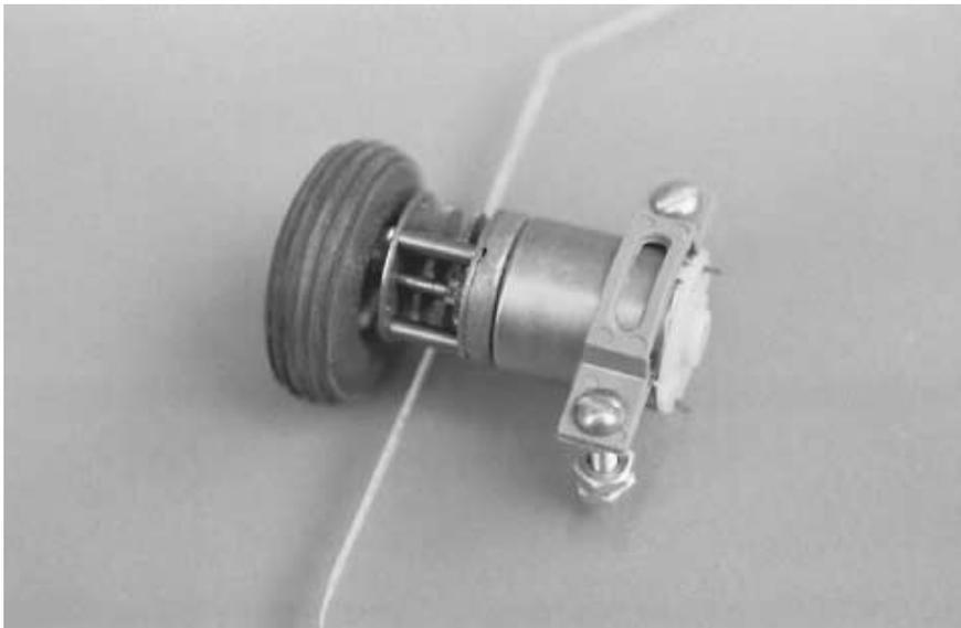
**FIGURE 8.3** How the drive motors of the Minibot look when mounted. In the prototype Minibot the wheels were threaded directly onto the motor shaft. Note the gear-reduction system built onto the hobby motor.
