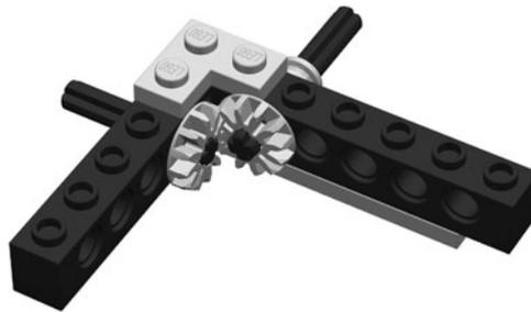
Fig. 9-18. Bevel gear.
