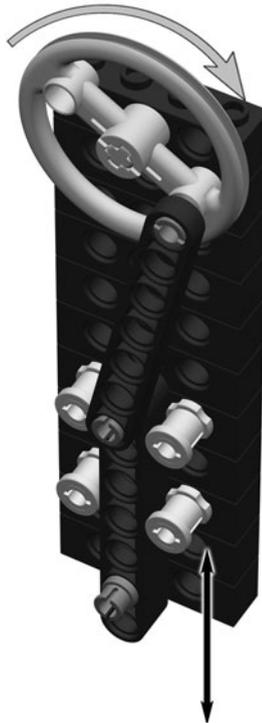
**Fig. 14-7.** Better rotary to reciprocal motion.
