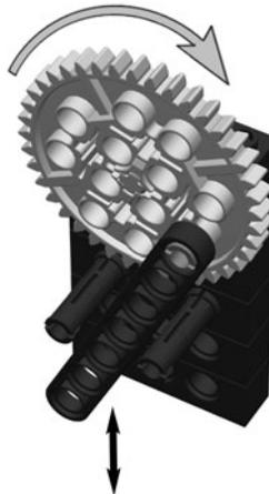
Fig. 14-3. Rotary to reciprocal motion.
