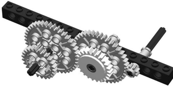
Fig. 9-23. Torque-limiting clutch.
