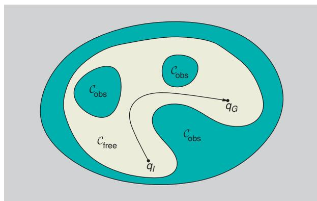
**Figure 4.** In the C-space, the problem looks simple: connect  $q_I$  to  $q_G$  while remaining in  $\mathcal{C}_{free}$ .
