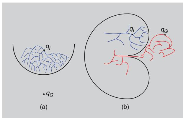
**Figure 14.** The C-space obstacles may contain wells that trap planners in local minima or one-way doors that resemble bug traps. (a) Filling a well. (b) A bug trap.
