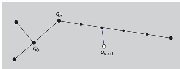
**Figure 12.** For ease of implementation, intermediate vertices can be inserted to avoid checking for the closest points along line segments. The tradeoff is that the number of vertices is increased dramatically.
