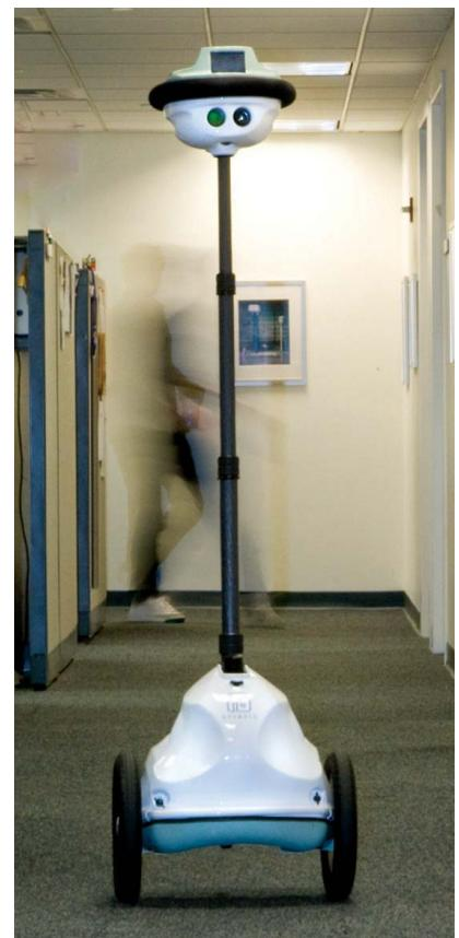
**Figure 3.** Anybot commercial telepresence robot (2010).
