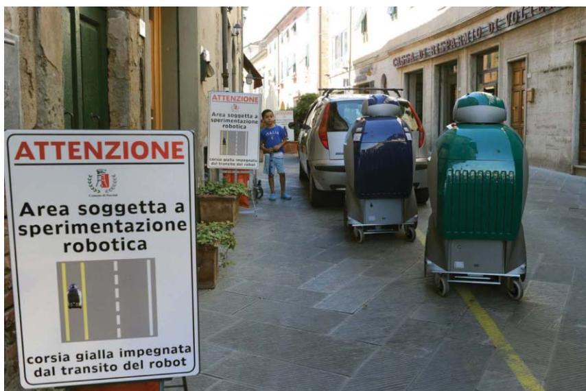
**Figure 7.** Example of a new road sign (C type), which was specifically designed for the testing of DustCart in Peccioli, Italy. (Photo courtesy of Foto Silvi.)
