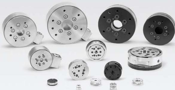
**Standard Features:** Six Axes of Force/Torque Sensing (Fx Fy Fz Tx Ty Tz) • High Overload Protection • Interfaces for Ethernet, PCI, USB, EtherNet/IP, CAN, and more • Sizes from 17 mm - 250 mm diameter • Custom sensors available
