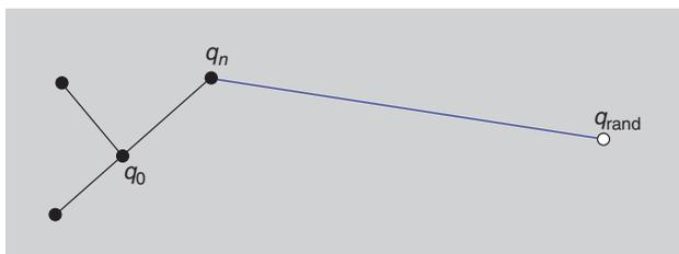
**Figure 10.** A new edge is added that connects from the random sample  $q_{rand}$  to the nearest point in  $S$ , which is the vertex  $q_n$ .
