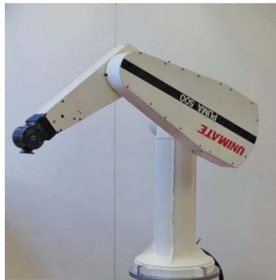
**Figure 18.** The classic Puma 560 arm is a chain of three rotatable bodies (excluding the end effector) attached to a rigid base. This yields a three-dimensional  $\mathcal{C}$ -space, which is handled by the standard planning algorithms. (Photo courtesy of the Technical University of Berlin.)
