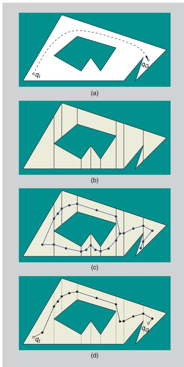
**Figure 5.** A combinatorial planning illustration: a) 2-D polygonal obstacle region with proposed  $q_I$  and  $q_G$  (one possible solution is shown in a dashed path); b) the trapezoidal decomposition; c) constructing a graph by placing a vertex in every vertical edge segment and every trapezoid interior; and d) connecting  $q_I$  and  $q_G$  to the graph and searching for a solution path.
