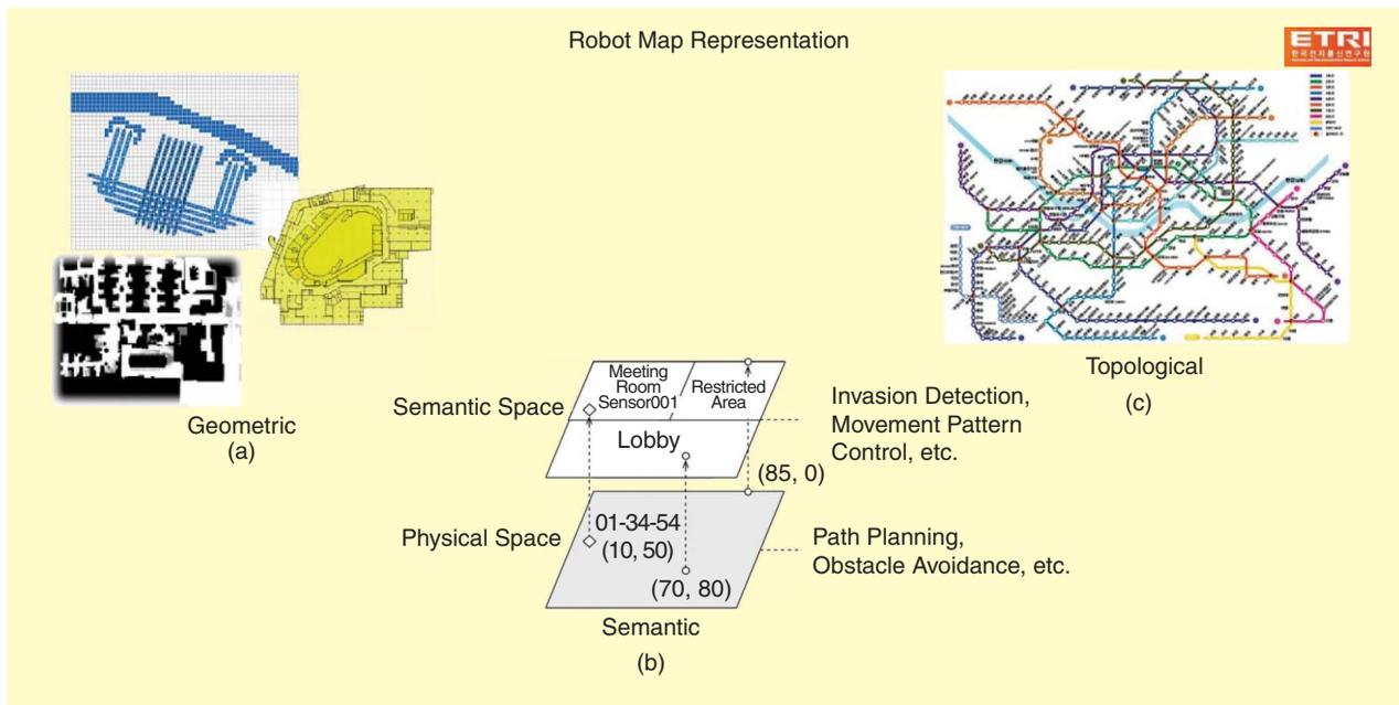
(a) Some examples of metric map, (b) conceptual illustration of semantic mapping between physical space and the corresponding semantic description, and (c) (pure) topological map (subway lines of Seoul).
