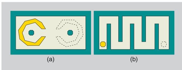
**Figure 11.** Rotation versus translation domination: (a) The task is to move the C shape to the right. Rotation dominates. Performance should improve if rotation is weighted heavily in the metric. (b) In this case, the translation dominates and should therefore be weighted more heavily if this fact is known in advance.
