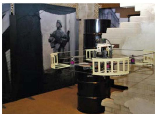
**Figure 3.** Pelican navigates autonomously over and under obstacles. (Photo courtesy of SEAS, University of Pennsylvania.)
