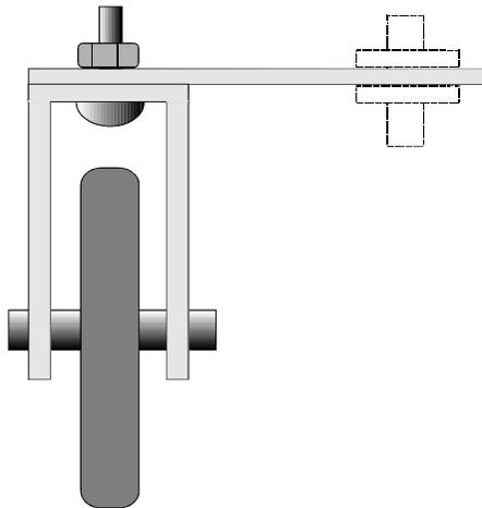
An alternative design for a castor has a single wheel. The mounting could be made from strip aluminium or brass about 10 mm wide.
