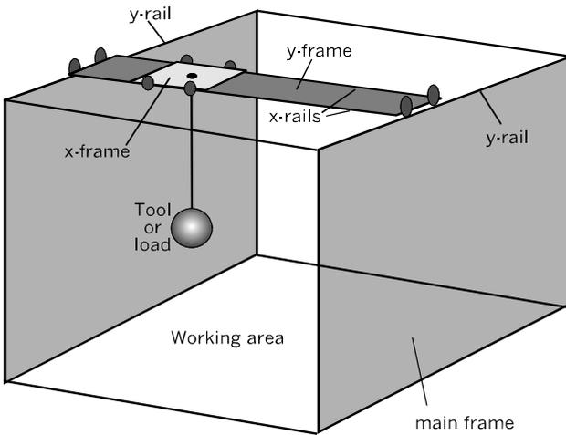
The architecture of a typical gantry robot.
