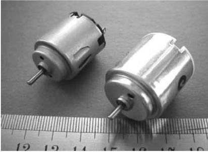
A pair of very inexpensive motors running on 1.5 V to 4.5 V. They produce 8 gf cm and 18 gf cm respectively. These motors have no gearbox.
