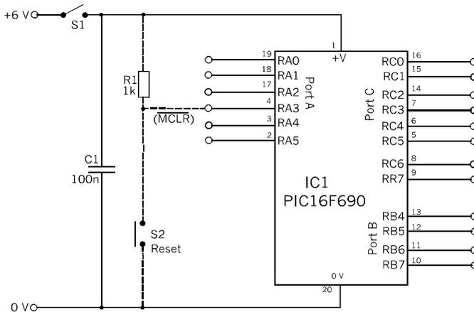
With its 20-pin package the 690 provides up to 18 I/O pins.
