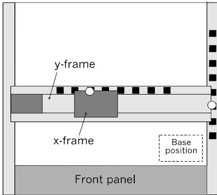
(Left). Using markers to track the location of the x-frame and thus the x- and y- position of the tool.
