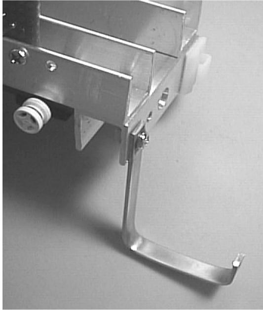
The finger attached to the x-frame reaches down beneath the right side-rail of the main frame. Its upturned end presses against the actuator lever of MS2 when the y-frame is at the front and the x-frame is at the right. Determine the dimensions of the finger by measurement when the x-frame is in position.
