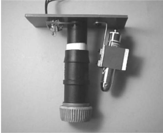
For many scanning applications the camera and laser are mounted on the same base plate.
