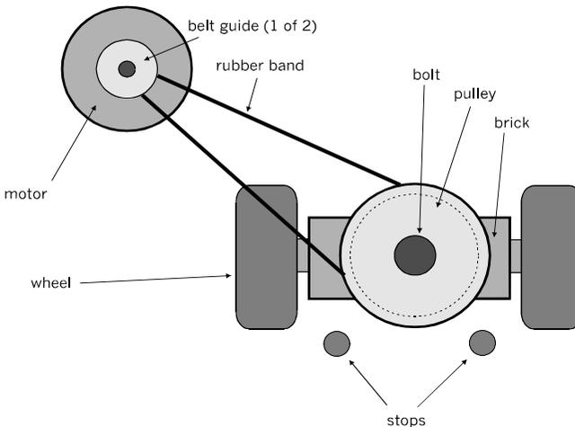
**Looking down on the steering mechanism, we can see the upper end of the castor bolt projecting upward. At its upper end a 25 mm pulley is gripped between two nuts and a third nut is tightened against the upper one of these as a lock-nut.**
