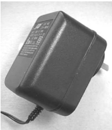
This plug-top PSU (with Australian plug) produces a DC output switchable to 3 V, 4.5 V, 6 V, 7.5 V, 9 V and 12 V. The maximum current is 1 A.
