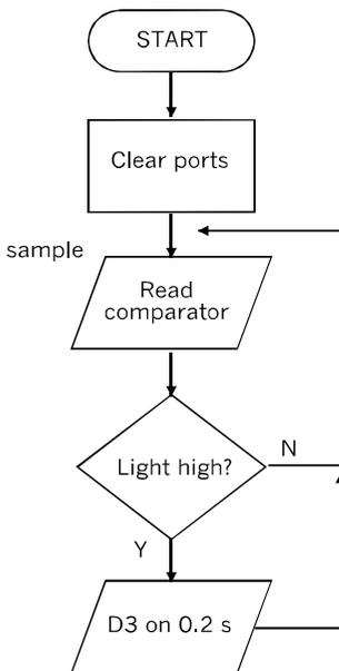
The flow chart shows that the program runs in a continuous loop. Each time around the loop the output of the comparator is read, and the LED is switched on for 0.2 s or not, depending on the reading.
