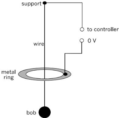
When the switch is tilted the wire of the pendulum touches the metal ring. This completes the circuit and the input channel of the controller is pulled down to 0 V.
