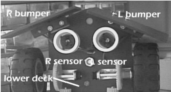
Underneath view of the robot, showing the two IR sensors. The circuit boards can be seen surrounded by the white plastic shields.
