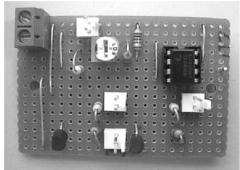
The light sensor occupies the upper half of the board, with the pair of LED switches on the lower half.
