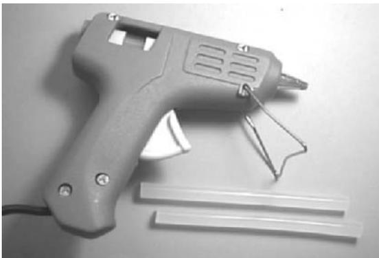
The glue sticks are melted by the electric heating coil in the gun. Press the trigger to extrude molten glue from the nozzle.
