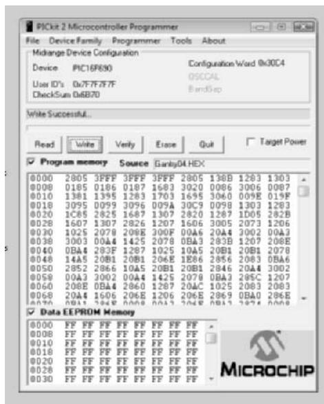
The PICkit 2 has just downloaded the source file *Gantry04.hex* into a PIC16F690. The window shows the hex code.
