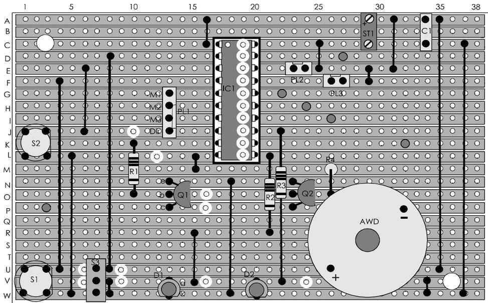
Stripboard layout of the PIC1 board. Cut strips between E23/E24 and F26/F27.
