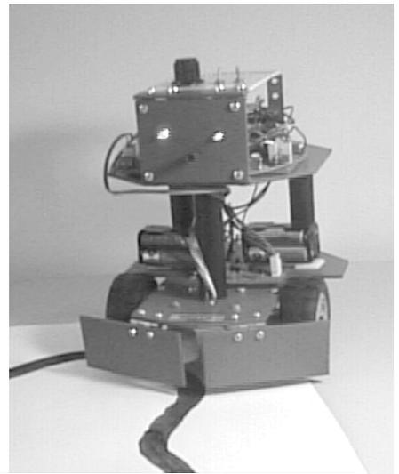
Too many wires visible? This is a research robot so wires are inevitable. Some people like to see the 'works' but, if you prefer a sleeker look, make a 'skin'. Use PVC sheet, foam board or thick cardboard. The skin drops over the *Quester*, to hide the circuit boards, batteries and wiring,
