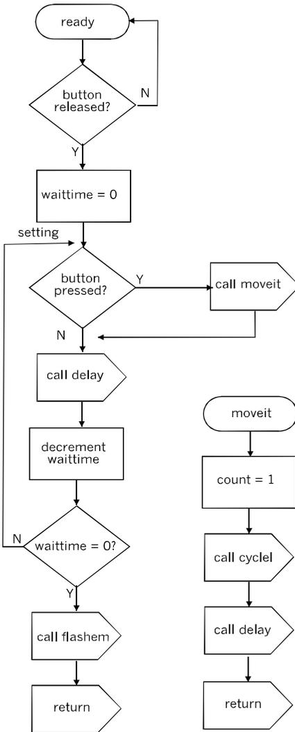
The *ready* and *moveit* subroutines, which prepare the robot for playing.
