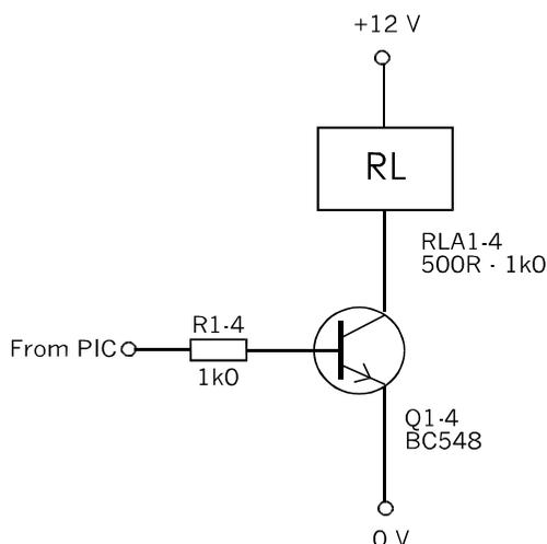
The four relays are operated by four transistor switches like the one shown in this figure. The lowest working voltage of commonly available relays is 12 V (but see above). This circuit allows the relay to be switched by a PIC operating at a lower voltage, such as 4.8 V.
