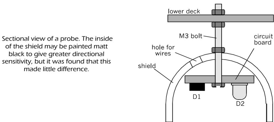
The sensors are tested by using a piece of white card, half of which is painted black. Connect the 6 V power supply and plug in one of the probes. Connect a voltmeter to the output pin. Adjust the preset resistor until the output voltage is low (close to 0 V) when the white area of the card is held 20 mm from the sensor, but rises close to the positive supply voltage when the black area is held there.
