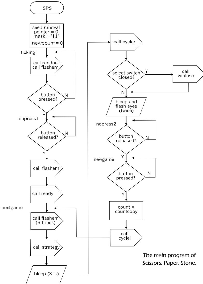
The value in *newcount* may be one that has resulted in a win for the robot. It is repeating its successful play. However, if the robot lost the previous game, *newcount* is usually (but not always) given a different value in the *tryagain* routine (the last routine in the listing, p. 245). It will try a different response in the current game.
