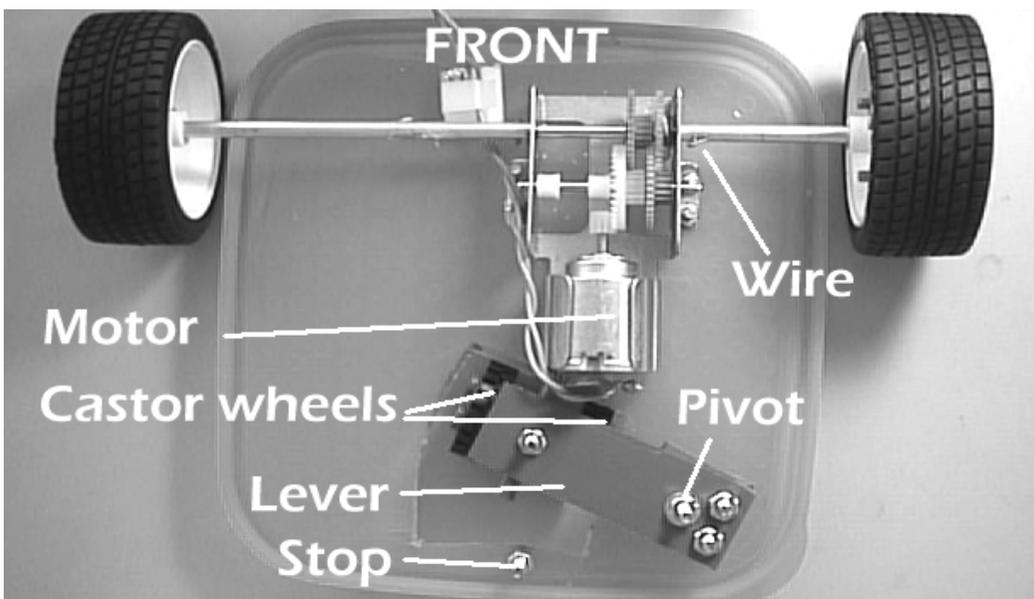
A top (inside) view of the wheel assembly on the lid. The castor wheels are mounted inside the lid but project through a fan-shaped aperture.
