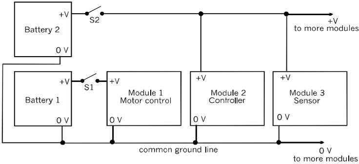
Power distribution circuit. The switches S1 and S2 are on the Control Panel.
