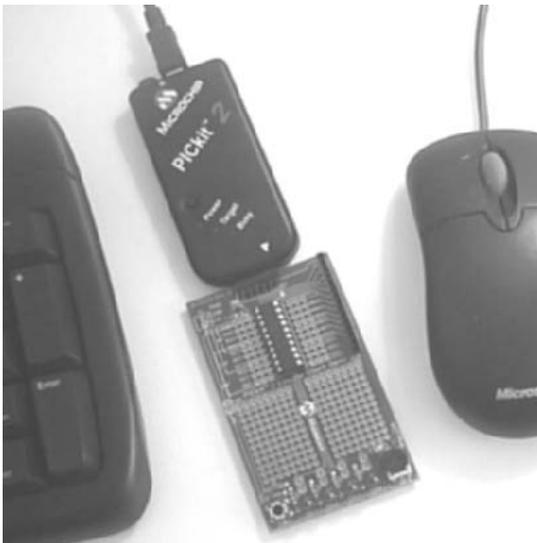
The PICKit 2 comes with a USB connector. It is a small neat unit that sits comfortably on the computer bench as you program it and watch it perform. It connects directly to a small board that carries the PIC while it is being programmed. The board has a switch and some LEDs for testing input and output routines. There is space for you to build a few interfaces to the PIC.
