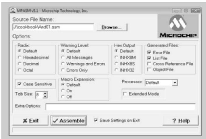
The MPASMWIN window lets you set various parameters for generating the machine code file (also known as the hex file). While assembling, it checks for errors and reports these and possibly some warnings. If there are errors they are reported in an error file (extension *.err*) which you can view by loading it into *Notepad*.
