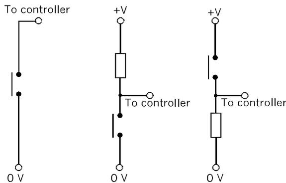
One-bit input circuits. *Left:* for use when the channel has weak pull-ups. Input normally reads as high, but goes low when the button is pressed. *Centre:* for use on channels without weak pull-ups. A 10 kΩ resistor is suitable. Input is normally high. *Right:* The same as the previous circuit except that input is normally low.
