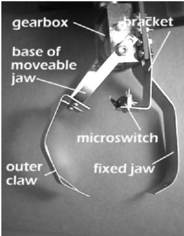
The microswitch on its bracket. The jaw base is secured to the lever by a bolt and a hole for the output shaft.
