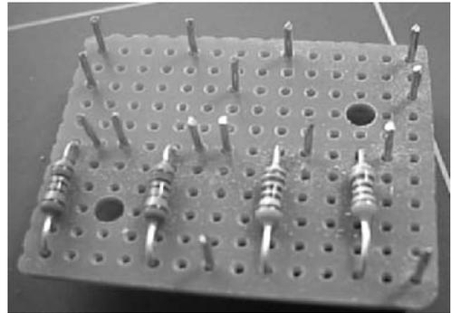
Most of the wiring of the control panel is between the components themselves, already mounted on the panel. There is a small stripboard (above) which connects the on-panel components to the outside modules using PCB pins. This board is mounted on the back of the control panel.
