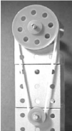
Pulleys transfer power over a distance. If the wheels are of different sizes, they turn at different speeds. The diameters of the races of these wheels are 36 mm and 12 mm.
