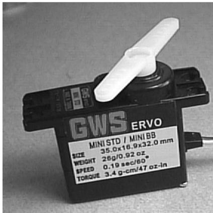
A small servomotor of the kind used in flying model aircraft and robots. The 'horns' (white levers) are used for connecting the motor to the mechanisms that it drives.
