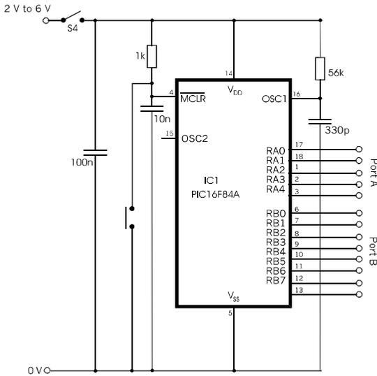
(Left) The 16F84A needs an external oscillator, provided here by a resistor/capacitor network.
