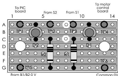
D1 and D2 are mounted on the reverse side of the board
