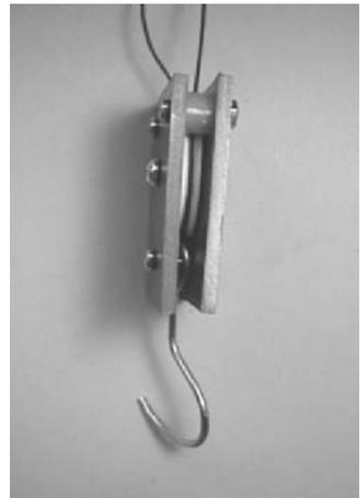
A special mechanism raises and lowers the hook. The same mechanism is used to raise and lower the gripper. The principle of this is illustrated below. The winch motor M3 is at the left end of the y-frame. From the winch the cord runs *under* the x-frame and is tied to the right end of the y-frame.
