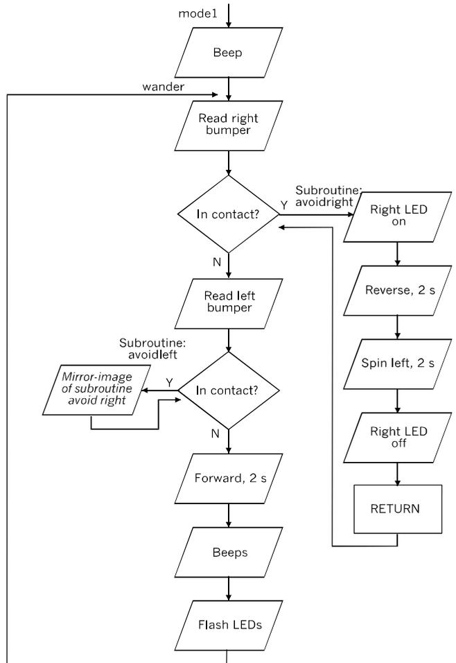
If nothing is detected, the robot runs forward for about 2 s, then stops, beeps and flashes its LEDs before returning to the beginning of the loop.
