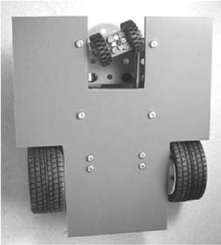
A view of the chassis from below shows how the wheels are within its rectangular area. This is so that the wheels will not be easily visible when the *Android* body is in place.
