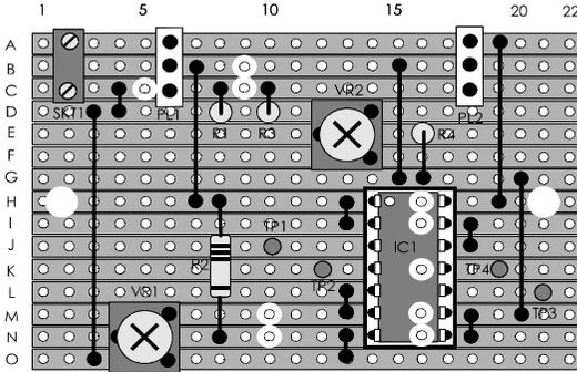
The IR sensor board interfaces the two sensors to the system. The board has two header plugs: PL1 connects to the left sensor and PL2 to the right. Connections are: strip A, +6 V; strip B, output from photodiode cathode; strip C, from IR LED anode. Output is normally taken from the board at TP1 (left) and TP3 (right).
