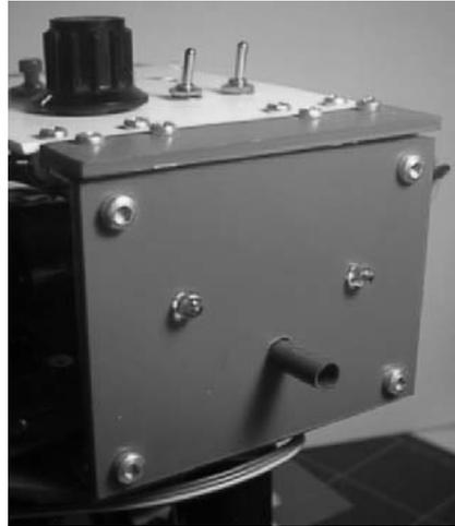
Note the strip of PVC bolted on top of the hinges. This is for neatness, to cover the gap between the front edge of the control panel and the upper edge of the front panel.
