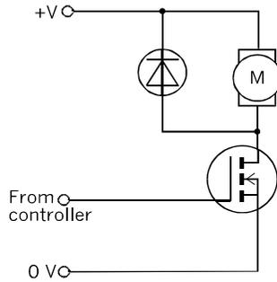
An npn BJT can be substituted for the MOSFET.
