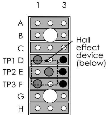
Two sensor probes are required and these are mounted at one end of the y-frame and on one side of the x-frame. To mount the probes, first solder each to a very small rectangle of stripboard (right).
