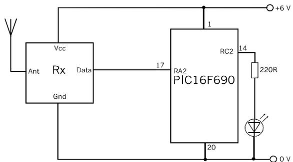
The modules require only a few milliamps. In the diagrams the PIC is run on the same supply as the transmitter or receiver. Because the transmitter operates on a lower voltage, the 6 V supply to the PIC is tapped to give 3 V for the transmitter, when the system is running both modules. Output from the PIC is fed to the transmitter through a potential divider.
