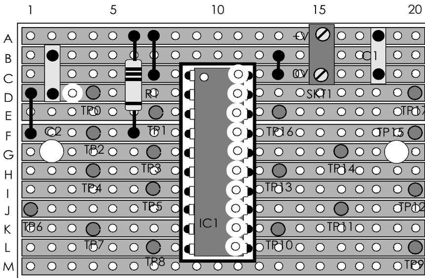
Layout of the controller board. Check the underneath of the board, using a hand lens to make sure that all the copper strips are cut beneath the PIC.
