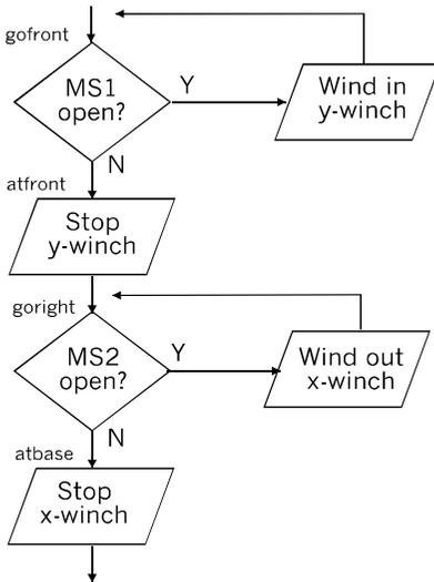
First move the y-frame toward the front until MS1 closes, then move the x-frame to the right until MS2 closes. Finally (and optionally), switch on the green LED to indicate that the x-frame is at base.
