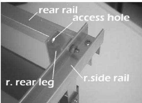
(Left). Close-up to show the right rear leg bolted to the right side rails and the rear rail (bolt not visible) for this rail. Note the screwdriver access hole.
