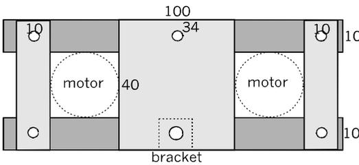
The rear ends of the motors are supported by a framework.
