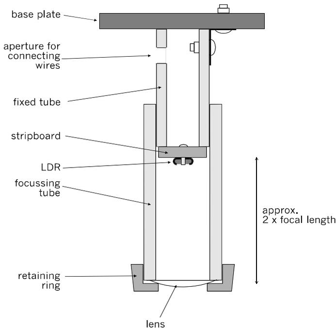
The camera, directed downward to focus an image of an object in the *Gantry's* working area.
