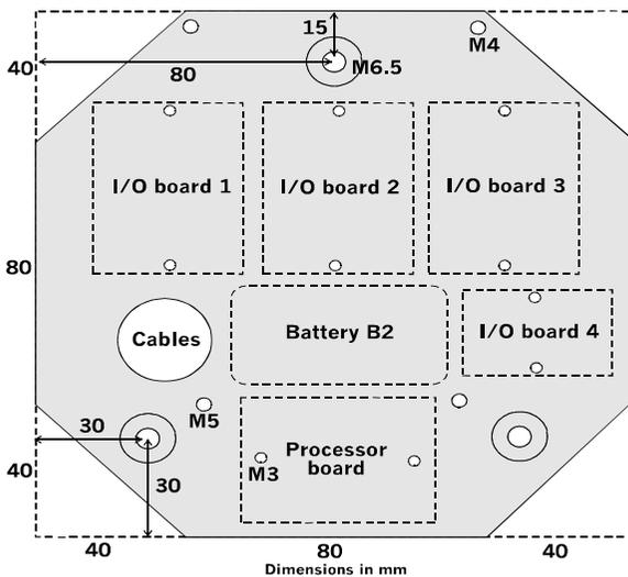
The upper deck, showing the layout of the circuit boards and the positions of the three spacers.
