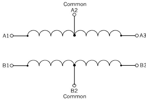
The two windings of the stepper motor are tapped at their centres.
