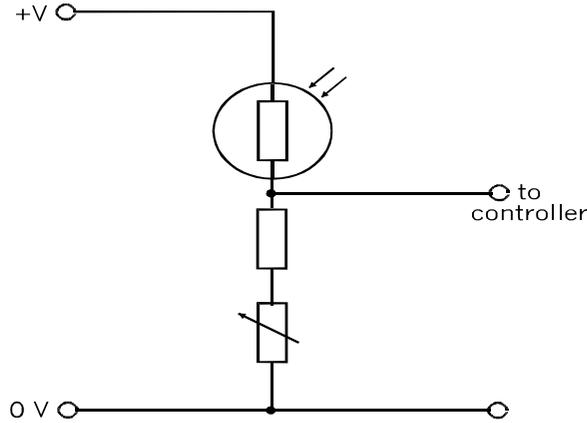
As light increases the resistance of the LDR decreases and the voltage sent to the controller rises.
