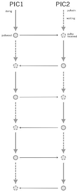
Programming two PICs to operate alternately. A PIC sends a pulse to the other when it has completed its current task. Then it waits (dashed lines) to receive a pulse before resuming its activities.
