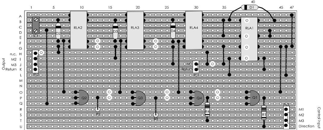
Layout of the motor control board. Strip A runs the full length of the board, with no cuts. Strip B is cut only at B39. The 12 V or 9.6 V power supply goes to the screw terminal block at B2 (+) and D2 (0 V)
