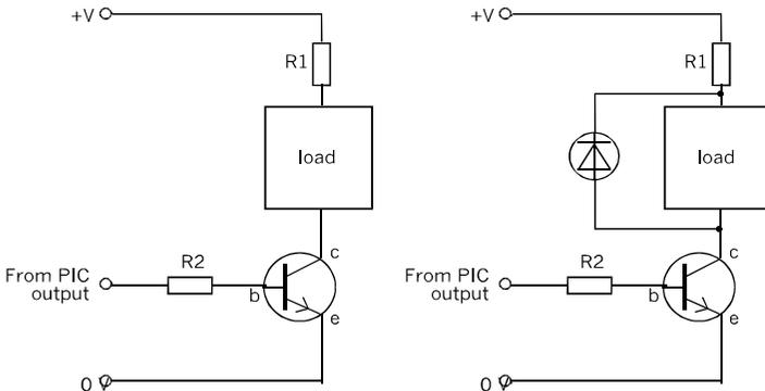
BJT switches for (left) non-inductive and (right) inductive loads. The current limiting resistor, R1, may not be necessary. The load is switched on when the input from the PIC goes high.
