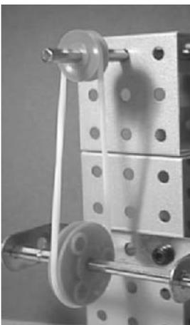
Shafts can be at right angles and at any other smaller angle. There is a risk of the belt coming off if the shafts are too close together.
