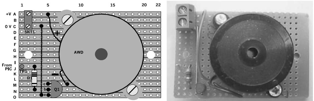
The Beeper board. For maximum loudness, make sure that the AWD is fixed firmly to the circuit board and the board is fixed firmly to the deck.
