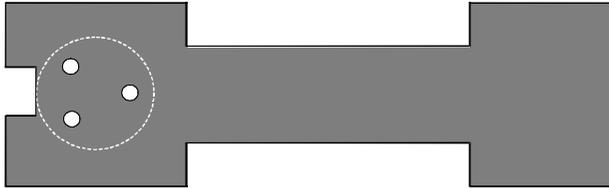
An arm is cut from a rectangle of Foam Board about 130 mm by 40 mm. The movable arm has three holes in the 'shoulder' for bolting on the pulley wheels that attach the arm to the shaft.
