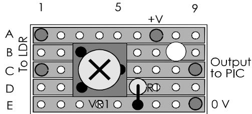
Stripboard layout of the camera board, VR1 is adjusted to suit the range of ambient light intensity.
