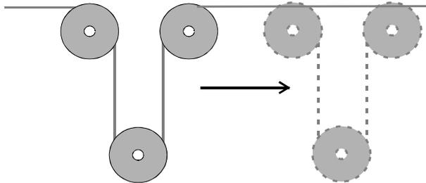
The travelling pulley mechanism. The upper two pulleys are mounted in a box on the x-frame. The lower pulley is in the pulley block that carries the hook. As the frame moves from left to right the height of the hook above ground is unchanged.
