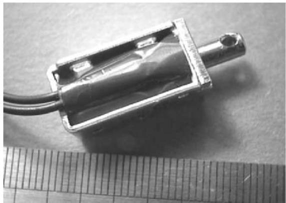
The main applications of solenoids are short-stroke actions, such as releasing catch mechanisms. An electric door latch is operated by a solenoid. They are also built in to operate electrically controlled valves.
