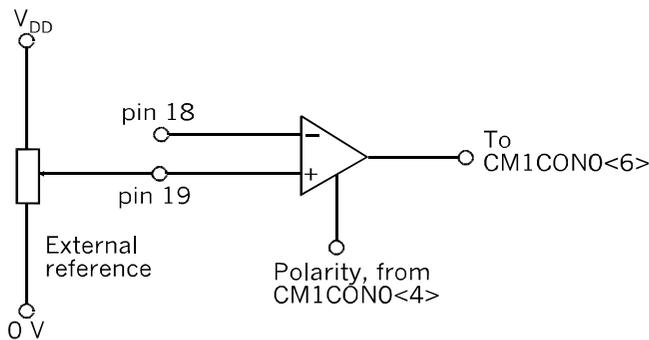
A PIC comparator visualised as a schematic. If the polarity bit is 0 (non-inverted polarity), the output is high when the input at pin 18 is less than the reference voltage.
