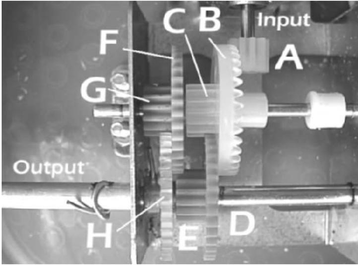
The motor turns the input shaft which has a pinion A meshing with a crown B. A small gear wheel C is moulded on to B so they turn as one. C engages with a larger wheel D, which has a pinion E moulded on it. D/E is a loose fit on the shaft. E meshes with a larger wheel F which has a pinion G moulded on it. G/H is loose. G meshes with a larger wheel H and this is a tight fit on the output shaft.
