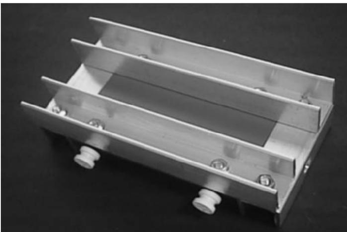
The x-frame consists of four lengths of channelling bolted together. The structure is held 'square' by the PVC panel bolted across the long members. The same bolts are used to secure the wheel base-plates.
