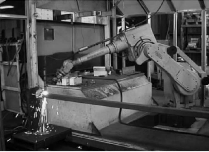
This robot has welding gear at the end of its arm. The arm is bolted to the floor but the welding torch can be manipulated so as to act at almost any location in the workshop. Other tools can be fitted to it when required.
