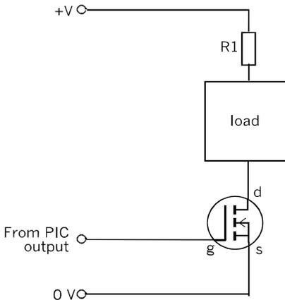
A transistor switch based on an n-channel MOSFET. The current-limiting resistor may not be required. A protective diode is necessary if the load is inductive,
