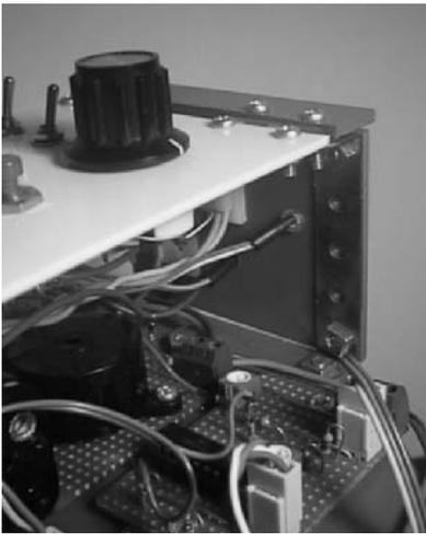
(Above) Three-quarters rear view of the upper deck and control panel (white). The control panel is supported at the front by being hinged to a framework of metal strip. In the foreground are the boards for the bumpers and IR sensors.
