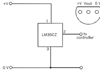
The bandgap temperature sensor needs no external components.
