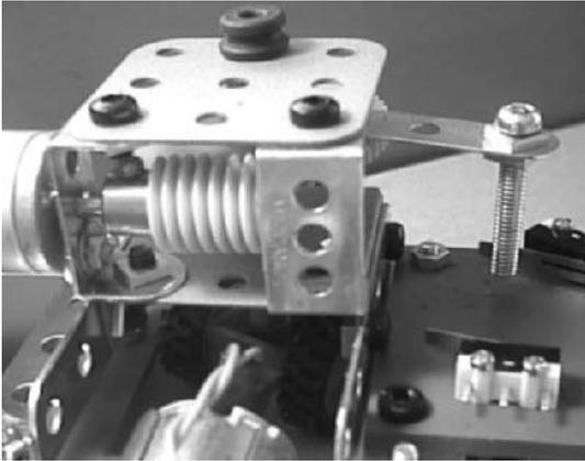
A lever is bolted to the gear wheel. The lever has a long bolt projecting downward to engage with the levers of the limit switches. These are mounted on a small platform of PVC sheet bolted to the frame of the steering mechanism. This photo was taken before the switches were wired up.
