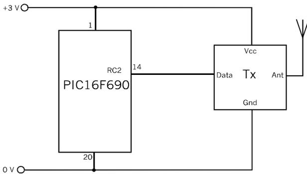
A digital signal from the PIC is sent directly to the Data terminal of the transmitter module. The drawing shows an antenna connected to the 'Ant' terminal but the module has been found to work well without an antenna for distances of several metres.
