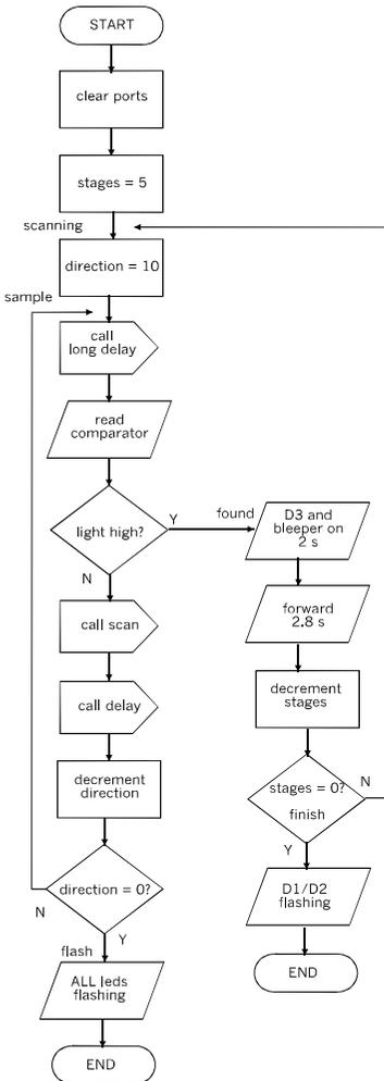
The *Scooter* first tries to find the light source, using the routine beginning at the label 'sample'. It reads the comparator output to determine if the light ahead of it is bright or not bright. By 'bright' we mean that the voltage from the LDR sensor is greater than the reference voltage.
