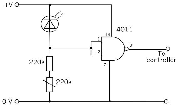
One-bit input from a photodiode (visible light or infrared).
