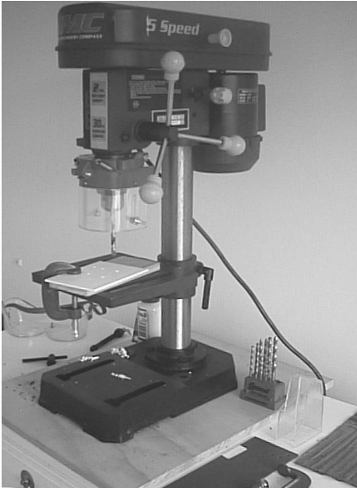
A drill press helps put the holes in the right places and at right angles. Use it for aluminium, brass, wood or plastic, preferably running it at its lowest speed.
