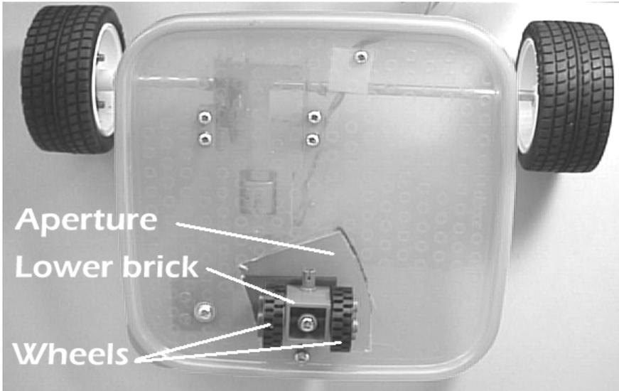
The Scooter's wheel assembly is on the lid, seen here from below (the outer side). It runs on three wheels, in effect, but the rear castor wheel actually is a pair of wheels. The castor is pivoted at a point to one side of the fore-aft centre line. In this photo the castor is in the position it takes up when the robot is running straight ahead.
