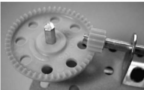
A crown and pinion gear is a reduction gear with the shafts at right angles. The smaller gear, the pinion, has ten teeth. The crown has 50 teeth. The ratio is 1:5, so the smaller wheel turns five times faster than the large wheel.
