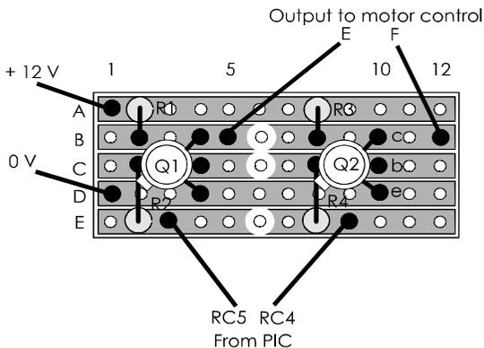
On the interface board, the connecting wires are soldered directly into the holes. Their other ends are stripped for inserting into the sockets on the controller and motor control boards. The power supply is taken from spare sockets on these boards.
