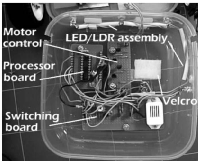
The interior of the box when wiring is finished, as seen from below. Most of the connections are between the Processor board and Switching board, but the wiring has been routed away from the processor socket so that it does not interfere with putting the PIC into its socket and removing it. The connections to the LED/LDR assembly can be seen going off to the left (right in the photo), near the label 'Velcro'. The main switch S1 can just be picked out between the Velcro and the buzzer.
