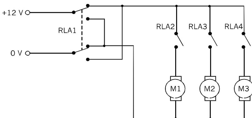
The circuit for controlling the winch motors. The motors are connected to three SPST relays, but share a common line to return the current to the DPDT reversing switch. The relays are rated to operate on 12 V, but those used in the prototype work just as well on 9.6 V from four NiMH cells.
