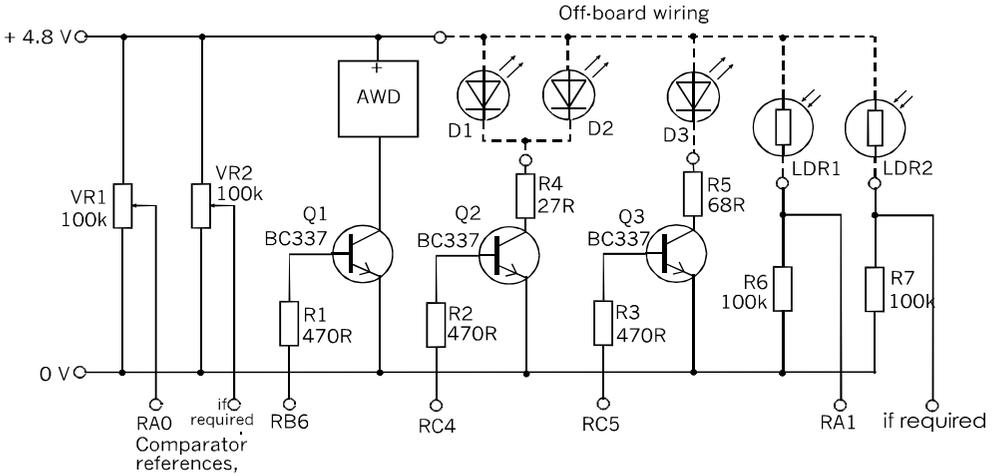
As well as transistor switches for the LEDs and buzzer (AWD), the switching board has the resistors of the two light sensor circuits. It also has two optional voltage dividers for use with comparator circuits.
