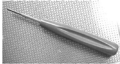
While on the subject of cutting the strips, **ALWAYS** examine each cut with a string magnifier. It is too easy to leave a microscopically thin hair of wire around the edge of the cut. It is surprising how much current can flow through such an invisible thread. Make this the first fault to look for (with that magnifier!) when a circuit fails to work.
