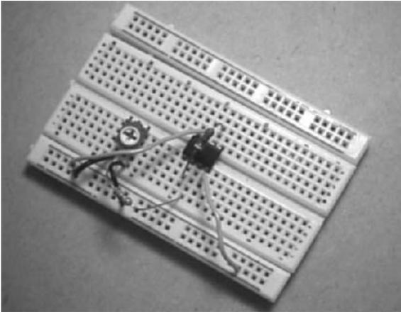
Breadboarding is usually the first practical step when designing a circuit.
