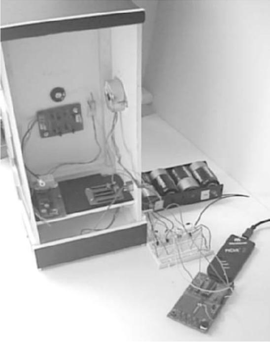
Before wiring up the board, the programming of the stepper motor of the arm was developed and tested. The motor is on the right-hand wall, with wires leading to the prototype motor control board (still breadboarded at this stage). The breadboard receives input from the PIC, which is on the PICkit 2 development board.
