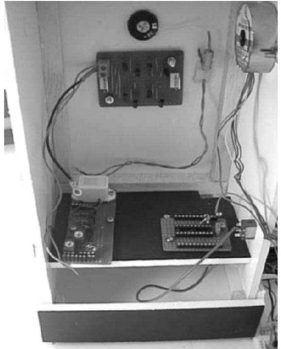
With all the essential circuit modules, except for one, taken ready-made from other robots there would seem to be little to do but join them together. But first there may be a problem to be attended to. The steering motor H-bridge does not provide a full 6 V supply so the motor may run too slowly or not at all. An interfacing circuit may be needed. The interface board and the steering motor are then supplied with a higher voltage (say, 9 V). which needs a separate power switch.
