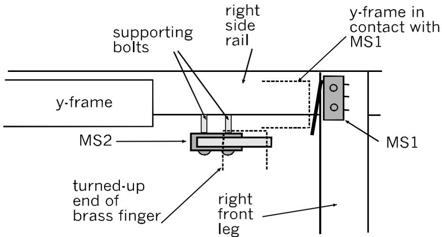
Both MS1 and MS2 are closed when the x-frame is at the front right corner of the main frame.
