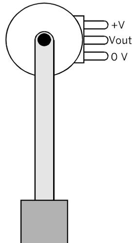
The voltage output from a tilt sensor varies with the amount of tilt.
