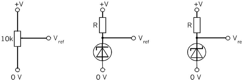
Voltage references: Left: variable output from a potentiometer is proportional to the supply voltage. Centre: Zener diode, gives stable voltage with varying supply. Right: Band-gap reference gives highest precision.
