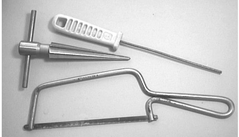
A **reamer** can enlarge circular holes up to 18 mm in diameter. It is not an essential tool, but does the job neatly. While on the subject of cutting large holes, consider getting a circular **hole-saw** that attaches to an electric drill. It is supplied with a range of interchangeable blades in diameters from 25 mm to 53 mm. Again, this is not an essential tool, but is the best way of cutting large holes quickly.
