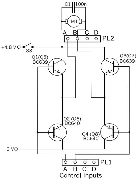
The circuit that controls the twin drive motors in the *Quester* robot. This diagram shows only the circuit for the left motor. The figures in brackets refer to the circuit for the right motor.
