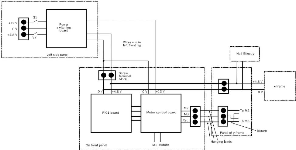
Power connections. Also shown are the control lines from the PIC1 board to the motor control board, and the output lines from there to the motors. The return line is common to all three motors.
