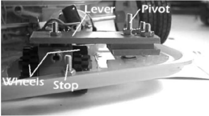
Before drilling the hole for the pivot, two small squares of plastic board are bolted to the lever, using two shorter bolts. Then the pivot hole is drilled through all three layers. The forward stop peg is seen in this photo.
