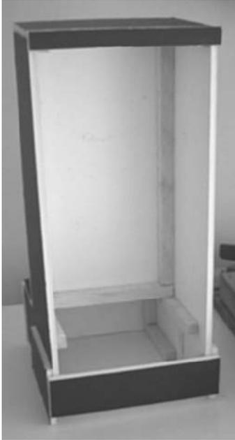
This is the body from the rear, showing the balsa strips glued in the angles. The two strips low down on the sides are to support the shelf that carries the battery and the main circuit boards. To allow easy access for checking, the shelf is not glued to these supports.
