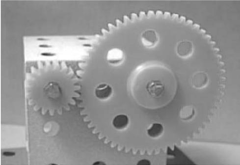
The small wheel has ten teeth and the larger wheel has 57. The ratio is 5.7:1, so the larger wheel rotated at about one sixth of the speed of the smaller one. Torque is increased about 6 times.
