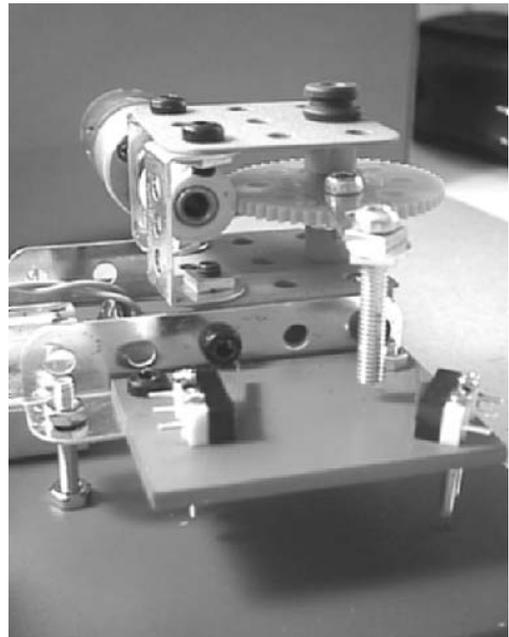
While assembling the chassis look ahead to the next stage to work out how the body is to fit on to and be supported by the chassis. The drive and steering mechanisms will be housed in the 'feet' of the body. There must be room for them to operate without touching against the inside of the body. Also it must be possible to remove the body to make alterations and adjustments to these mechanisms.
