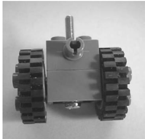
The wheel assembly is bolted to the lever, which is cut from metal strip or sheet plastic. The wheels are at right-angles to the length of the lever. At the other end the lever pivots on a bolt (see photo overleaf). The length of the bolt and the position of the lever on the bolt are adjusted so that the lid is level when resting on the drive and castor wheels.
