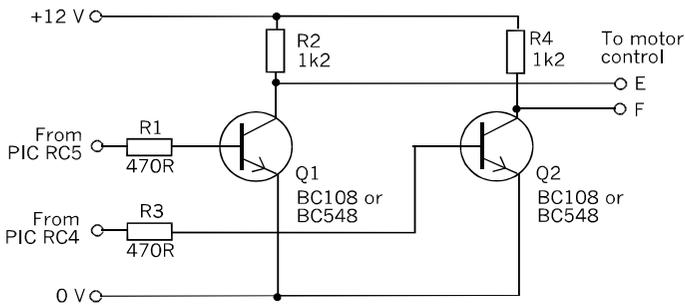
The interfacing circuit comprises two transistor switches. Almost any type will do. In the prototype they are a couple of BC108 transistors that have been unused in the spares box for a few years, but the more recent BC548 is equally suitable.
