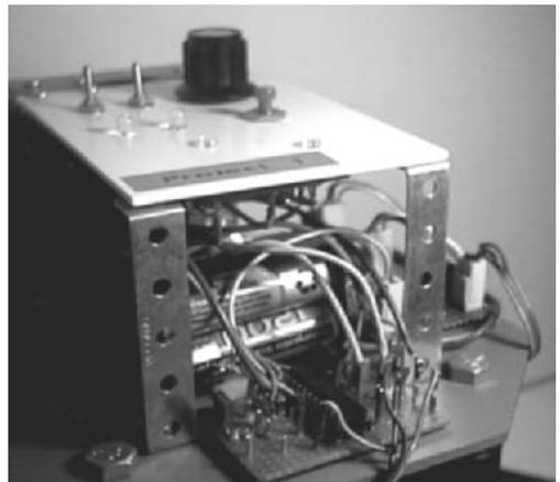
The figure shows one of the two vertical supports bolted to the upper deck. These are Meccano pieces. The control panel is hinged to a PVC cross-member joining the upper ends of the supports. At the rear, the control panel rests on another pair of supports, as seen in the photo opposite.
