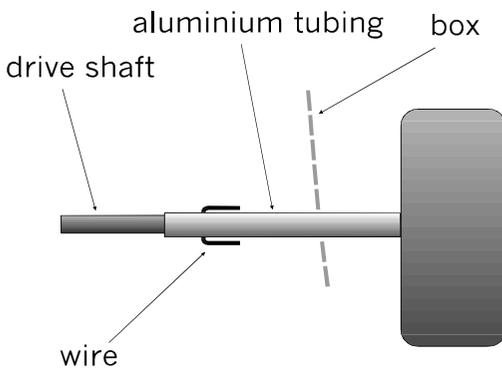
Coupling one of the drive wheels to the output drive shaft of the gearbox. The wire, threaded through a hole bored in the drive shaft and tubing, eliminates slipping. (Not to scale)
