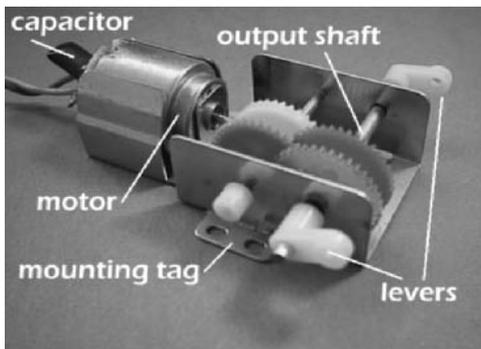
The jaw motor from CIC. The movable jaws are bolted to the two levers at each end of the output shaft. This shaft projects a few millimetres beyond the levers, fitting into one of the two holes in the base section of each movable jaw (see overleaf).
