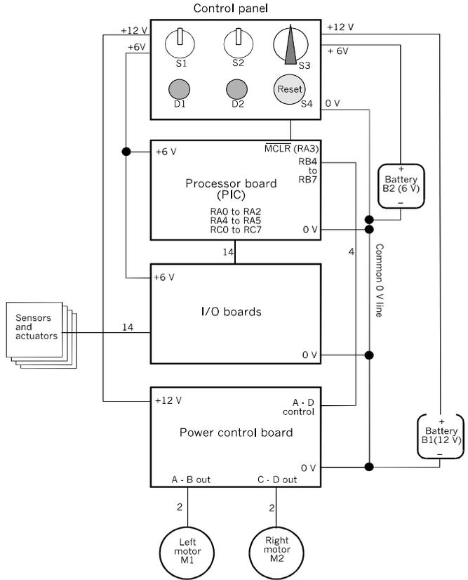
A block diagram of the whole electronic system of the *Quester*.
