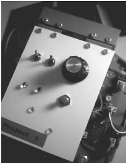
The completed control panel. You may prefer to label the switches and LEDs.
