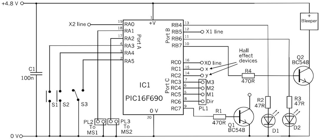
Schematic of the PIC1 controller board.
