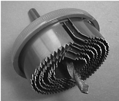
The saw blades cut holes of a range of sizes, centred on the hole first drilled by the bit.
