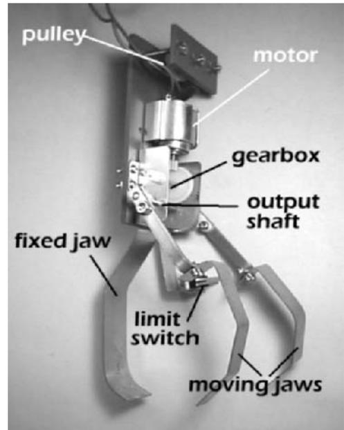
The motor unit is compact, measuring about 40 × 64 × 20 mm. It has holes for bolting it to the PVC panel, and a clip to hold the motor. The gears are plastic and a tight fit on the shafts. There are two drive levers that are pushed on to the opposite ends of the output shaft. The motor unit is bolted to a 100 mm × 45 mm PVC base plate, which also carries the pulley and the fixed jaw.
