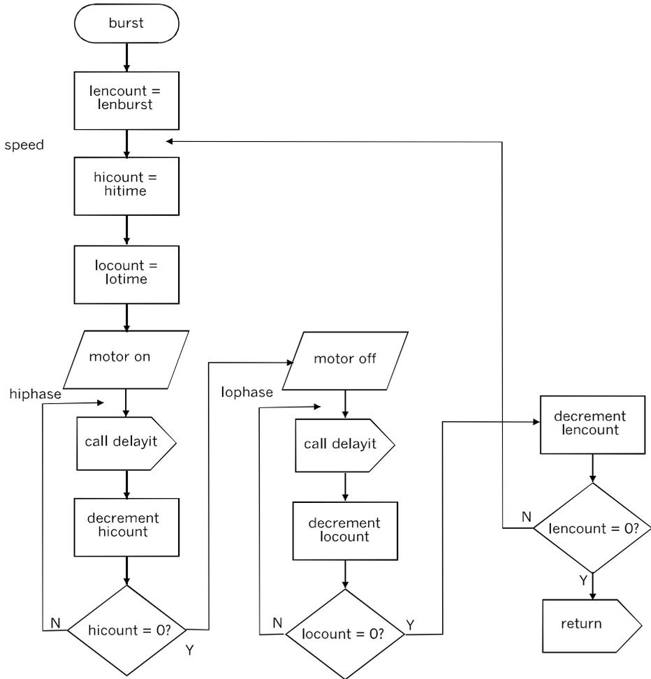
The *burst* subroutine produces a train of pulses of fixed frequency and length but with variable mark:space ratio.
