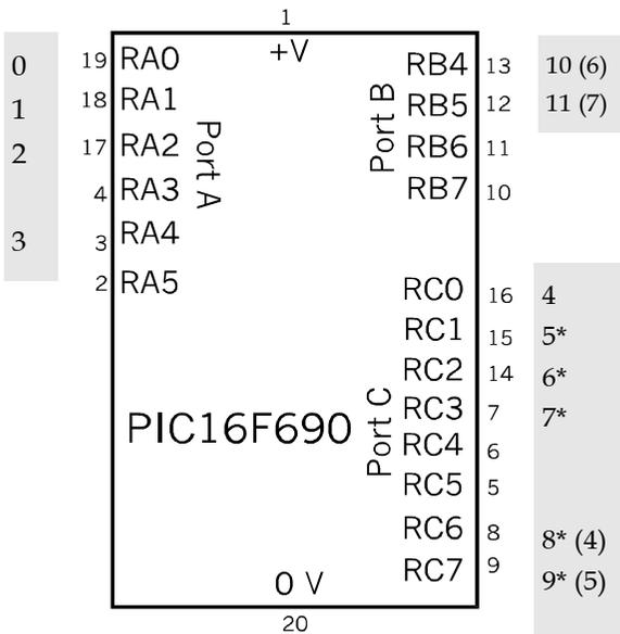
Ports and pin numbers of the PIC16F690 controller. The channels of each port are numbered from 0 to 7, from the least significant to the most significant bit. Port A has only six channels. Port B has channels for only the four most significant bits.
