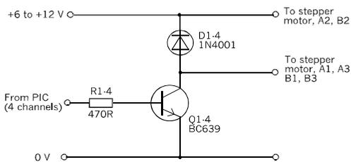
The circuit for driving the stepper motor. Four transistor switches like this are needed.
