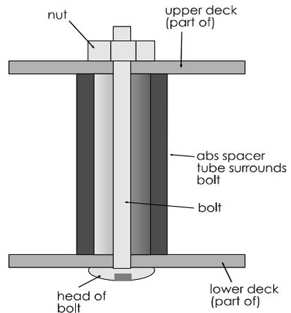
The decks are clamped together by three long bolts (one shown here). Each bolt is surrounded by a spacer tube cut from garden sprinkler tubing. The nut is tightened to hold the decks firmly against the ends of the tube.
