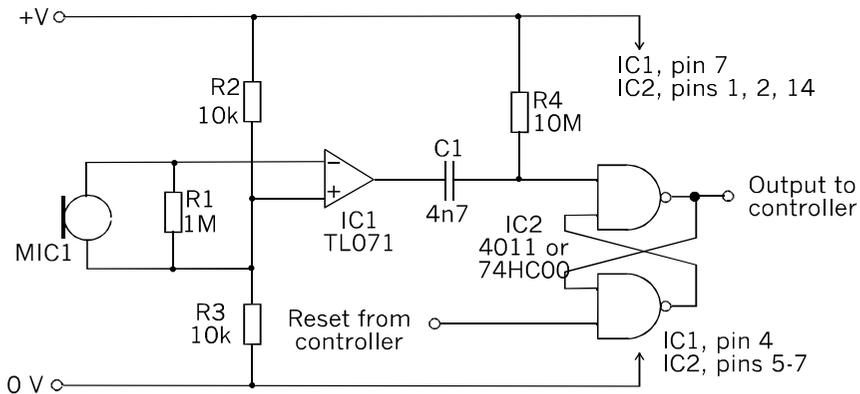
A crystal microphone generates a voltage spike that is amplified and used to trigger a flip-flop.
