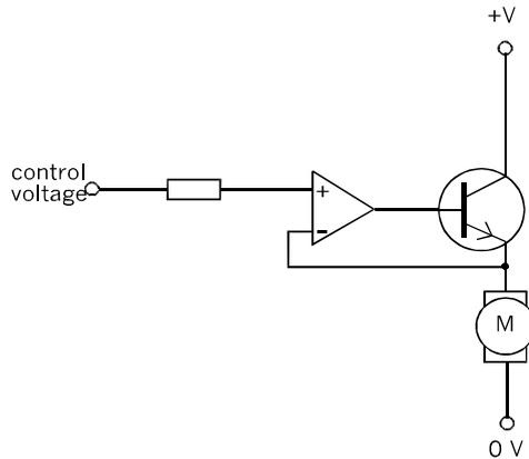
This circuit holds the speed of a motor steady even though the mechanical load on it changes.
