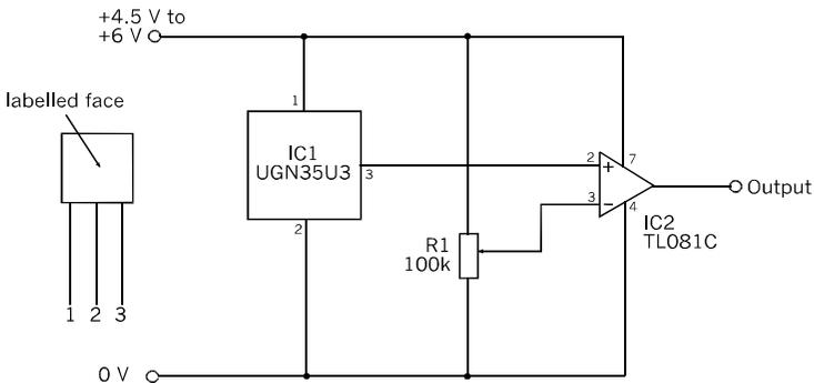
The output from the Hall effect device may be measured as a varying voltage or can be converted into a digital signal as in this circuit. The PIC's built-in comparator can be used instead of the op amp.
