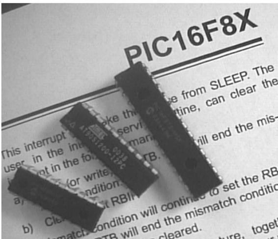
A selection of microcontrollers. From left to right, the 18-pin PIC16F84, from Microchip, the 20-pin Atmel AT90S1200, and the 28-pin PIC16F87.
