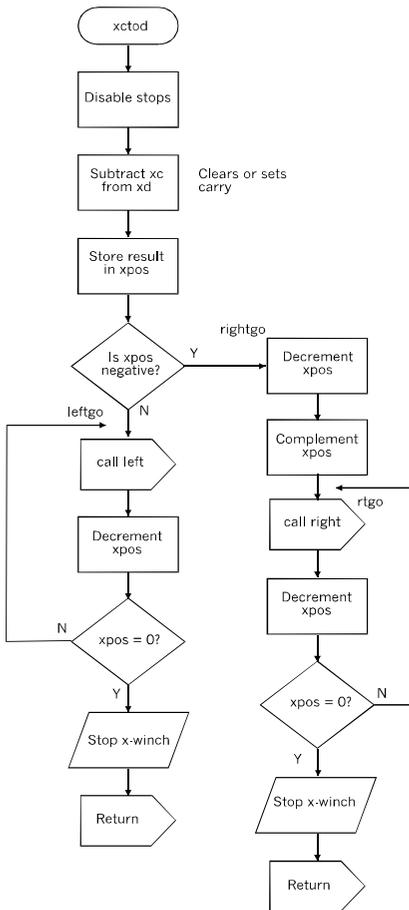
The *CtoD* routine works out the direction and distance between the current and destination locations, then moves the x-frame directly to its new location.
