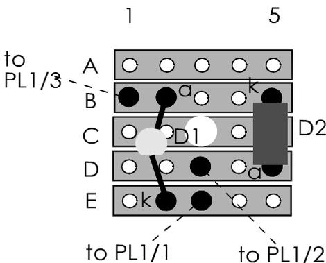
(Left) Stripboard layout of an IR probe. There is a central hole for the supporting bolt.
