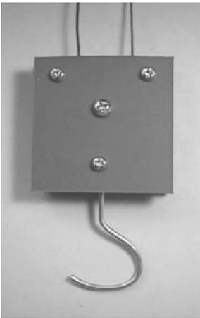
Two views of the hook, show it attached to a pulley block. The sides of the block are bolted together by two bolts at the top, with 6 mm spacers between them.
