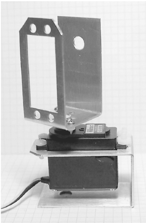
Figure 12.22 Assembled bottom brackets for robotic arm.
