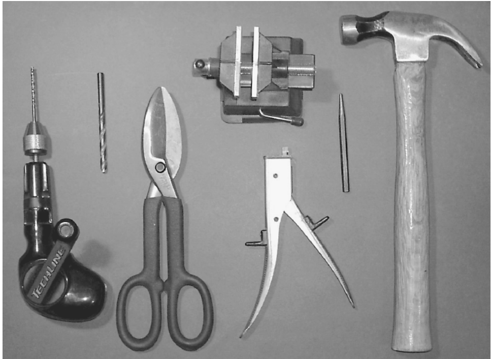
Figure 8.2 A few sheet metal tools.
