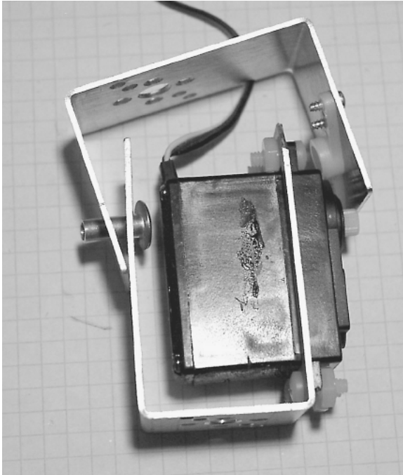
Figure 12.10 Bringing top bracket onto lower bracket to assemble.
