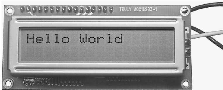
Figure 6.9 Photograph of LCD display “Hello World.”
