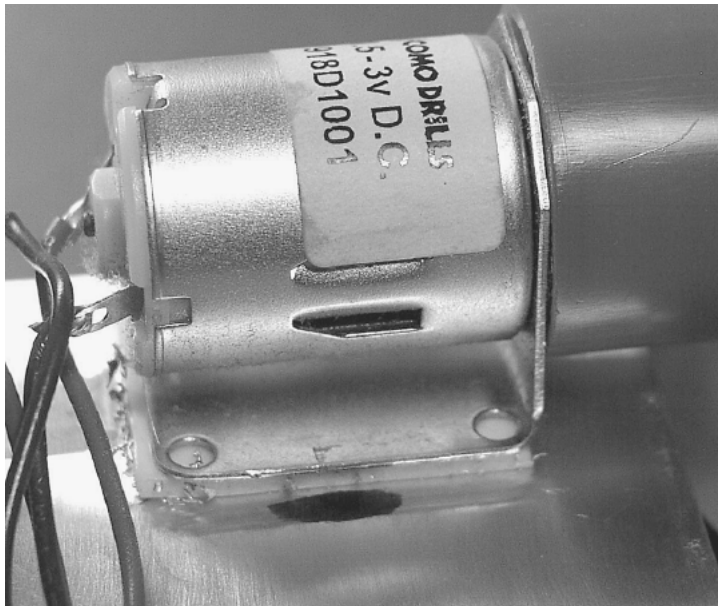
Figure 9.9 3M double-sided tape is used to secure gearbox motor to base of vehicle.
