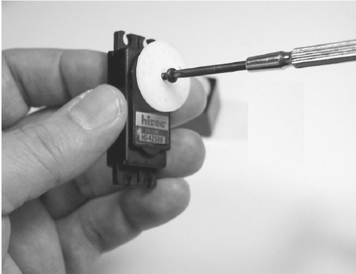
Figure 8.8 Removing servomotor horn from front of case.
