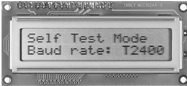
Figure 6.19 Photograph of LCD display in self-test mode.
