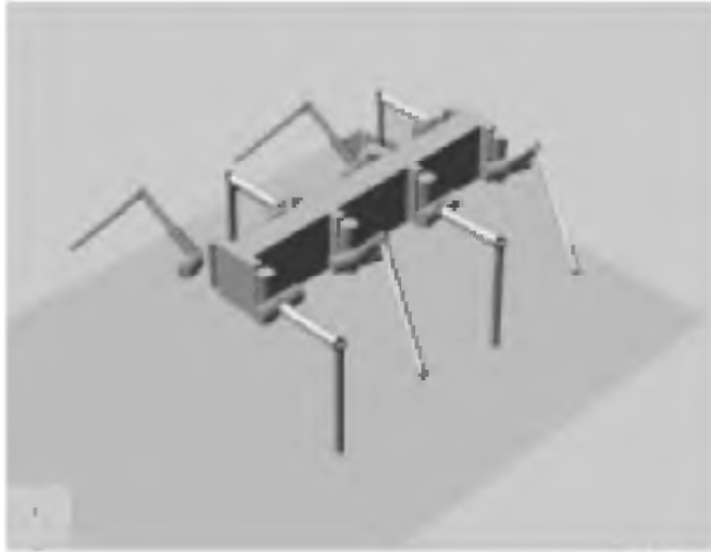
Figure 21.10 Due to the parametrical design approach it is possible to define two groups of legs in different starting positions each, thereby enabling the simulated Scorpion robot to initiate a walking maneuver.
