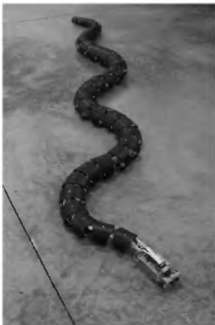
Figure 13.9 S5 seen from above. Two wavelengths of undulation fit within the length of the snake robot.
