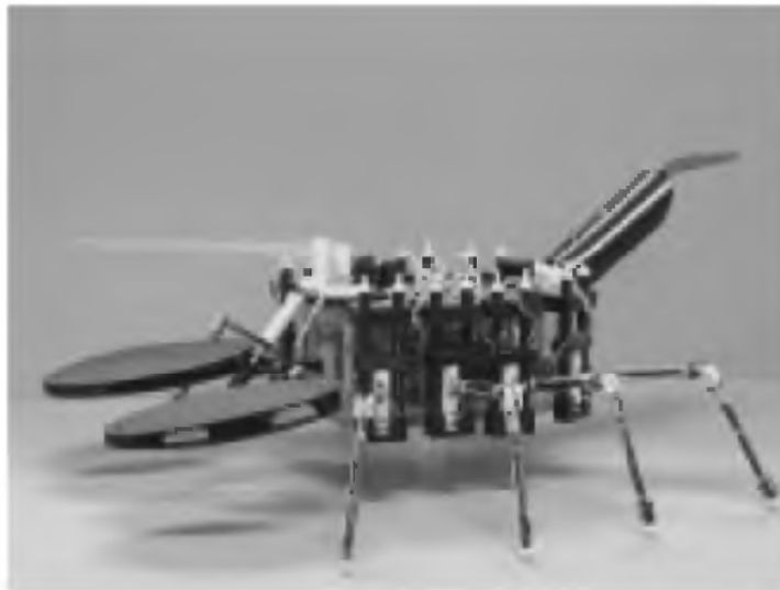
Figure 6.12 (a) schematic of the functioning of the leg assembly. L_m and L_d denote the equal length of the middle and distal leg segments. (b) a photograph of the assembled 8-legged ambulator.
