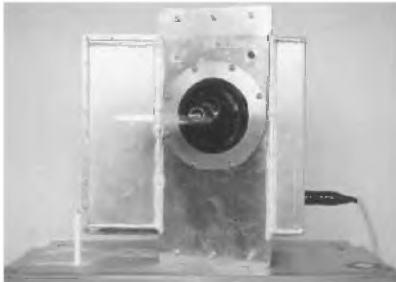
Figure 17.10 Three-motor-driven mechanical pectoral fin.
