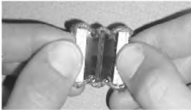
Figure 7.12 Acrylic film double bow-tie actuator.
