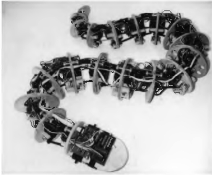
Figure 13.7 S3 seen from above. The tail and neck taper, and the universal joints form a spine along the length of the robot.
