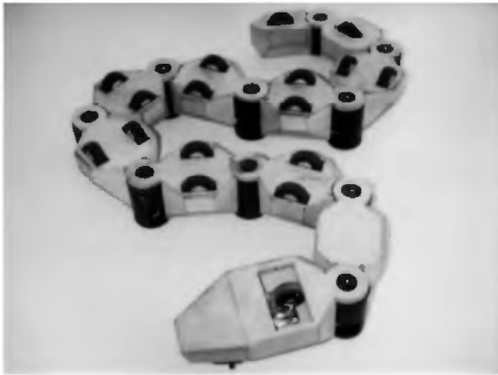
Figure 13.5 S2 seen from below. Note the caster wheel on the head and the lack of wheel on the next section back.
