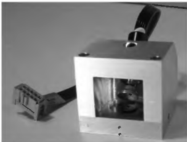
Figure 4.8 Photograph of a device producing circular scanning by spinning a tilted mirror. The device size is 38 mm × 38 mm × 38 mm.
