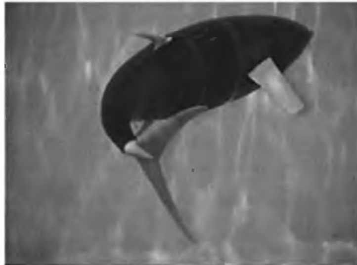
Figure 15.1 The Draper Laboratory VCUUV.
