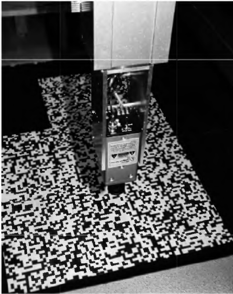
Figure 29.9 View of robotic gantry, showing camera head and visual texture on the floor.
