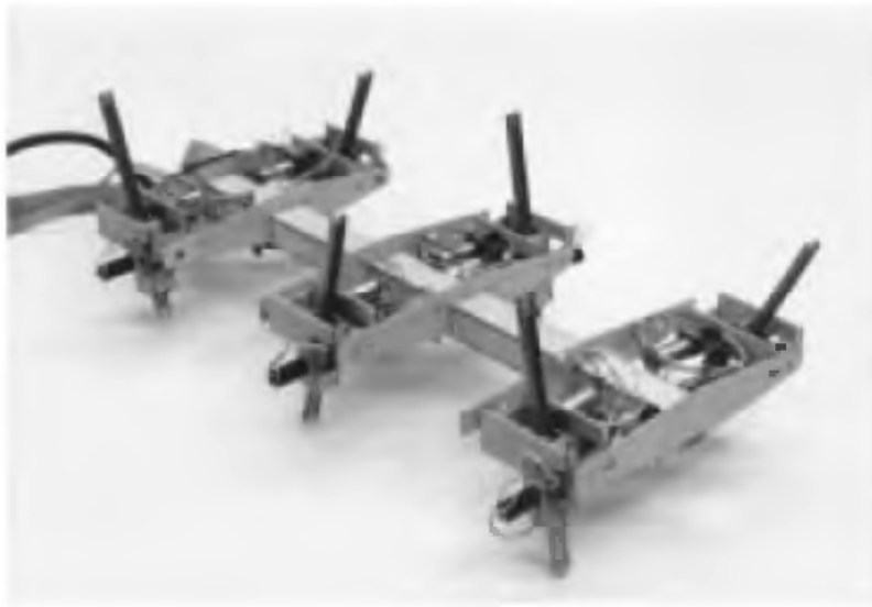
Figure 20.1 Robot I had legs with two degrees of freedom each: one rotational and one linear.
