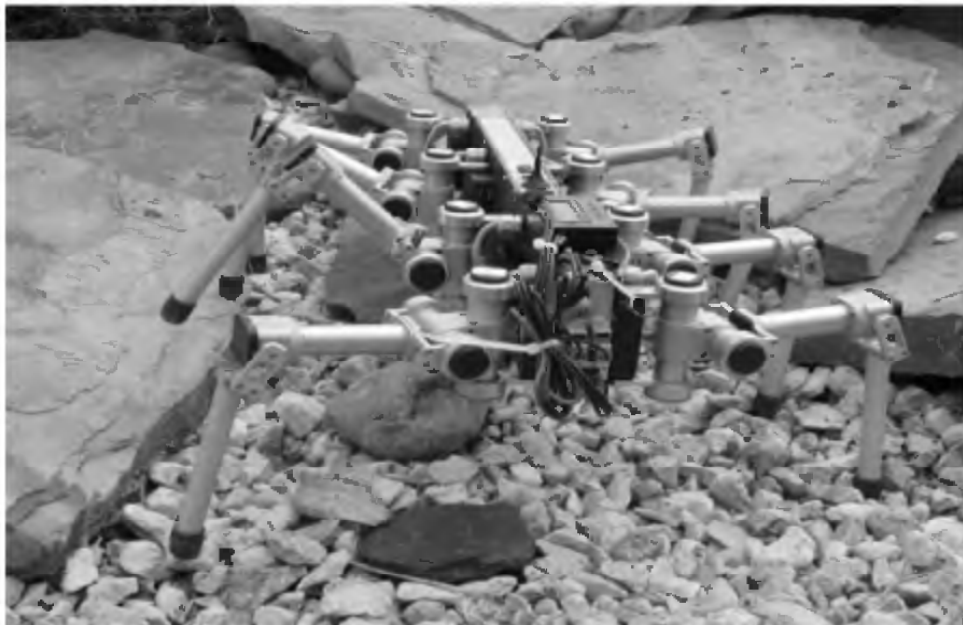
Figure 21.1 The first prototype of the Scorpion robot during an autonomous exploration into a rock channel. Note that obstacles have been up to three times as high as the robot itself. The obstacle course was 3 m wide and approx. 9 m long. The task was to complete the course within 20 min time.
