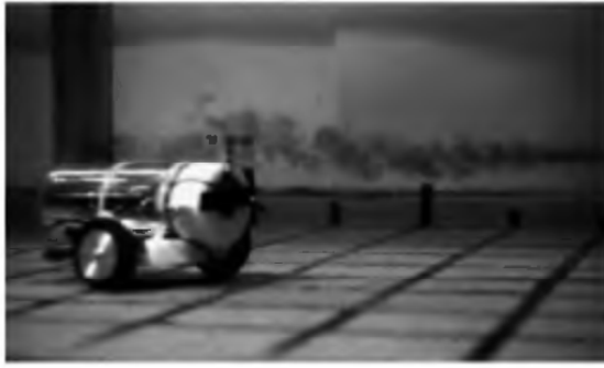
Figure 27.2 (Left) RoboLobster with a standard dye-tinted plume running a tropotaxis algorithm. The robot is inside a 10m \times 2m flume in seawater 44 cm in depth. The robot is designed to serve as a platform to carry chemical sensors, visible above the front end of the robot, through an odor plume. (Right) the BICSAAR Robot “Wilbur” in chemo-orientation trials in the same flume running one of the OGR algorithms.
