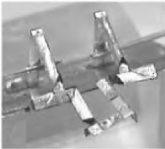
Figure 23.6 Flexural differential mechanism to provide both wing stroke and rotation by coupling two 4 bar structures.
