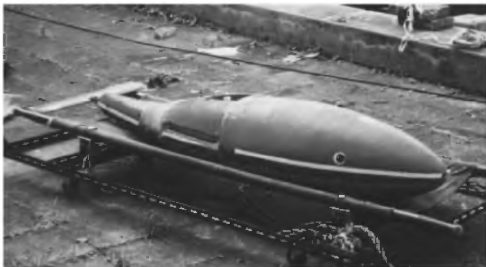
Figure 16.1 Photograph of the first two-joint dolphin robot.
