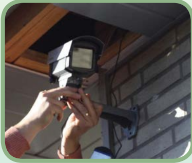
Christoph's smart surveillance project places a Raspberry Pi and Camera Module inside a fake CCTV camera housing
