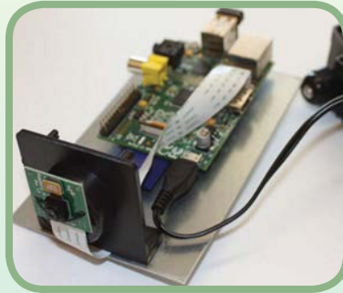
Christoph's smart surveillance project places a Raspberry Pi and Camera Module inside a fake CCTV camera housing
