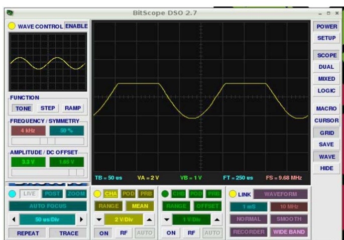
Fig. 9: Note the upper curve of the sine wave is clipped.
