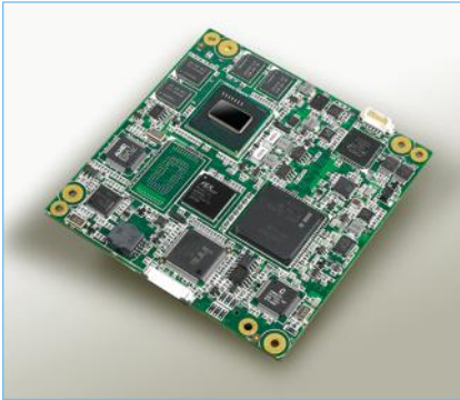
Figure 1 | The SOM-6764 COM Express 95 x 95 mm module from Advantech is based on the Intel Atom E6xx series processor.
