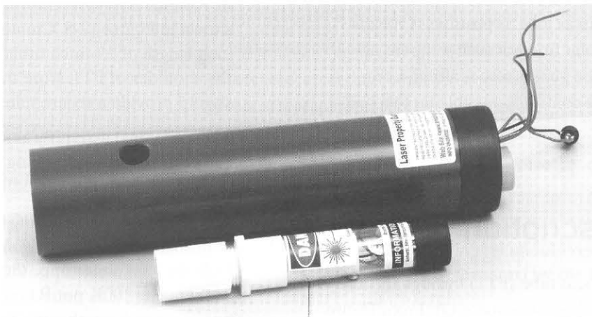
Figure 12-1 Property protection system
