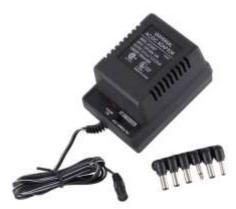
An External supply will consist of an AC to DC adapter. These come in various current and voltage ratings, and some even contain a variable regulator. You'll need to make a long cable to connect this to your robot, which can be cumbersome at times. You'll obviously need a regulator on board because different components run at different voltages.
