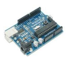
An Arduino is one of the simplest and most easy to use microcontrollers out there.
