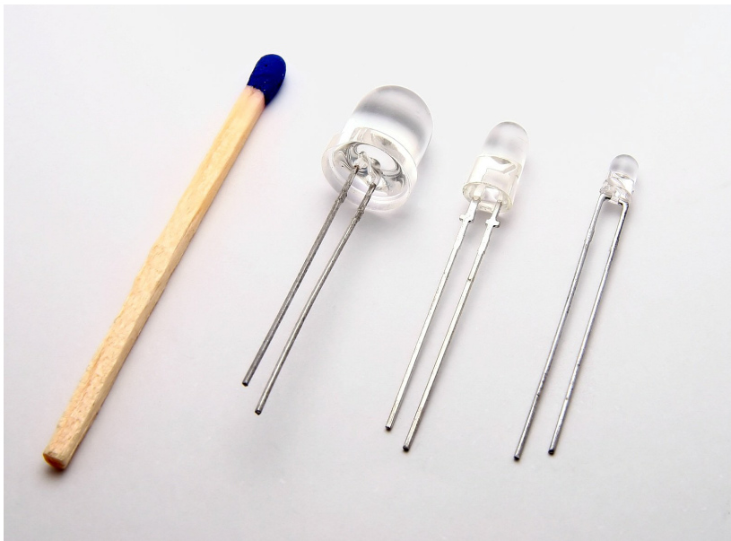
Figure 3-1. LEDs in 8 mm, 5 mm, and 3 mm sizes.
