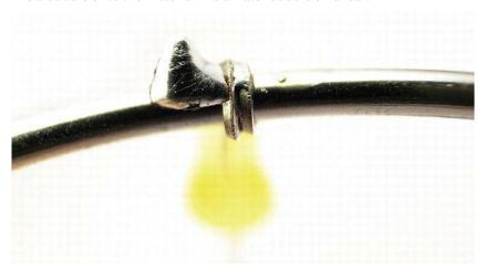
Figure 5-23. A cold soldering joint
