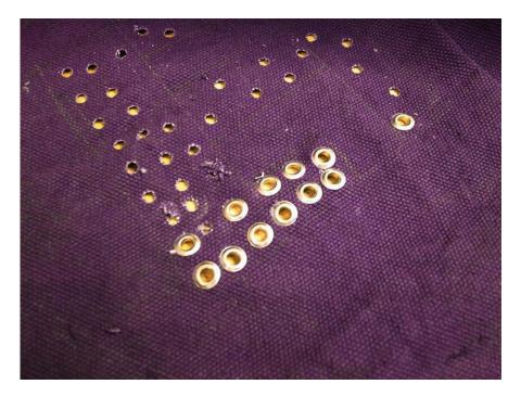
Figure 6-12. Eyelets punched in place
