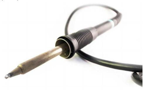
Figure 4-17. Soldering iron
