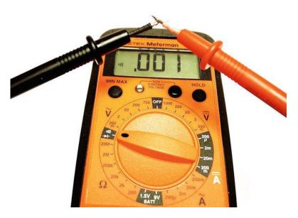
Figure 5-1. Finding conductivity with a multimeter
