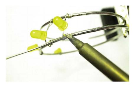
Figure 5-22. Soldering the LEDs
