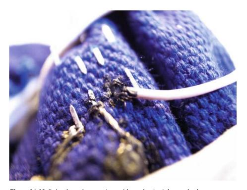
Figure 14-12. Paint the end connections with conductive ink to make them more secure.
