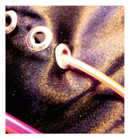
Figure 13-21. Pull the EL wires through the eyelets
