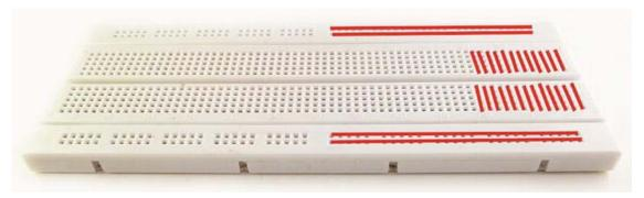
Figure 4-12. The connection of the breadboard
