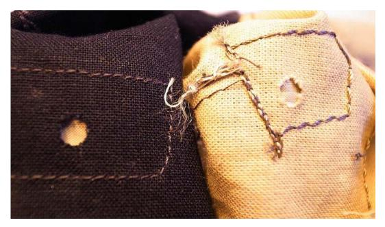
Figure 7-7. Conductive thread connections
