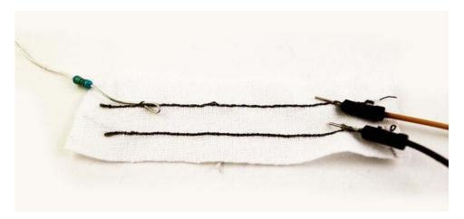
Figure 9-7. Making a test sensor
