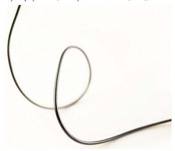
Figure 4-9. Smart wire that remembers shapes
