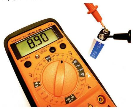
Figure 5-4. Measuring voltage
