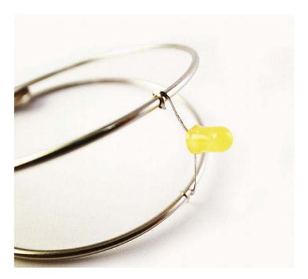
Figure 5-20. Wrapping the LED legs around the rings
