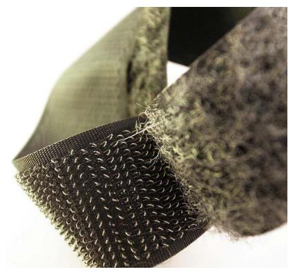
Figure 4-7. Conductive Velcro
