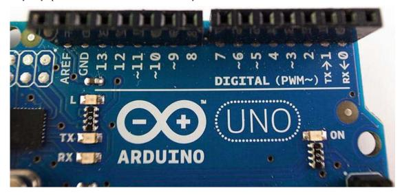
Figure 3-9. Digital pins from 0 to 13
