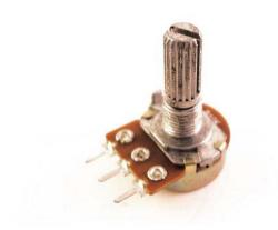
Figure 8-5. A standard potentiometer
