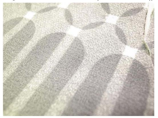
Figure 4-1. Thermochromic screen print on fabric
