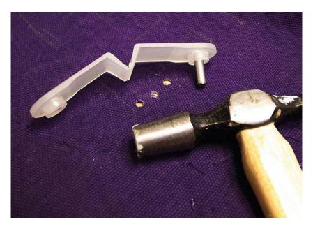
Figure 6-11. Punching holes for the eyelets
