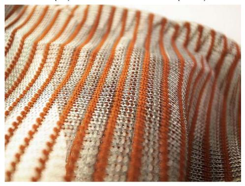
Figure 4-6. Conductive mesh fabric mixed with non-conductive thread
