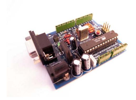
Figure 1-1. Early version of the Arduino serial board
