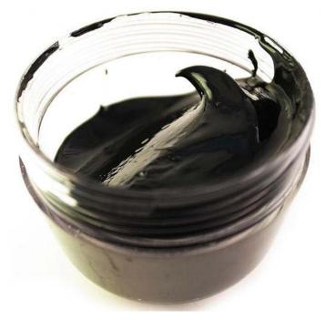
Figure 4-8. Conductive paint
