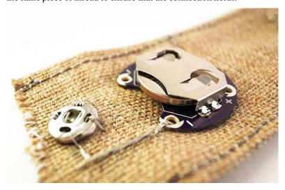
*Figure 5-15. Ground connection from the battery holder to the button*
