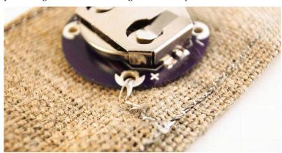
Figure 5-16. Making the power connection
