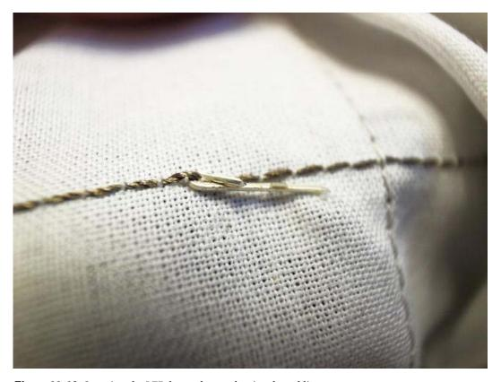
Figure 11-13. Securing the LED leg to the conductive thread line
