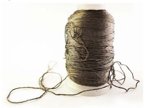
Figure 4-4. Roll of conductive thread
