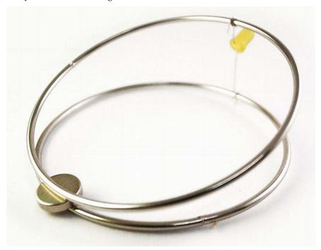
Figure 5-19. Magnet holding the rings together
