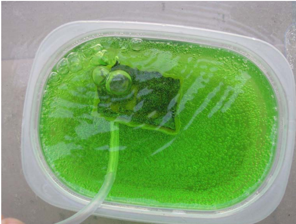
Figure 6-27. The etchant solution changes colors from clear to green as the copper dissolves.
