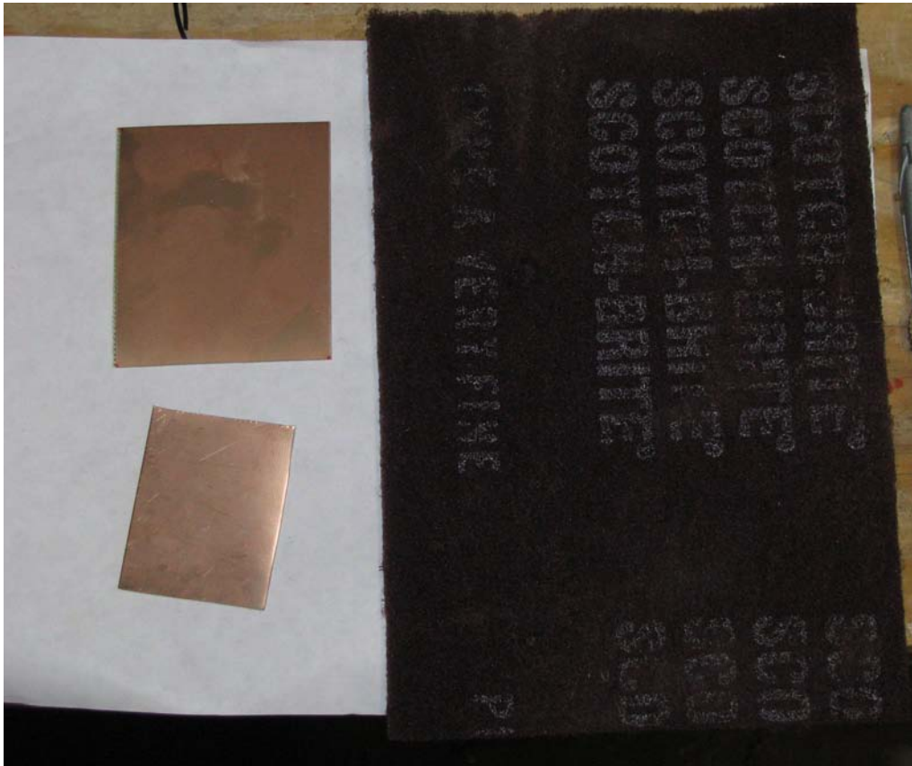
Figure 6-19. The two pieces of copper clad board cut to size and ready for cleaning
