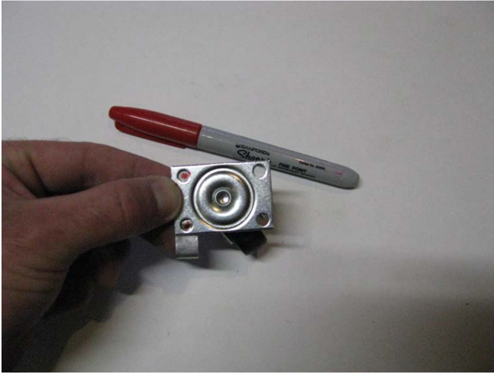
Figure 4-23. Bend the brackets so that there is enough room to swing the caster completely around. Then mark the mounting brackets, using the caster wheel-mounting holes with a permanent marker.
