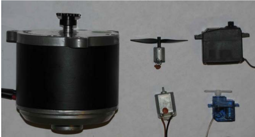
Figure 3-1. DC motors come in all shapes and sizes. The large motor is made for an electric scooter, the 2 in the center are small hobby motors, and the 2 on the right are DC servo motors.
