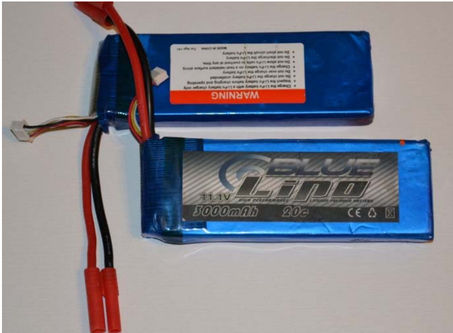
Figure 12-20. A blue Lipo, hobby grade 3-cell lithium polymer battery pack (11.1v)
