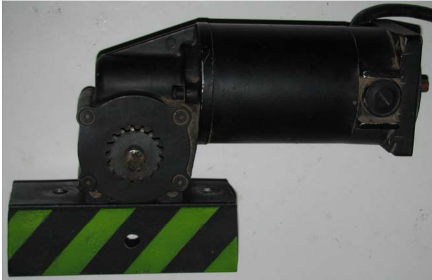
Figure 10-14. The motor secured to the motor mounting plate
