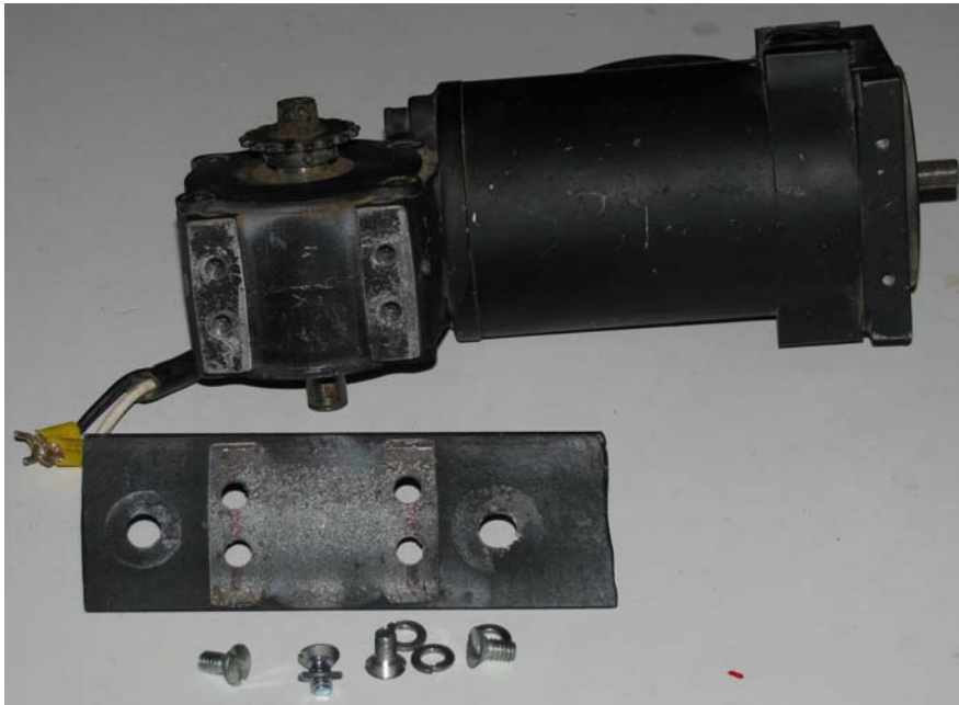
Figure 10-13. The motor mounting plate with 1/4-inch bolts
