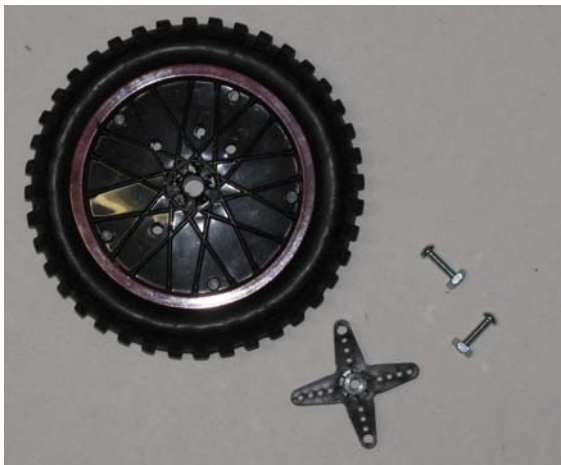
Figure 4-21. Some wheels from a thrift-store R/C car with the servo mounting bracket
