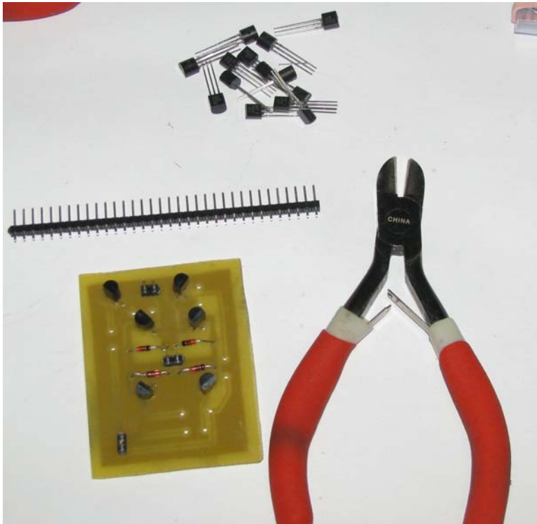
Figure 6-40. Snip three sets of two header pins from the strip with pliers, and solder one set for the power terminals, one set for the motor terminals, and the last set for the input connections.
