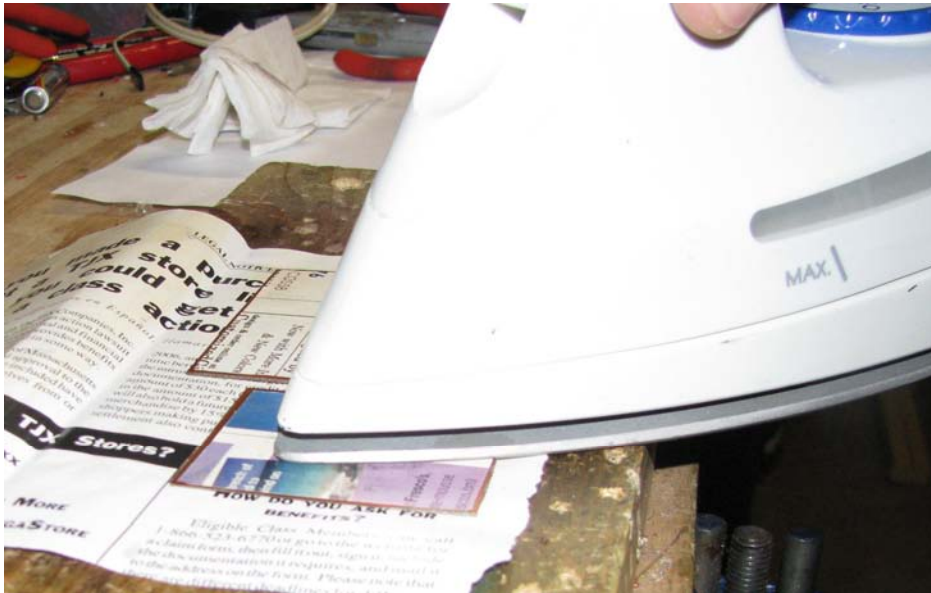
Figure 6-21. Heat each board with an iron (on the highest heat setting), placing an extra sheet of magazine paper between the iron and the back of the actual design.
