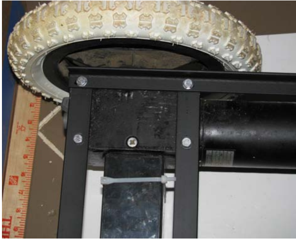
Figure 8-12. The main frame piece attached to the rear wheels using four bolts through the remaining mounting holes on each side.
