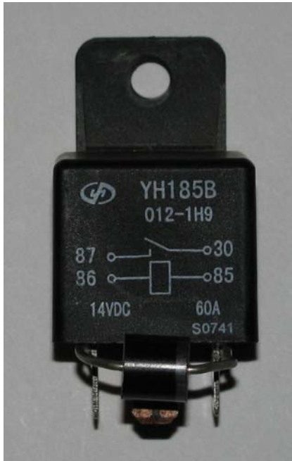
Figure 10-27. The Failsafe power relay used to switch the main power supply to the motor controller
