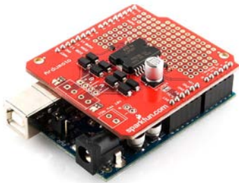
Figure 3-20. The Sparkfun Arduimoto is a motor-controller shield that is built around the L298N dual H-bridge IC.
