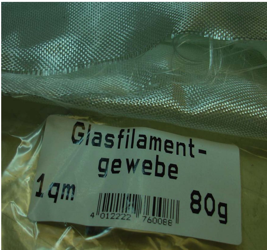
Figure 9-2. Woven fiberglass fabric with 80g/m 2
