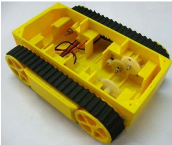
Figure 5-11. The DFRobot RP5 Mobile Tank Platform includes two drive motors with gearing, wheels, and tank tracks. You can easily mount your Arduino, batteries, motor-controller, and sensors to this frame.
