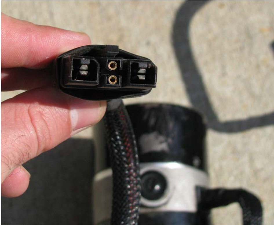
Figure 11-9. The wiring harness connector of a motor with an electric solenoid brake installed
