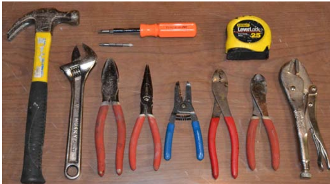
Figure 1-28. My basic tool kit: multi use 6-in-1 screwdriver (top-center), 25-foot tape-measure (top-right), (from left to right) hammer, crescent wrench, lines-man pliers, needle-nose pliers, wire strippers, wire-crimpers, wire-snippers, and vice-grip pliers.
