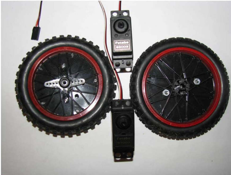
Figure 4-22. Both wheels with the servo brackets mounted and the motors next to them
