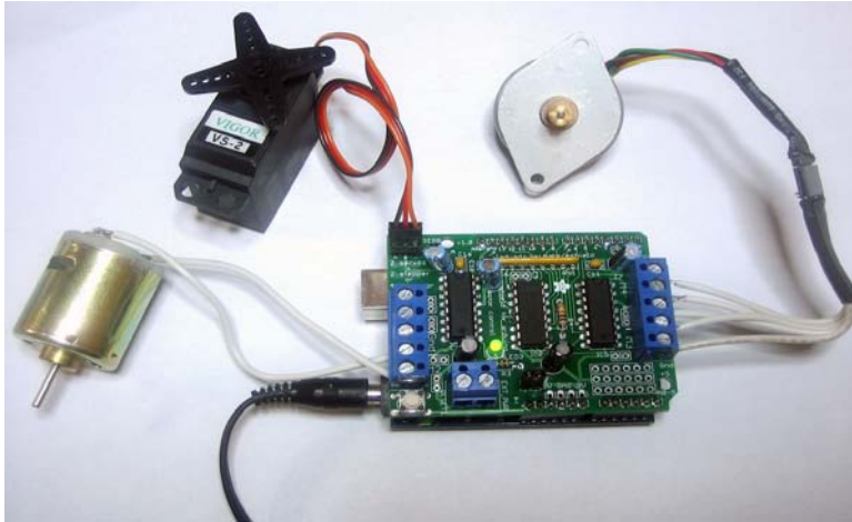
Figure 2-16. The Adafruit motor-shield is an easy-to-use motor-driver for the Arduino that can drive a variety of different motors, from left to right: DC motor, Servo motor, Stepper motor.
