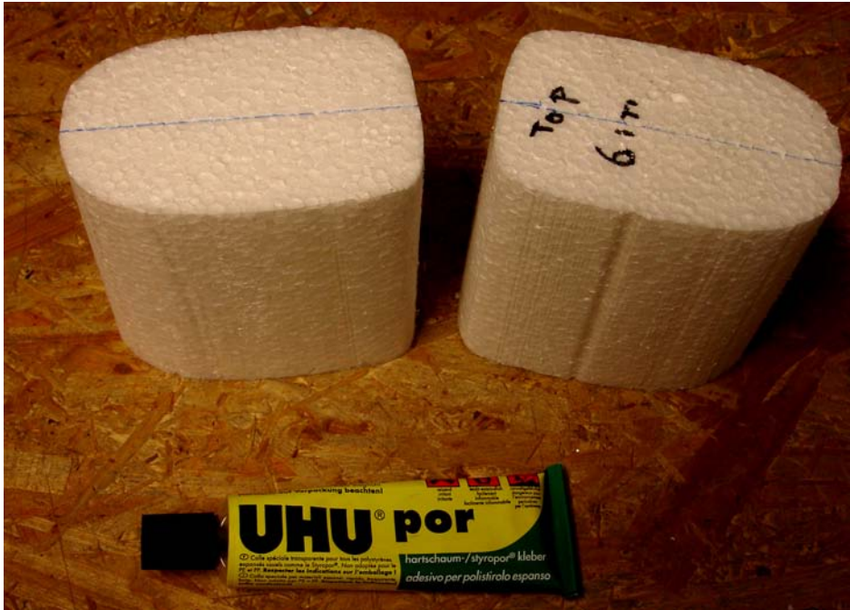
Figure 9-13. Two adjacent segments with EPS/XPS glue
