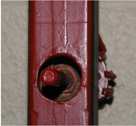
Figure 11-24. The Gain potentiometer mounted through the steel square tubing. If you look through the 5/8-inch hole, you can see the potentiometer mounting nut tightened down to the backside of the square tubing. Also visible behind the square tubing on the right side is the potentiometer base with three signal leads.
