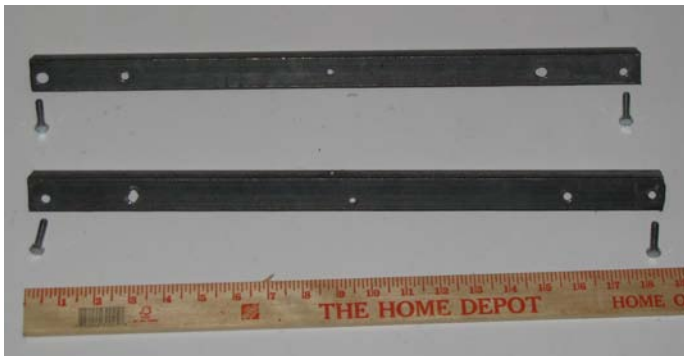
Figure 8-6. The two upper frame braces, used to hold secure the motors together on the top, which should be the same length as the bottom battery brace.
