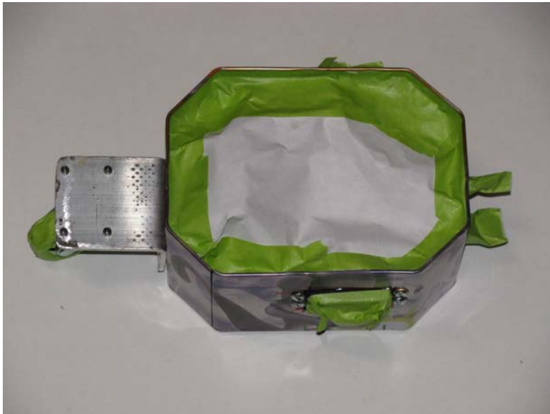
Figure 4-41. The bot is prepped with tape and ready for spraying.
