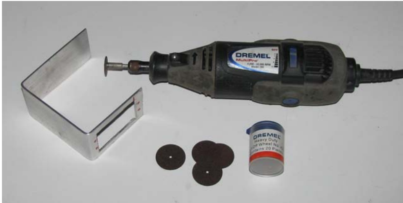
Figure 8-20. Cut a hole for the servo motor using a Dremel tool and metal cutoff wheel.
