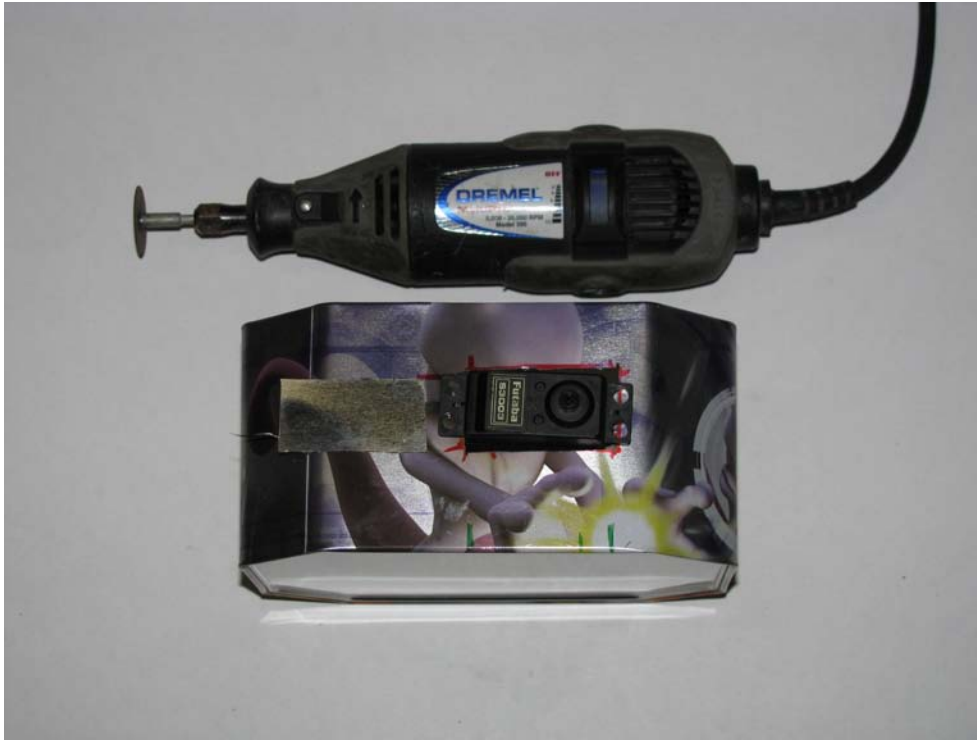
Figure 4-26. Using a Dremel rotary tool (or similar), cut holes the size of your motors.
