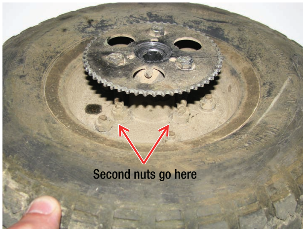
Figure 10-5. The rear wheel with sprocket installed
