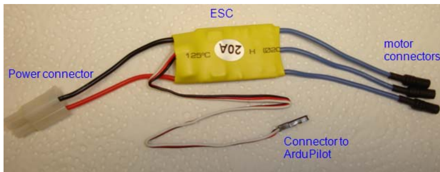
Figure 9-35. The electronic speed controller (ESC)
