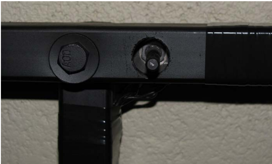
Figure 11-25. The steering potentiometer (without knob) mounted to the handlebar, just to the left of the handlebar grip
