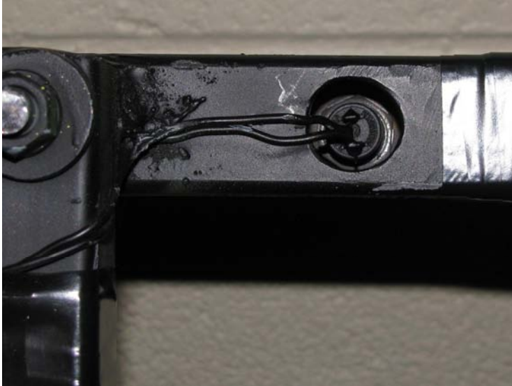
Figure 11-26. The backside of the Engage button switch, mounted into the square tube frame. There are two wires soldered to the rear terminals of the switch; one connects to GND and the other to Arduino D4.
