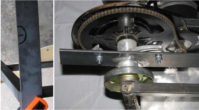
Figure 12-30. Modify the swinging arm to fit around the weapon axle (left, and the swinging-arm test fitted onto the weapon axle assembly (right).
