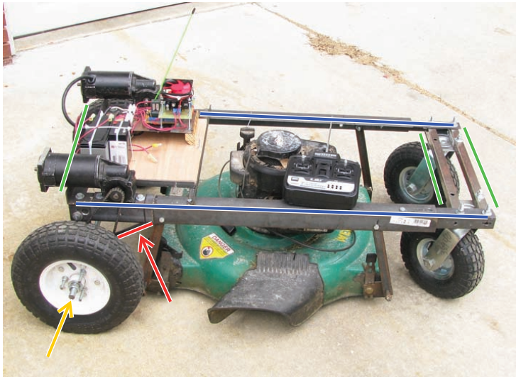
Figure 10-7. The axle and frame support bar
