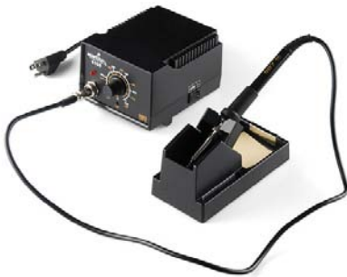
Figure 1-26. I had been using cheap soldering irons for years, and then my wife decided to buy me a “nice” soldering iron. The Hakko 936 is probably not the nicest available, but it is immeasurably better than the $7-$10 soldering irons that I had been wasting my time with before. It heats up in a matter of minutes and can get much hotter than a typical iron, making soldering a breeze.
