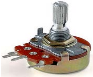
Figure 1-19. This typical turn-style potentiometer has three terminals. The outer two terminals should be connected to GND and +5v respectively (orientation does not matter), whereas the center terminal should connect to an analog Input pin on the Arduino.
