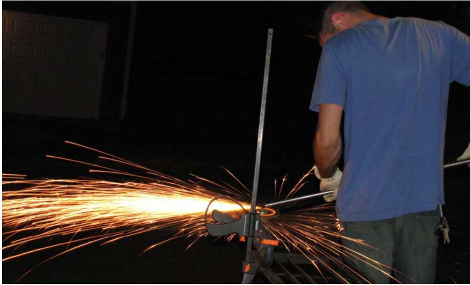
Figure 12-33. Grinding the spikes to make sharp points
