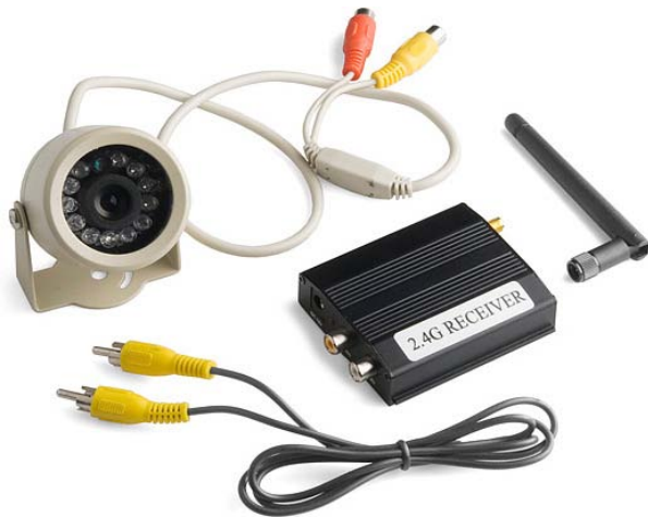
Figure 2-28. This 2.4GHz wireless camera from Sparkfun.com (part# WRL-09189) is an excellent way to add a remote set of eyes and ears to your robot for about $75.
