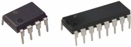
Figure 1-13. Here you can see an 8-pin Dual In-Line Package (DIP) IC (left), and a 16-pin DIP IC (right). The Arduino's Atmega168/328 is a 28-pin DIP IC (14 pins on each side).
