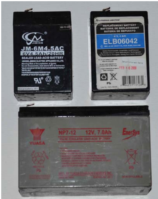
Figure 3-24. A few standard AGM sealed lead-acid batteries. Pictured are two 6v, 4.5AH batteries (top) and one 12v, 7AH battery (bottom).
