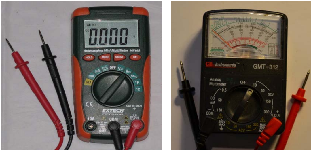
Figure 1-5. The Extech MN16a digital multi-meter (left) measures AC and DC voltages, resistance, continuity, diode test, capacitance, frequency, temperature, and up to 10 amps of current. An inexpensive analog multi-meter purchased at my local hardware store (right) measures DC and AC voltages, resistance (1k ohm), and up to 150mA (0.15A) of current. Either work to diagnose an Arduino and most other circuits—but you definitely need one.
