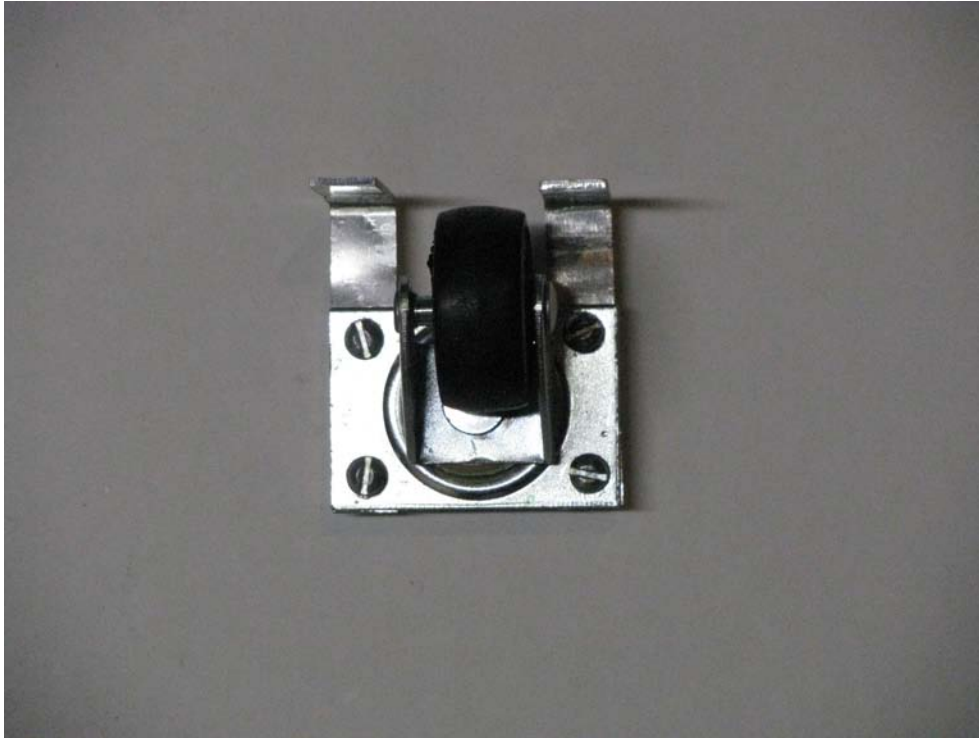
Figure 4-25. The castor wheel with all four bolts secured to the mounting bracket.
