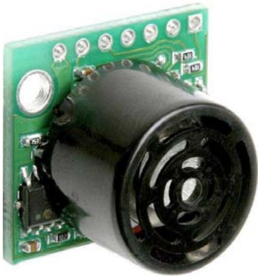
Figure 2-24. The MaxBotix LV-EZ0 ultrasonic range finder with an effective range of 6 inches to 25 feet (Sparkfun.com part# SEN-08502)
