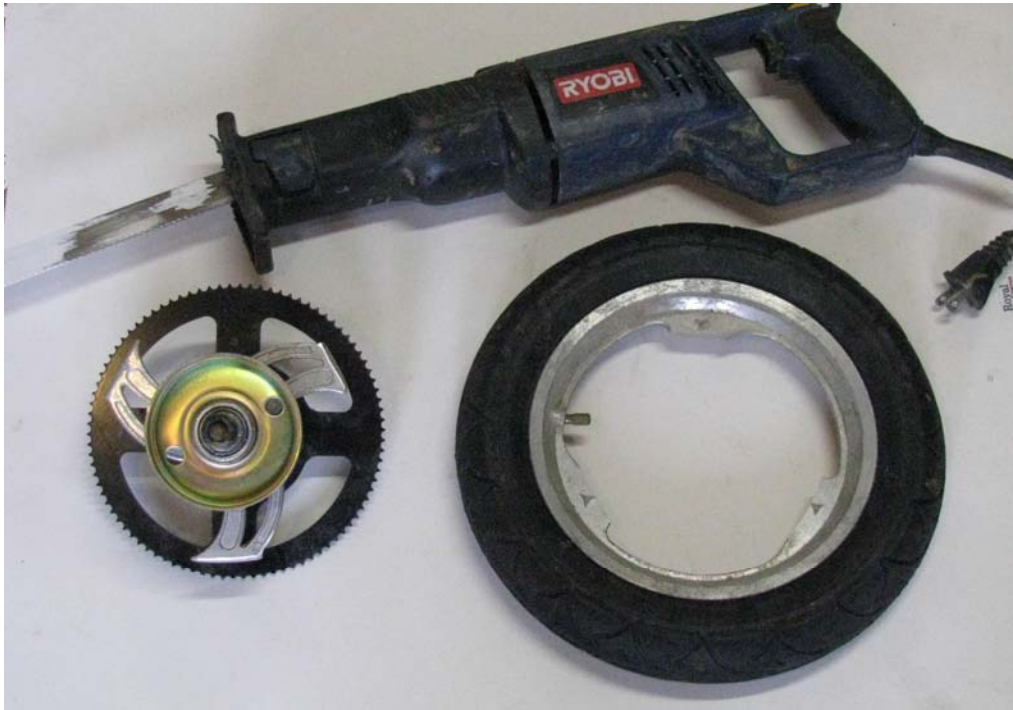
Figure 12-25. Cutting the wheel hub assembly from a rim to use as the weapon axle
