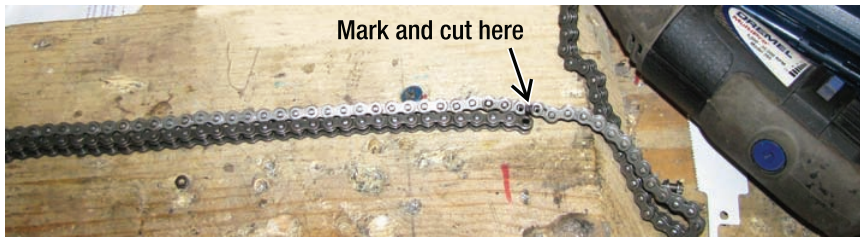
Figure 12-17. Measuring and cutting the chains
