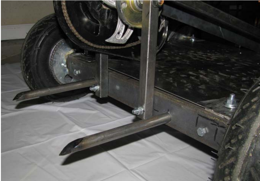
Figure 12-34. The spikes protruding from the frame, ready to impale an opponent
