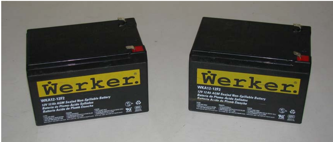
Figure 11-16. These two 12v 12AH Werker brand batteries provide plenty of run time for the Seg-bot.
