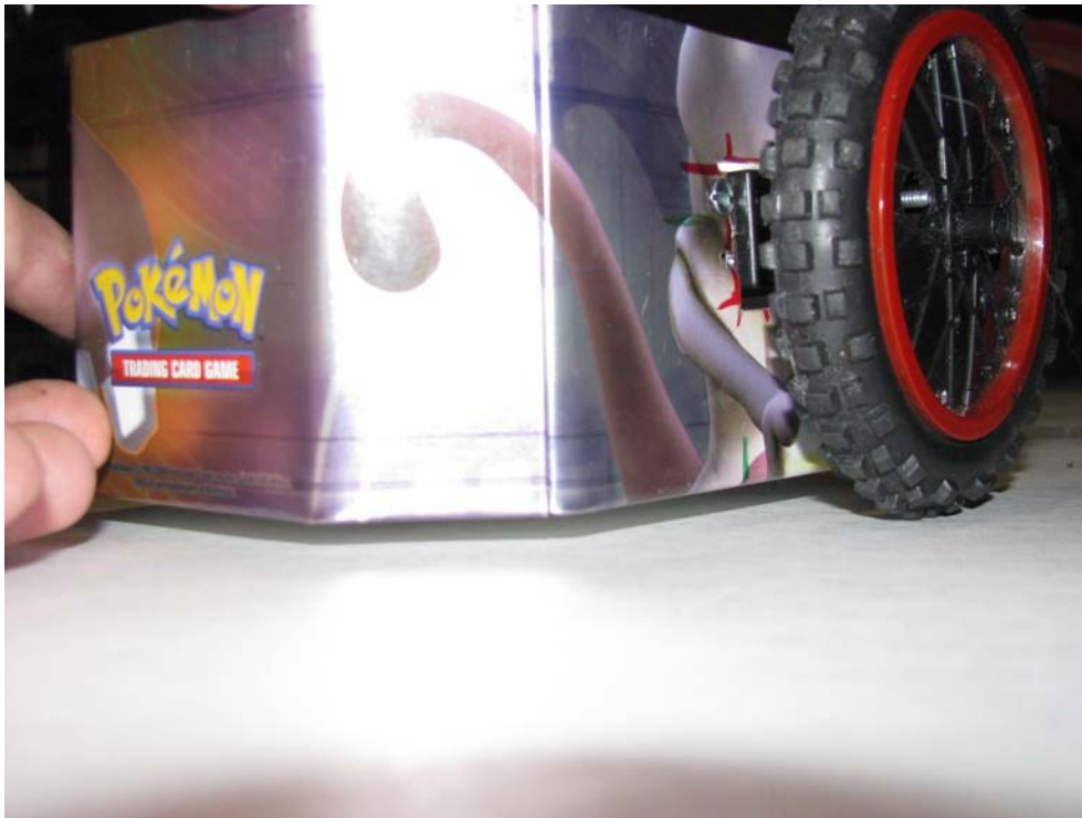
Figure 4-27. The wheel holes have been cut, the wheel test-fitted, and the rear ground-clearance looks good (about 0.25 inch to 0.5 inch).
