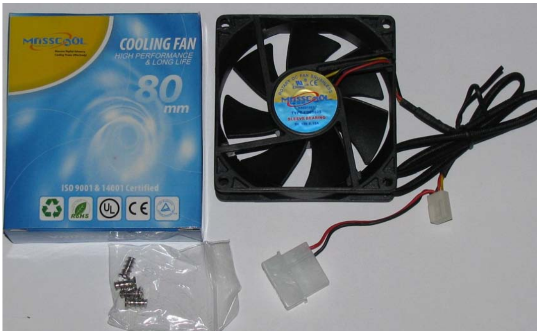
Figure 10-21. A standard 80mm PC cooling fan works perfectly to remove heat from a motor controller.
