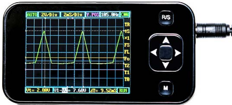
Figure 1-8. The DSO Nano from SeeedStudio.com (and sold through Sparkfun.com) is an excellent choice for an inexpensive ($89), but full-featured, digital pocket oscilloscope.
