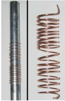
Figure 7-19. This image shows the wire wrapped around a 3/4-inch rod to give it a coiled shape (left), and when removed it retains the coils (right).
