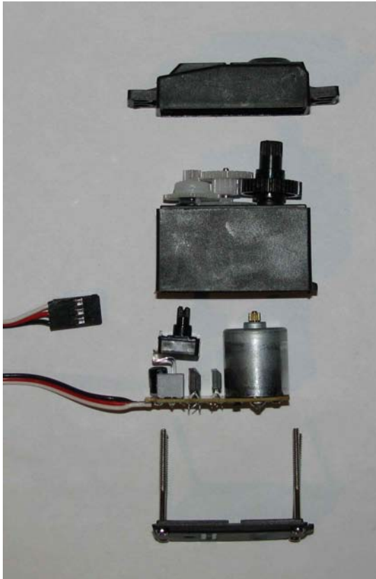
Figure 3-6. A dismantled view of the larger Servo motor from Figure 3-1 reveals the gears, potentiometer, circuit board, and DC motor that are normally packed inside the plastic casing.
