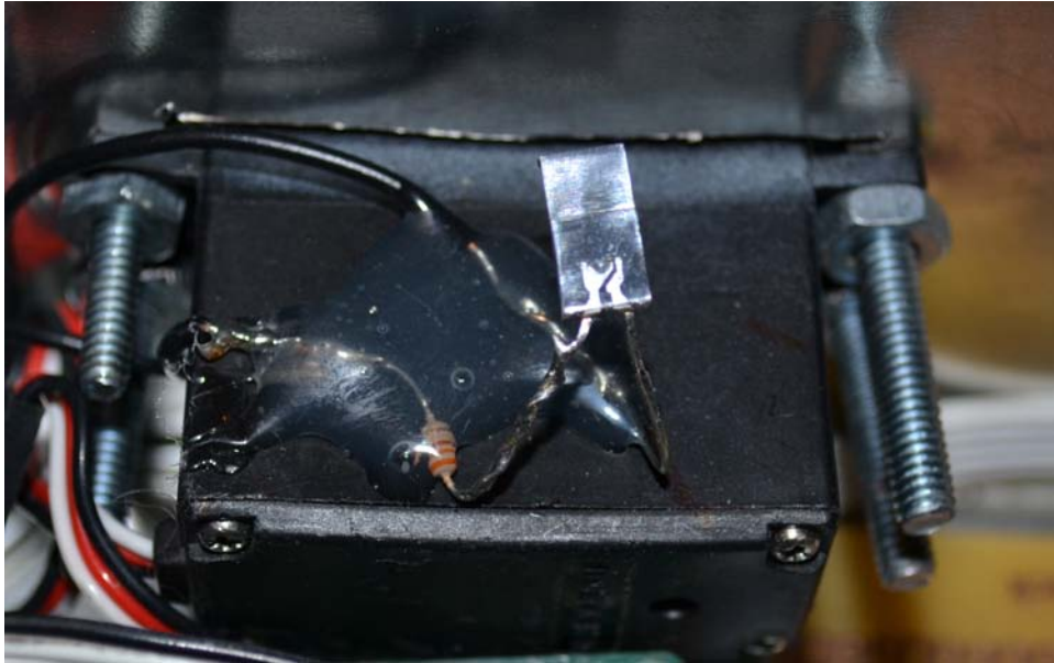
Figure 4-37. LED with resistor hot-glued to the top of the servo motor casing
