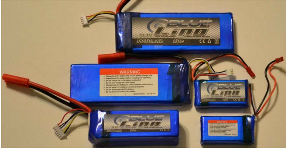
Figure 3-23. A few different sizes of hobby LiPo battery packs that I use for robotics projects. Shown are two 7.4v packs (2-cell), two 11.1v packs (3-cell), and one 18.5v pack (5-cell).
