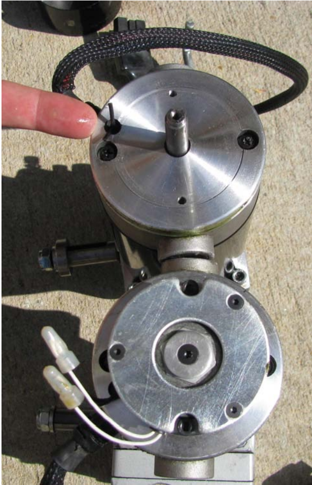
Figure 11-11. The two motors with dust caps removed—the brake has been removed from the upper motor, while still in place on the lower motor.
