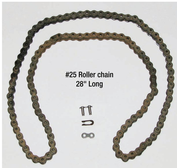
Figure 10-17. Each drive chain should be approximately 28-inches long and requires a master link to connect each cut end.
