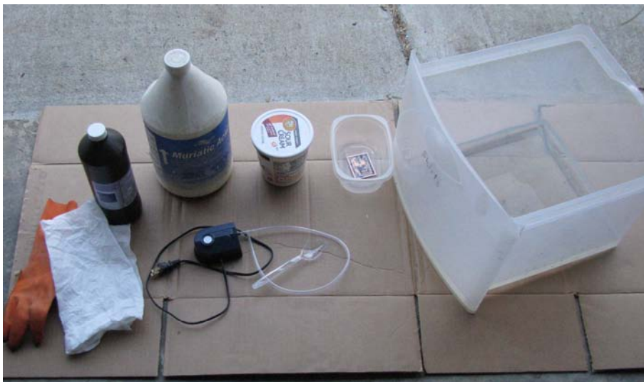
Figure 6-25. The chemicals and materials needed to etch a PCB at home. The two smaller containers will be used for different etching methods.
