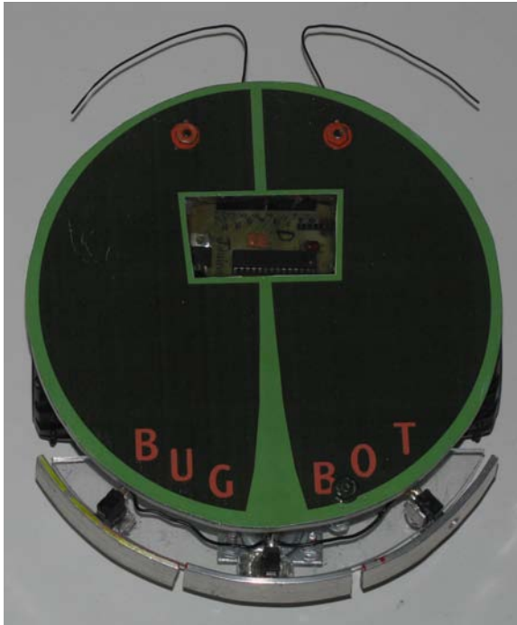
Figure 7-27. The finished Bug-bot with antennae contact sensors, rear bump sensors, and decorative top hat to give the robot a bug-themed exterior.
