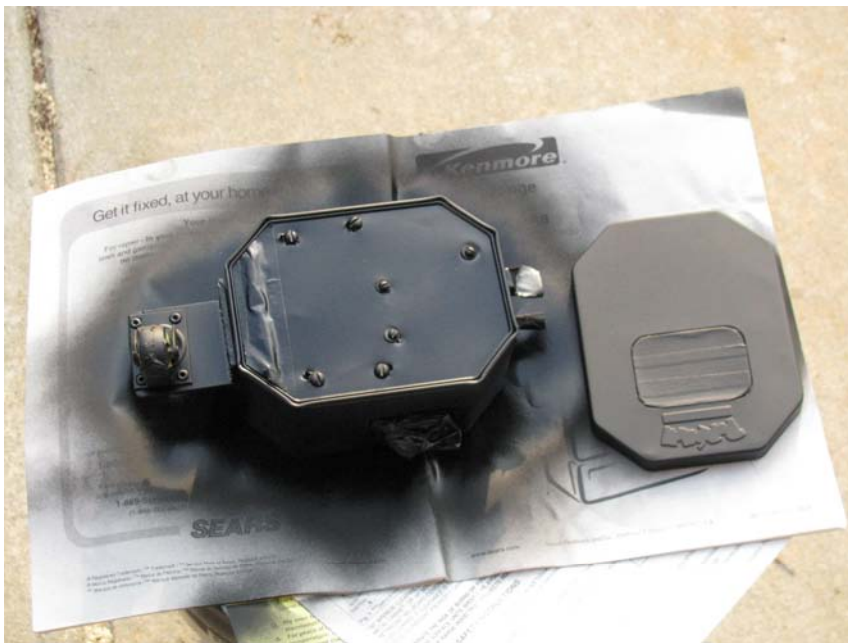
Figure 4-42. The first coat of flat black paint, after the gray primer
