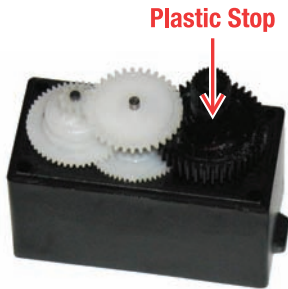
Figure 4-18. Using a soldering iron, melt away the plastic stop from the main black gear. It protrudes from the rest of the gear and keeps it from spinning continuously.
