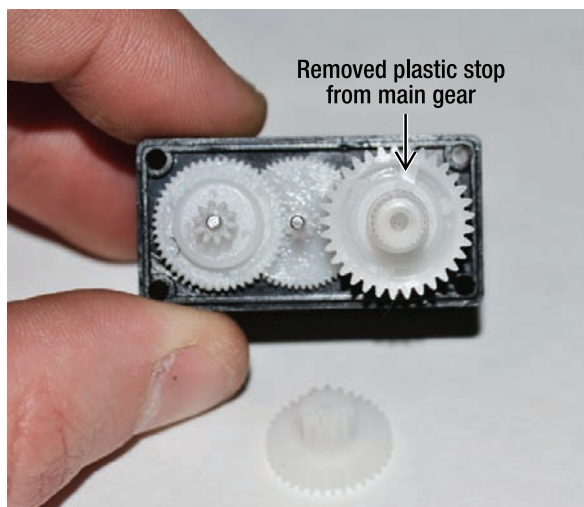
Figure 7-5. The plastic stop removed from the largest plastic gear (which is also the gear box output shaft)
