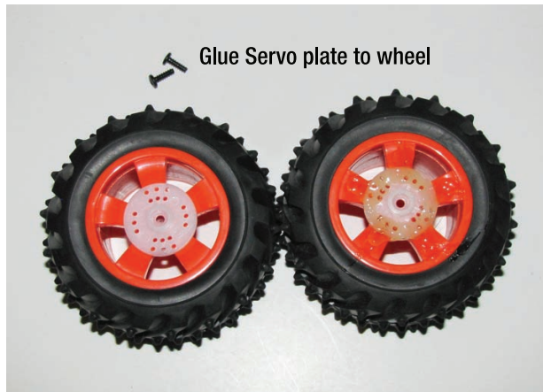
Figure 7-8. Center the Servo wheel adapter plates on each wheel before gluing them. You can use Super Glue or high strength hot glue.
