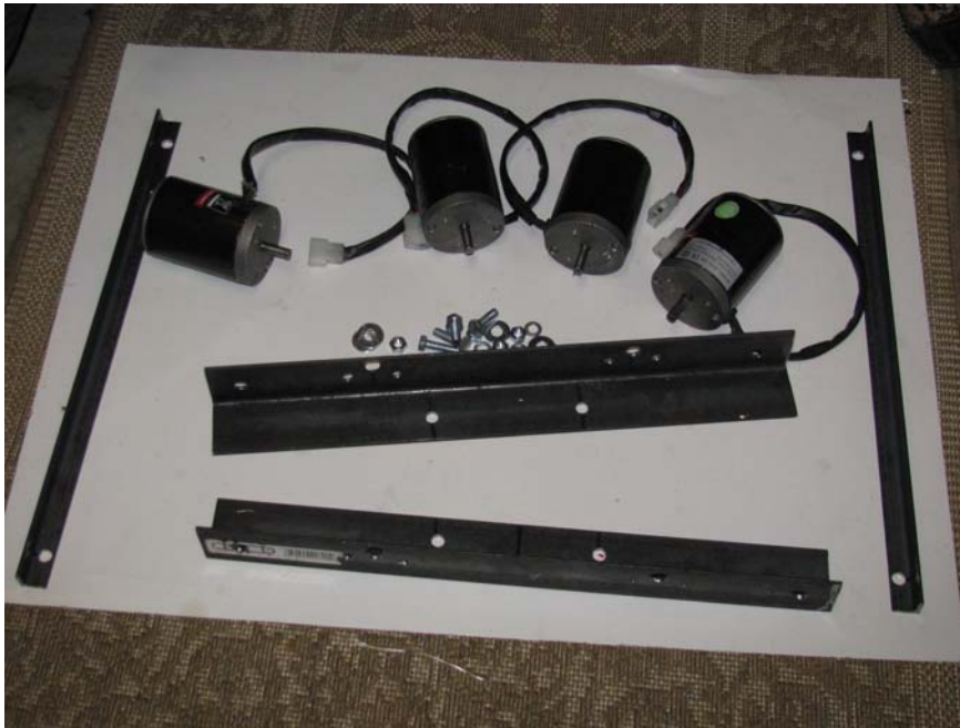
Figure 12-11. The side and center pieces of the sub frame with motors, ready for assembly
