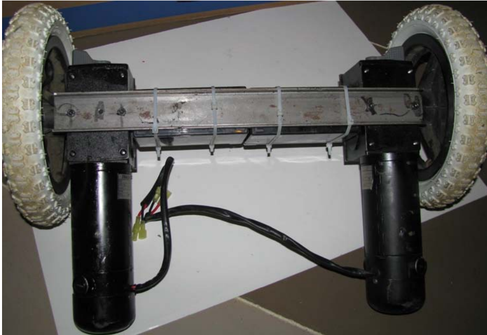
Figure 8-4. The battery brace attached to the bottom of the motor gear boxes, using two bolts to secure the brace to each motor
