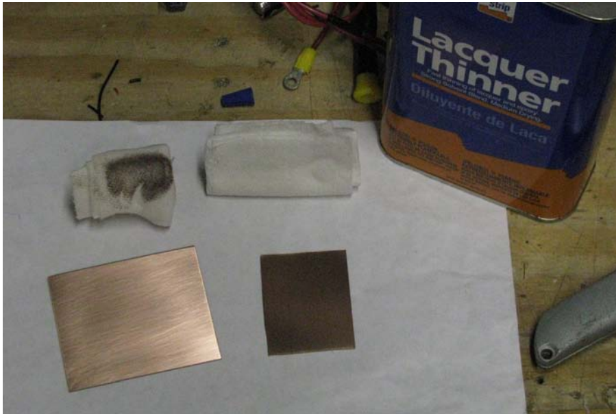
Figure 6-20. Both boards after scrubbing with the Scotch-brite pad and cleaning thoroughly with lacquer thinner (acetone works, too)
