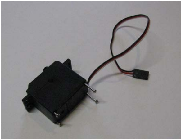
Figure 4-16. Remove servo motors rear screws and cover using a small Phillips head screwdriver.
