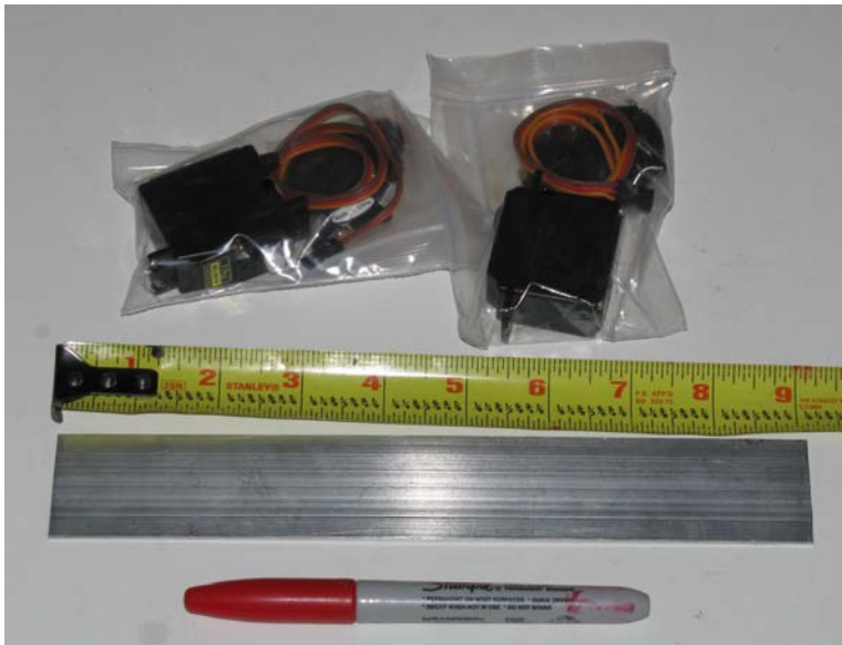
Figure 8-19. The pan/tilt mechanism is made from a few pieces of aluminum, some nuts and bolts, and two hobby servo motors.
