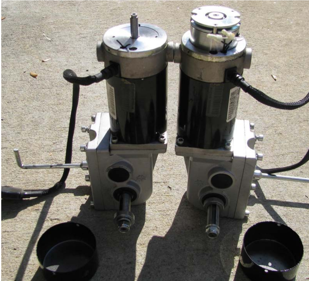
Figure 11-12. The two motors standing next to each other, the brake has been removed from the left motor, while still in place on the right motor. The dust caps are on the ground next to the motors.
