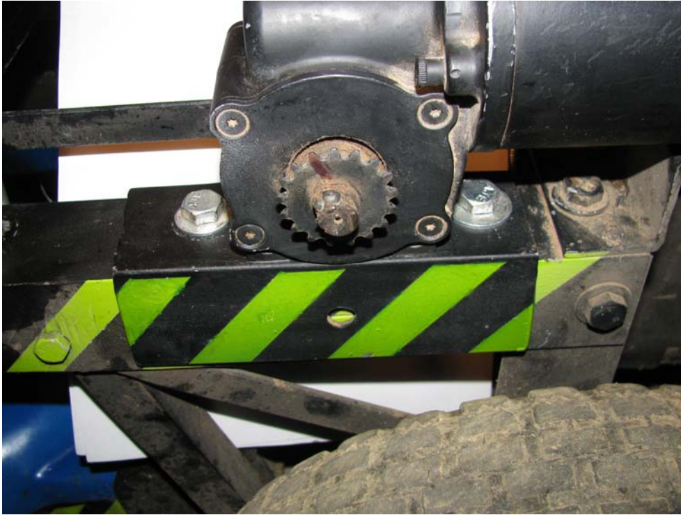
Figure 10-16. The motor mount secured to the main frame rail using two bolts
