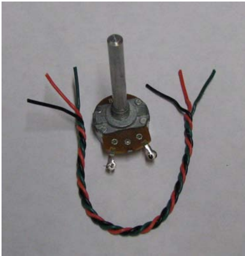
Figure 4-45. A potentiometer and three strands of solid copper wire to use for the speed control
