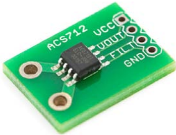
Figure 2-29. The ACS-712 bi-directional current sensor can be used in series with one of the load terminals to measure the amperage level. It can easily be read using an Analog input on the Arduino.
