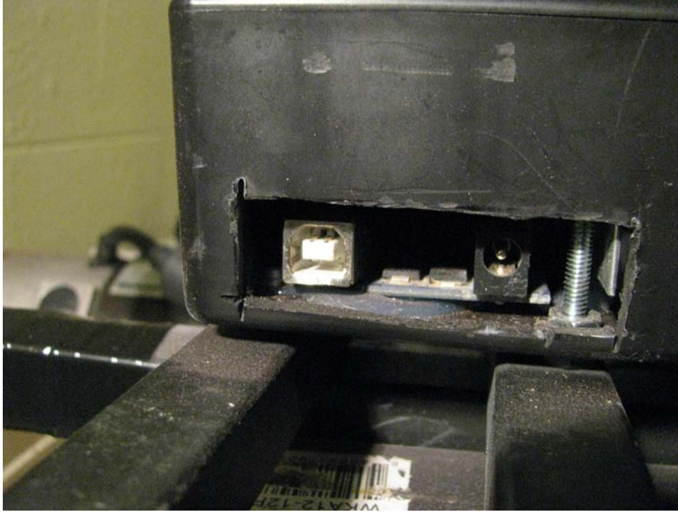
Figure 11-29. A rough cut into the project box with the Dremel tool enables easy access to reprogram the Arduino during testing.
