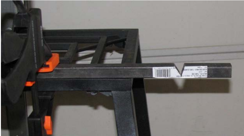
Figure 12-26. Cutting V notches in the weapon brackets
