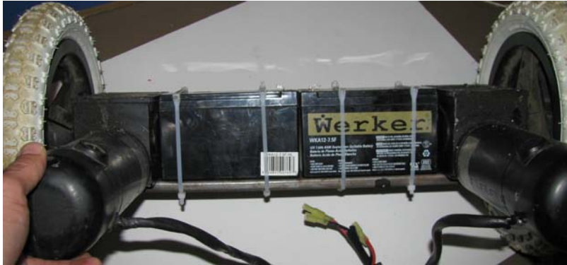
Figure 8-5. The two drive motors connected together by the battery brace
