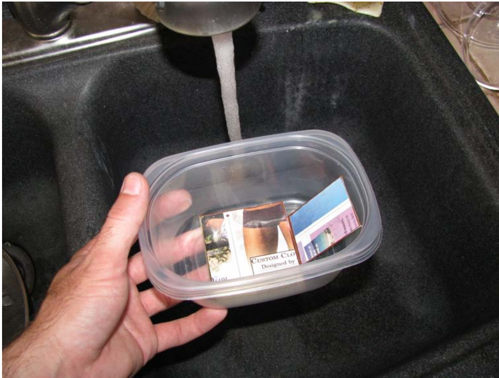
Figure 6-22. Place the cooled boards into a plastic container and add warm water with some soap to dissolve the magazine paper.
