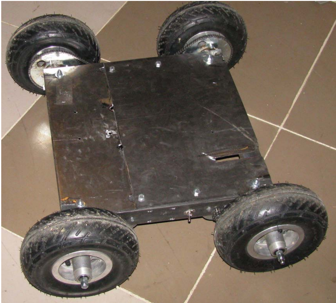
Figure 12-24. The basic frame fully assembled with armor
