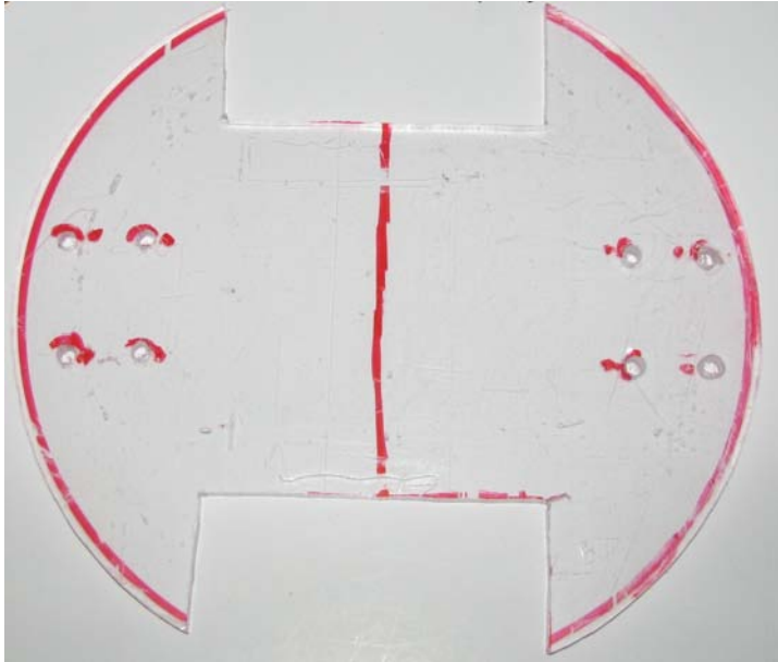
Figure 7-12. After cutting with a jigsaw (fine-tooth blade) and drilling holes for the caster wheels, the frame base plate is ready to mount the motors and wheels.
