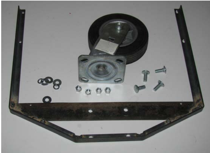
Figure 8-10. The main frame piece ready to be mounted to the motors and wheels
