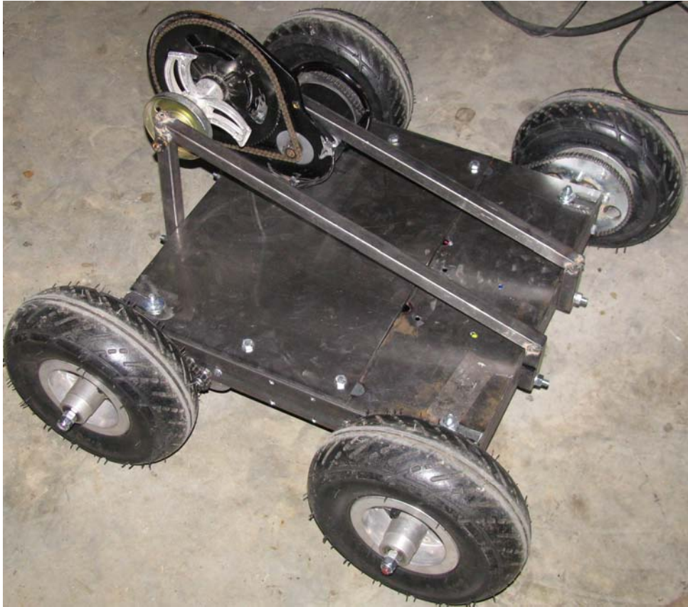
Figure 12.29. The finished frame with weapon axle and motor installed
