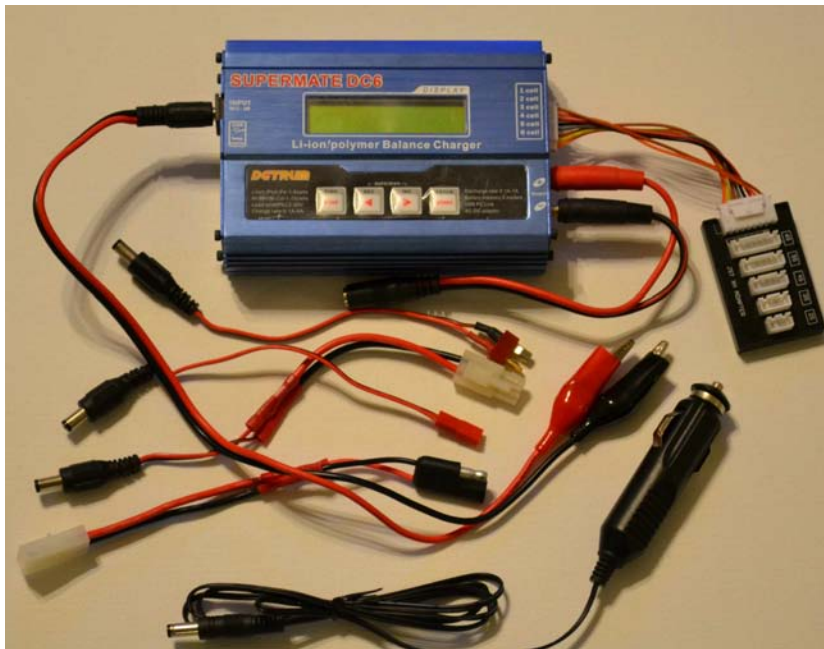
Figure 3-25. A Dynam DC6 multi-battery charger. This charger is compatible with LiPo, NiMh, NiCd, and Lead-acid—as well as having an adjustable charging rate.
